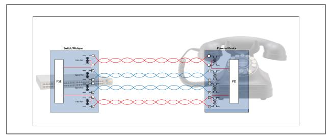
FIGURE 1: DATA DELIVERY OVER TWO PAIRS
