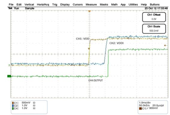
Figure 1 • I/O State When VDD is Powered Before VDDI
