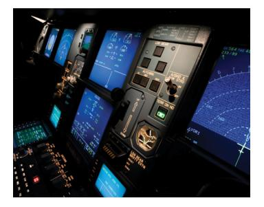
With the introduction of the Fly-By-Wire (FBW) electronic flight control avionics system for More Electric Aircraft (MEA), the movement of flight controls are converted to electronic signals transmitted by wires and the flight control computers determine how to move the actuators at each control surface to provide the expected response.
