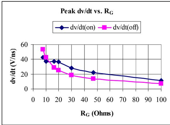
Figure 2 Peak drain dv/dt vs. gate resistance
