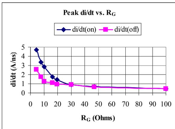
Figure 3 Peak drain di/dt vs. gate resistance
