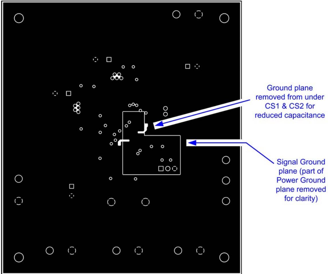
PCB LAYOUT GUIDE – INNER LAYER 2 – V1 & V2 POWER
