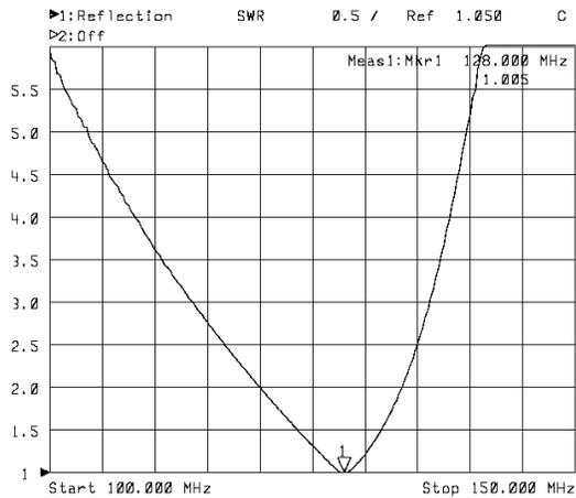
**Figure 2 Input VSWR vs Frequency**
