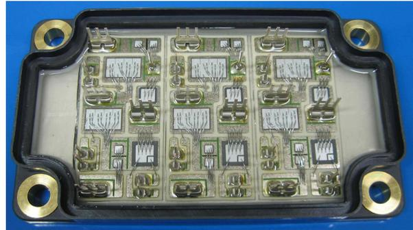
Fig.6 Picture of the open Microsemi power module
