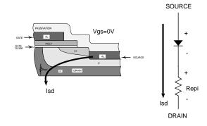
Fig. 11. Forward current flow in the Body Diode.
