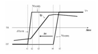
Fig. 6. Switch voltage and primary current relationship.
