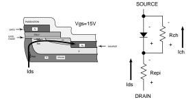
Fig. 14. Reverse current flow in the channel only.
