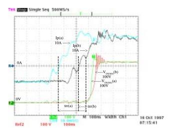
Fig. 7. Onset of MOSFET failure with short-circuit load
