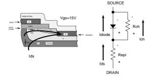
Fig. 13. Reverse current flow in the Body Diode and the channel.
