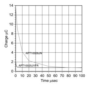
Fig. 17. Stored charge remaining in junction after forward current equals zero.
