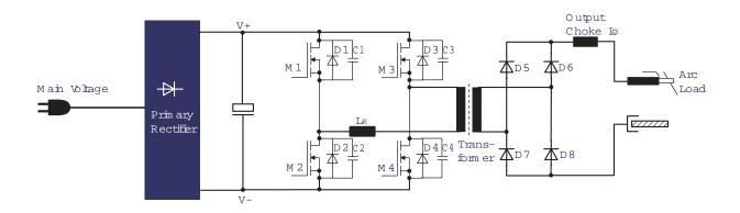
Fig. 1. Full bridge welding converter.
