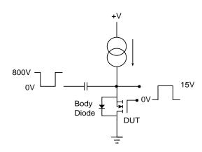
Fig. 16. Abbreviated schematic.
