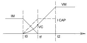
Fig.4 Turn off behaviour with snubber circuit connected across the switch.
