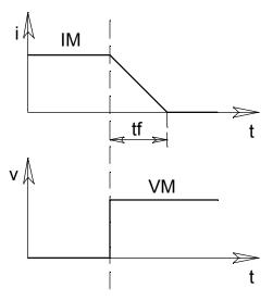
Fig.1 Switch turn-off behaviour with an inductive load
