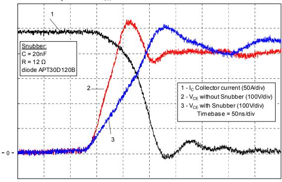
Fig. 6 Influence of 20nF snubber capacitor on turn off behaviour of an APTGF300A120 module
