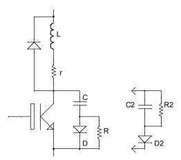
Fig.5 Chopper with turn-off snubber and over voltage protection circuit.
