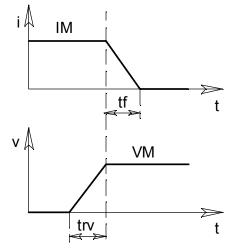
Fig.2 Experimental turnoff behaviour with an inductive load
