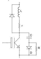
Fig. 3 Chopper with turn-off snubber circuit
