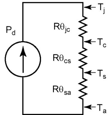
The transistor manufacturer sets the absolute limit on maximum junction temperature, which is then lowered by the designer to meet system reliability goals. The maximum ambient temperature is set by the system specifications. The designer must then provide the minimum heat sink impedance to satisfy these conditions.
