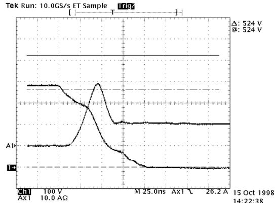
Figure 5 – MOSFET Turn-on,  $R_G = 4.7\Omega$  (APT5010B2VR)
