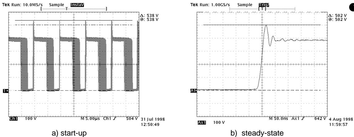
**Figure 7 – Drain Voltage at turn-off, APT5010LVR**
