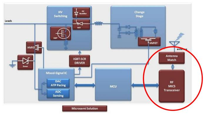
Area of focus – MICS Transceiver Circuit
