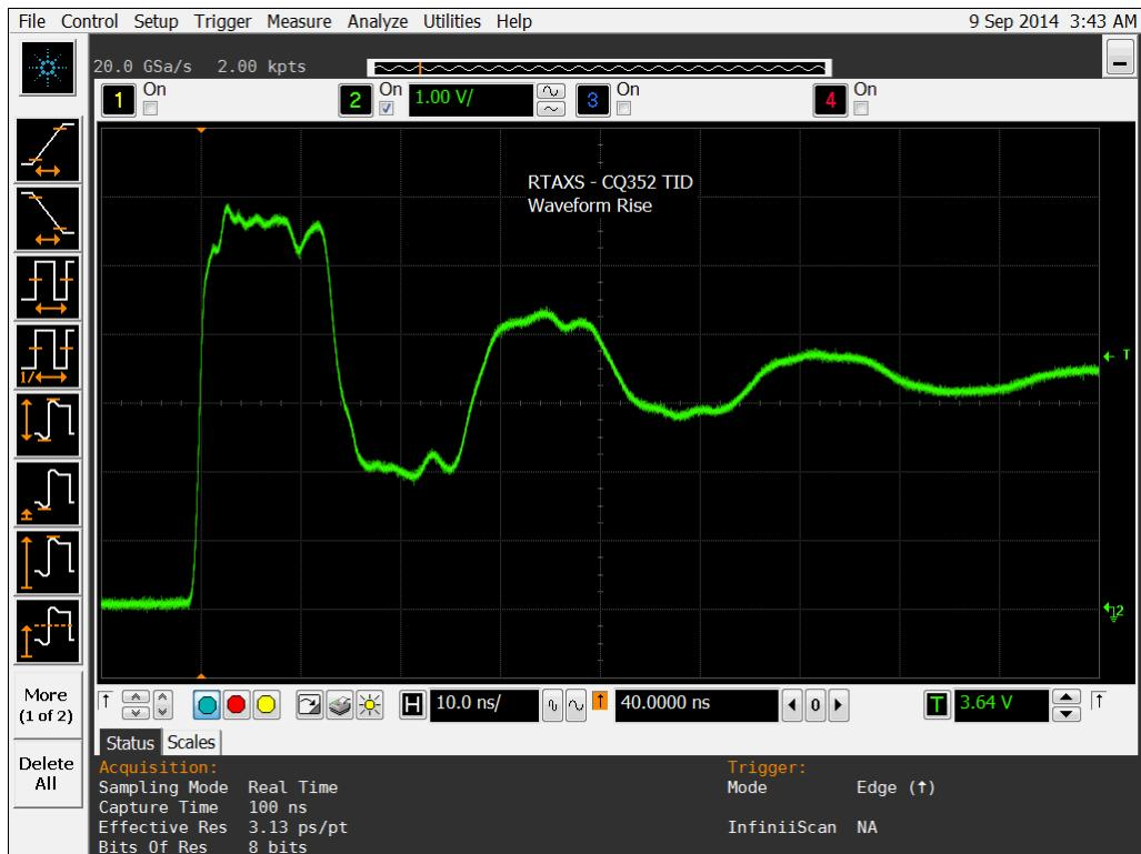
Figure 10b DUT 5764 Post-Annealing Rising Edge
