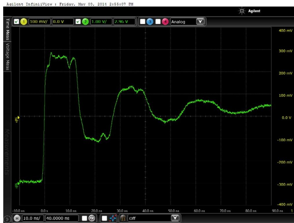
Figure 13a DUT 1595 Pre-Irradiation Rising Edge
