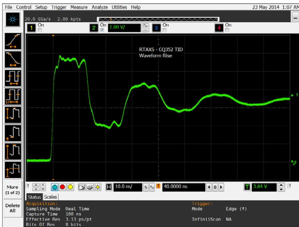
Figure 9b DUT 1553 Post-Annealing Rising Edge
