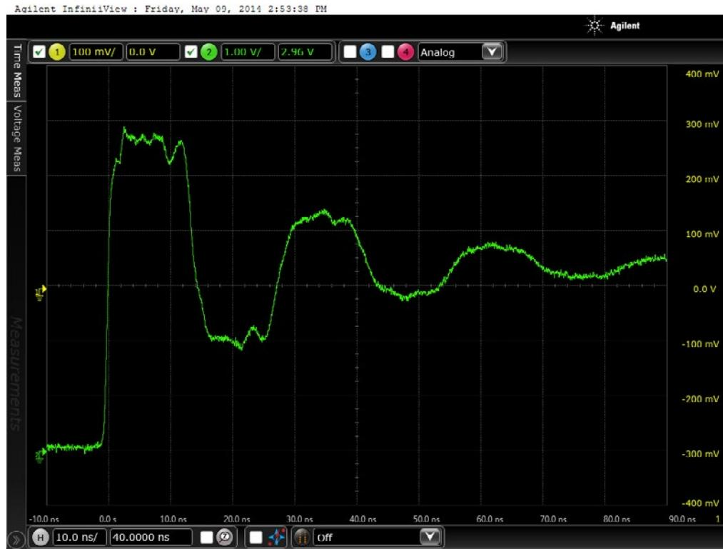
Figure 10a DUT 1564 Pre-Irradiation Rising Edge
