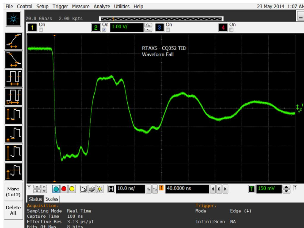
Figure 15b DUT 1553 Post-Annealing Falling Edge
