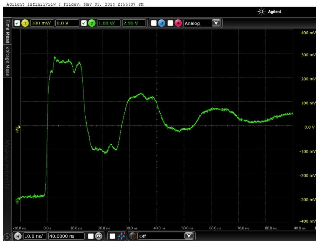
Figure 14a DUT 1610 Pre-Irradiation Rising Edge
