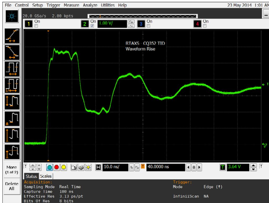
Figure 13b DUT 1595 Post-Annealing Rising Edge
