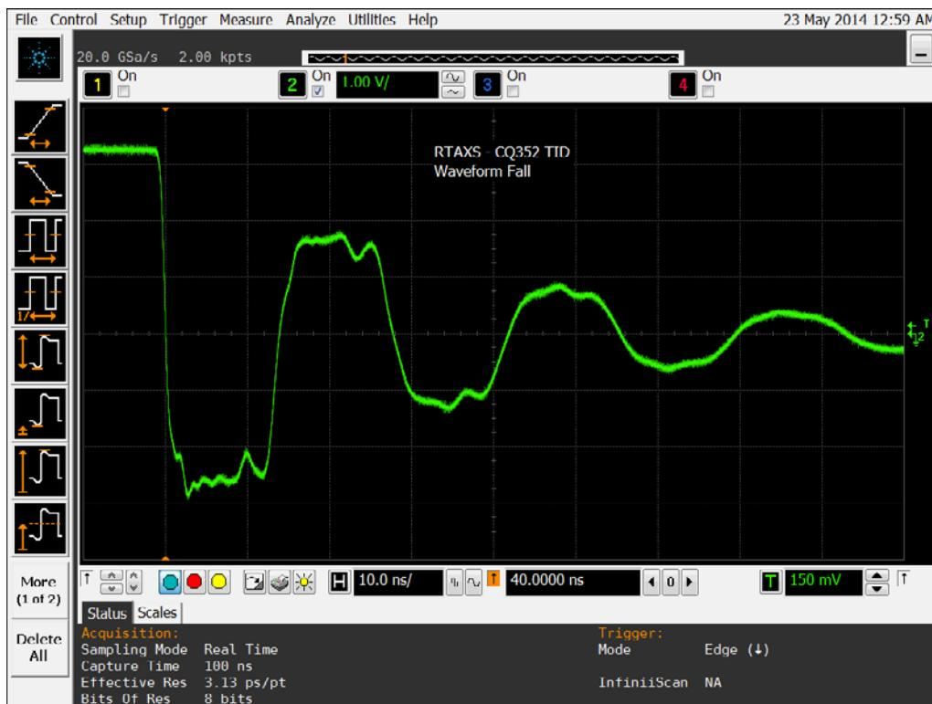
Figure 20b DUT 1610 Post-Annealing Falling Edge
