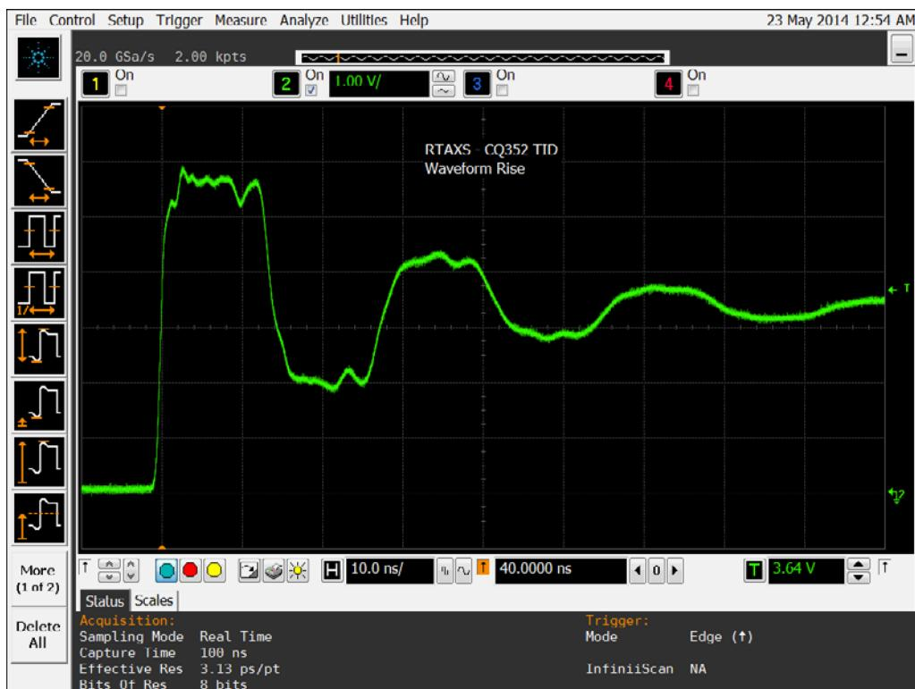
Figure 12b DUT 1585 Post-Annealing Rising Edge
