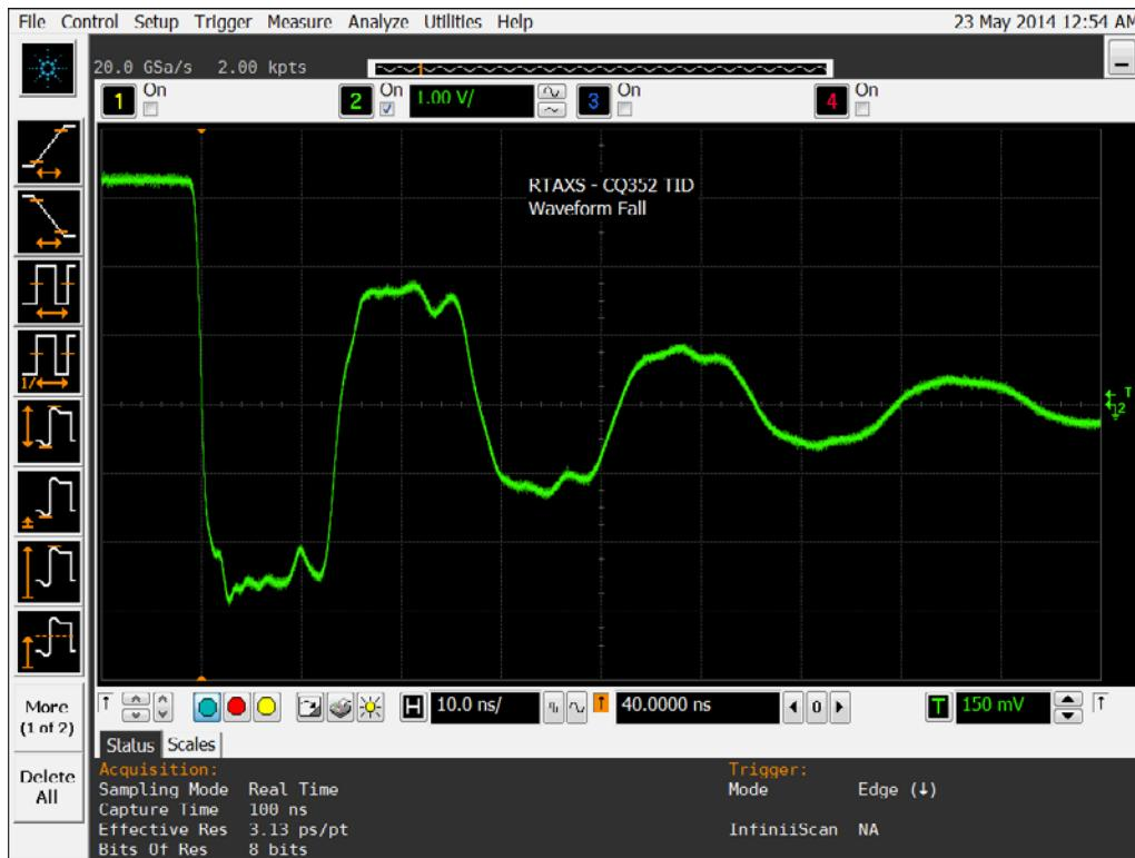
**Figure 18b DUT 1585 Post-Annealing Falling Edge**
