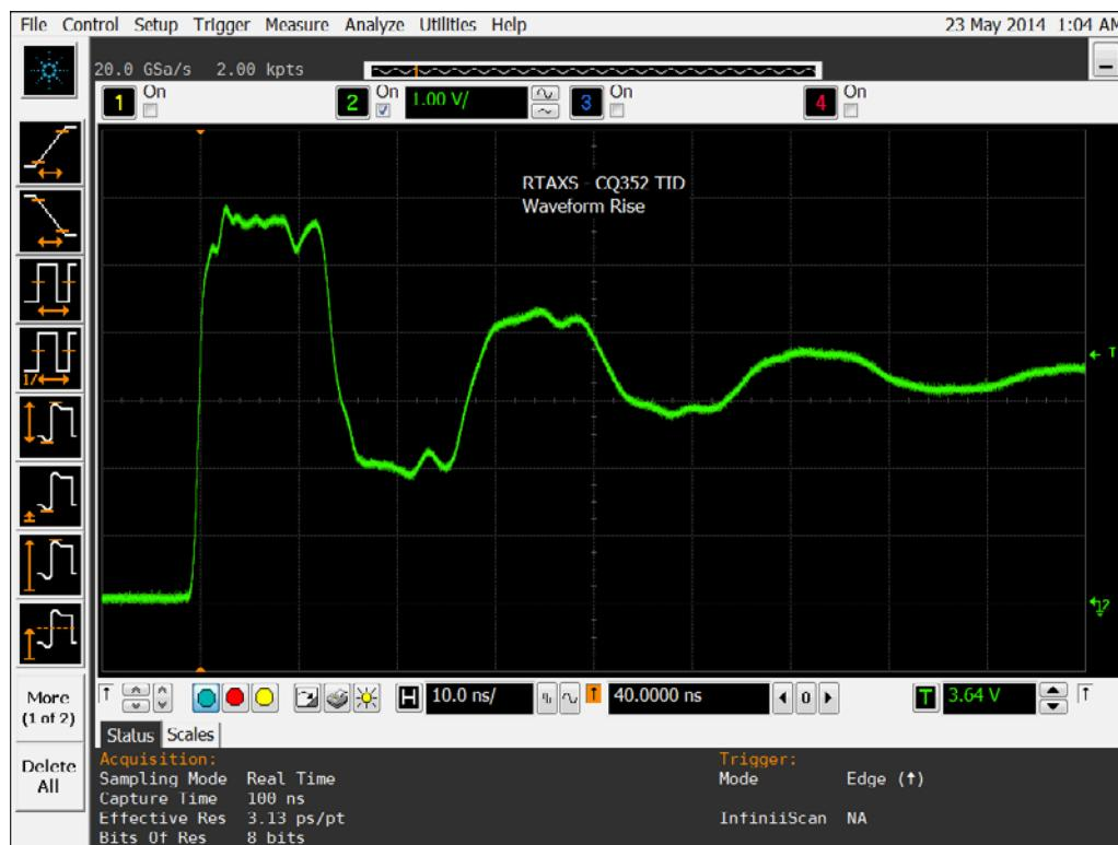
Figure 11b DUT 1575 Post-Annealing Rising Edge
