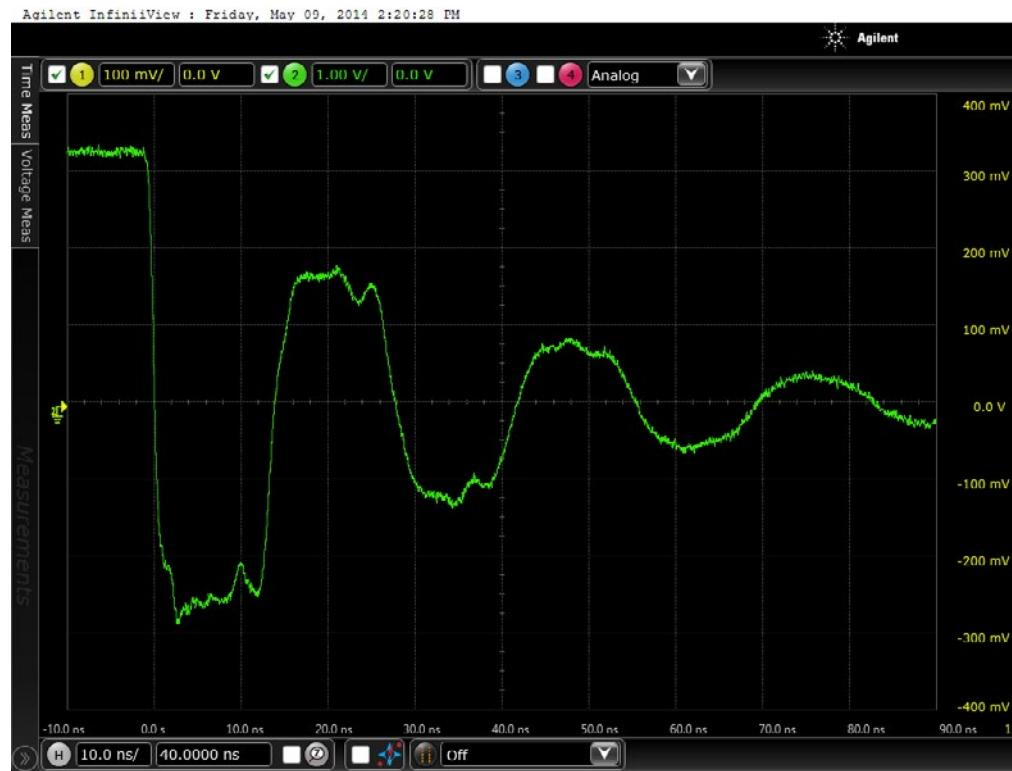
Figure 15a DUT 1553 Pre-Radiation Falling Edge
