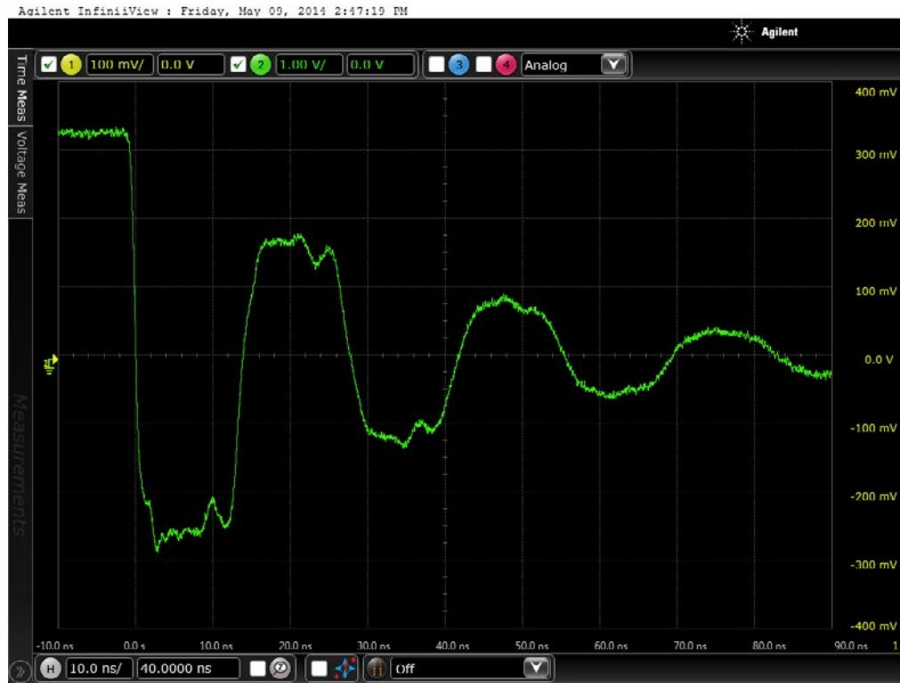
Figure 16a DUT 1564 Pre-Irradiation Falling Edge
