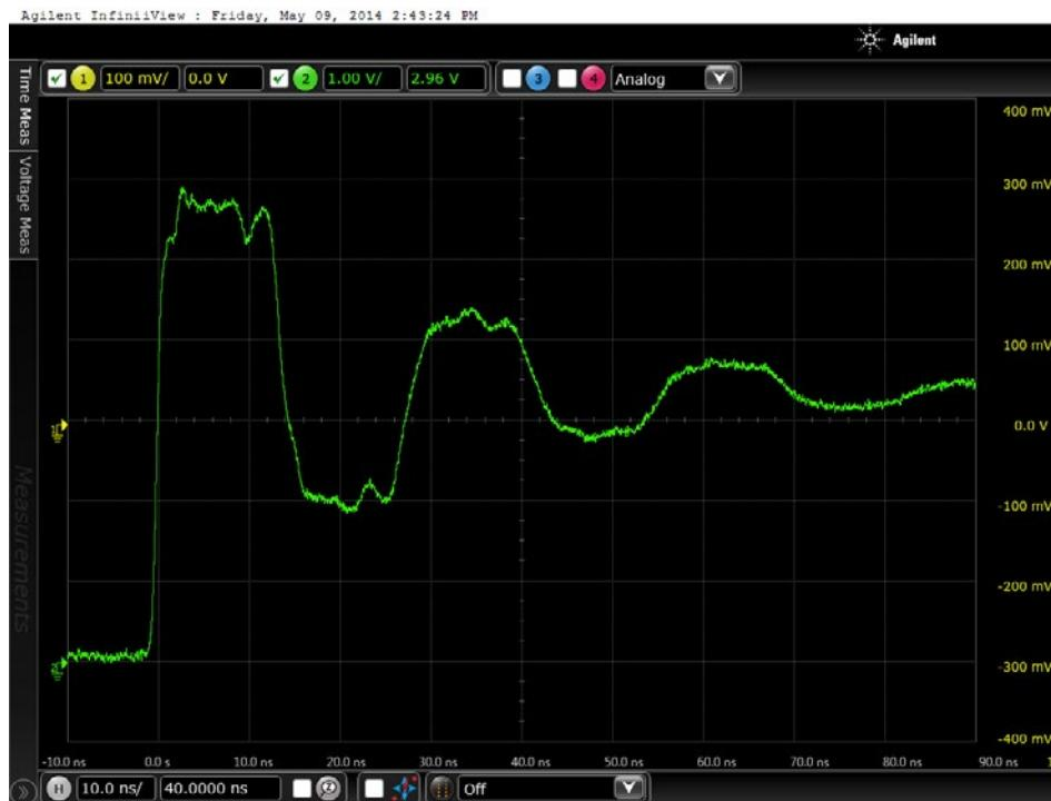
Figure 9a DUT 1553 Pre-Irradiation Rising Edge
