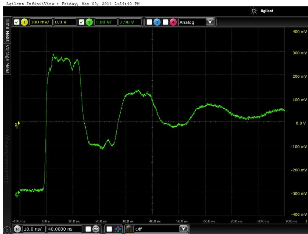
Figure 12a DUT 1585 Pre-Irradiation Rising Edge
