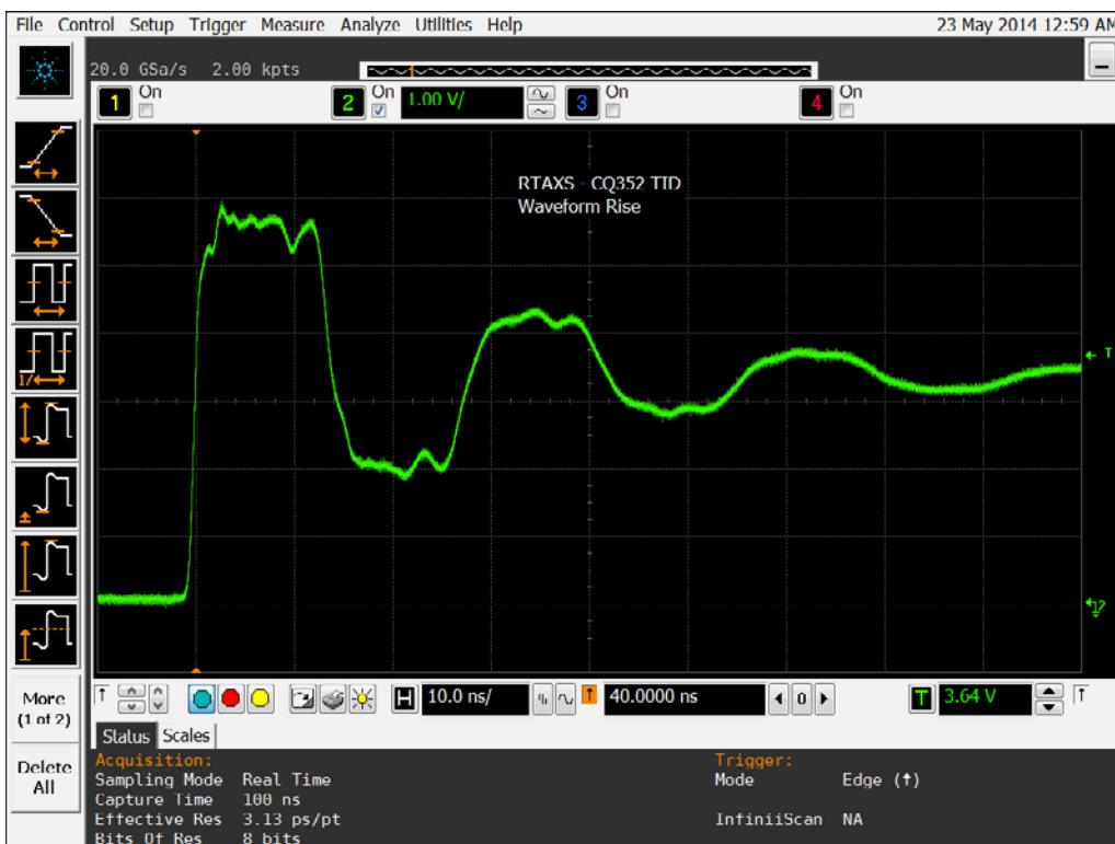
Figure 14b DUT 1610 Post-Annealing Rising Edge
