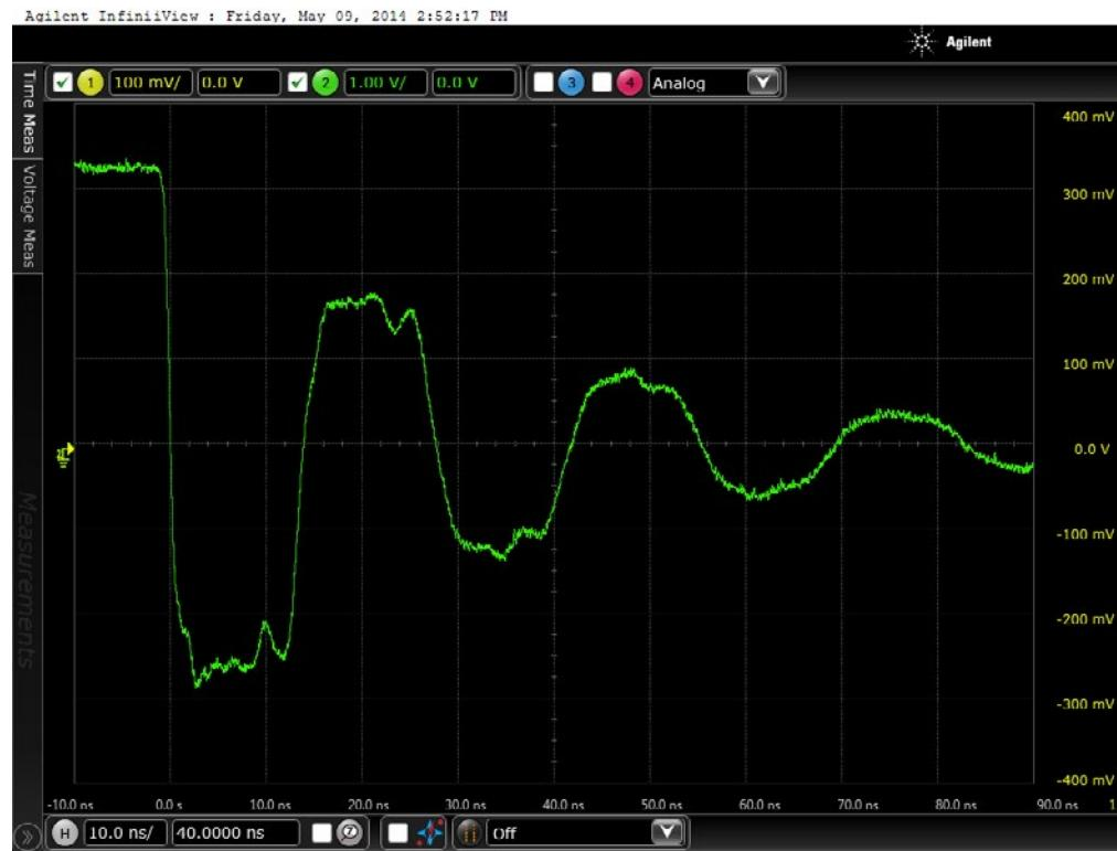
Figure 19a DUT 1595 Pre-Irradiation Falling Edge
