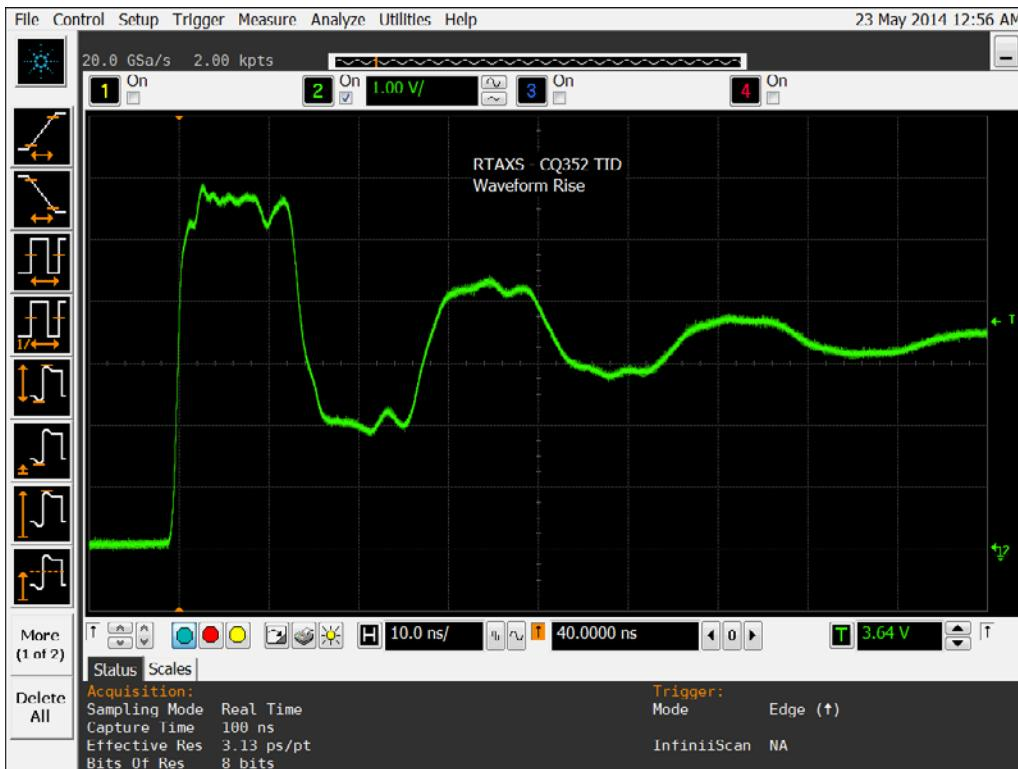
Figure 10b DUT 1564 Post-Annealing Rising Edge
