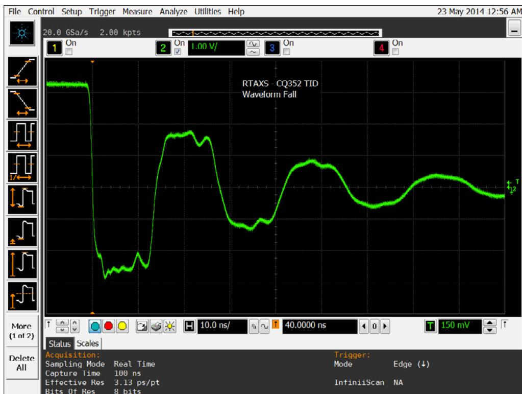
Figure 16b DUT 1564 Post-Annealing Falling Edge
