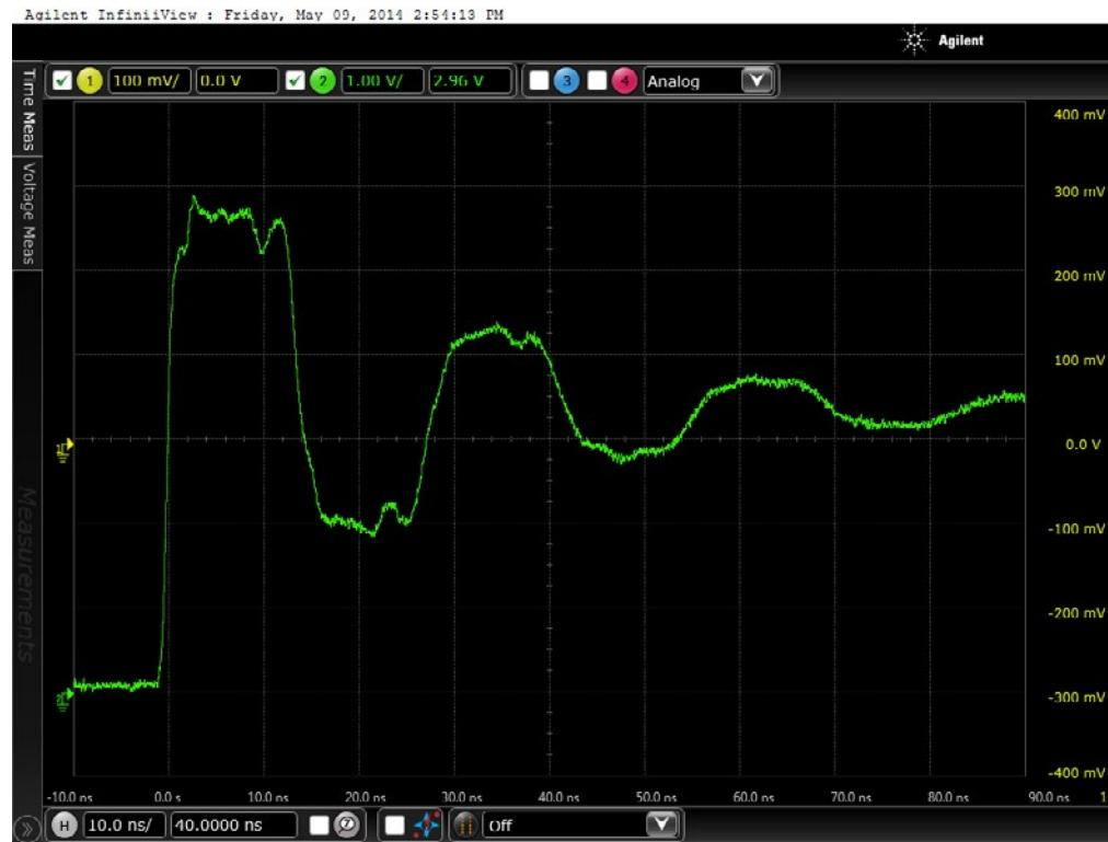
Figure 11a DUT 1575 Pre-Radiation Rising Edge
