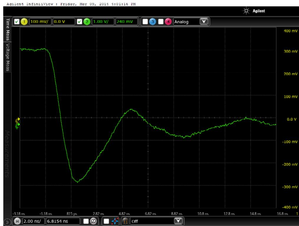
Figure 15b DUT 15128 Post-Annealing Falling Edge
