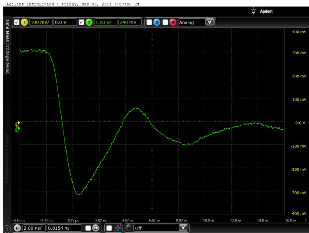
Figure 18b DUT 15140 Post-Annealing Falling Edge
