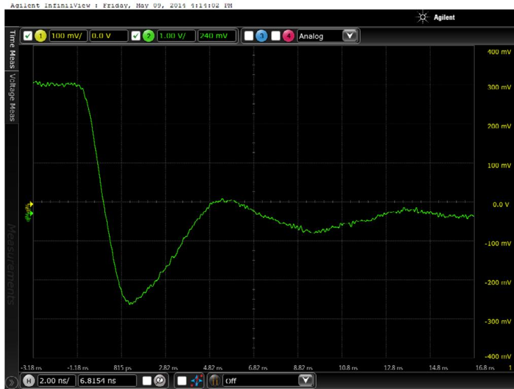
Figure 16a DUT 15129 Pre-Irradiation Falling Edge
