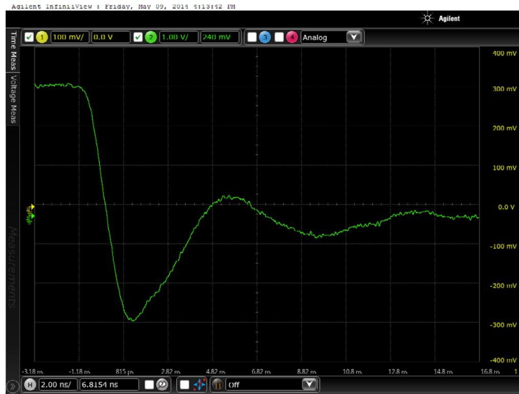
Figure 15a DUT 15128 Pre-Radiation Falling Edge
