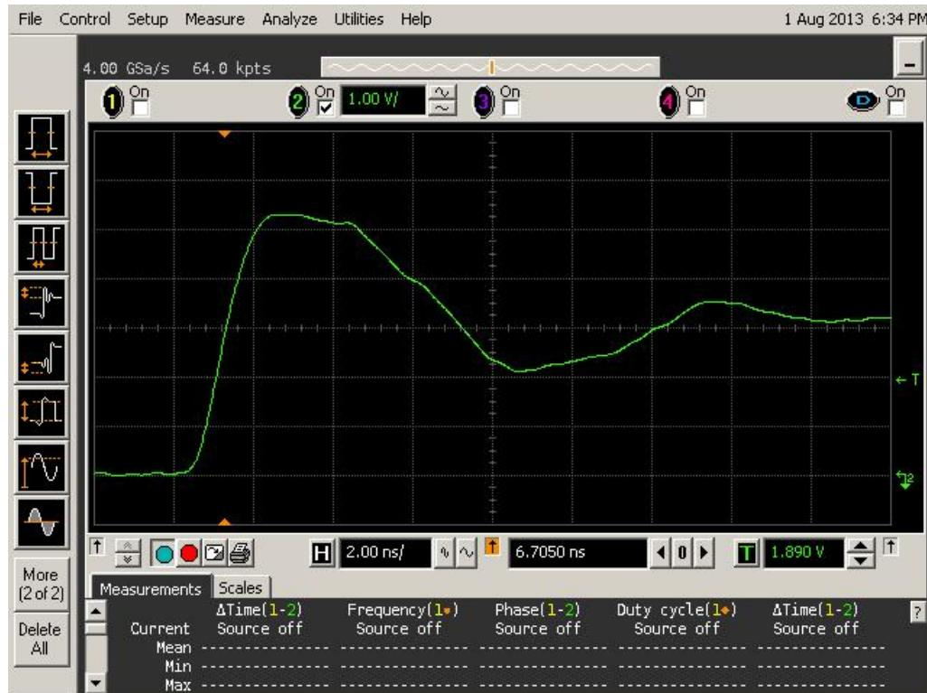
Figure 12a DUT 6645 Pre-Irradiation Rising Edge
