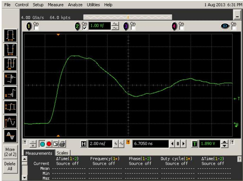
Figure 9a DUT 6583 Pre-Irradiation Rising Edge
