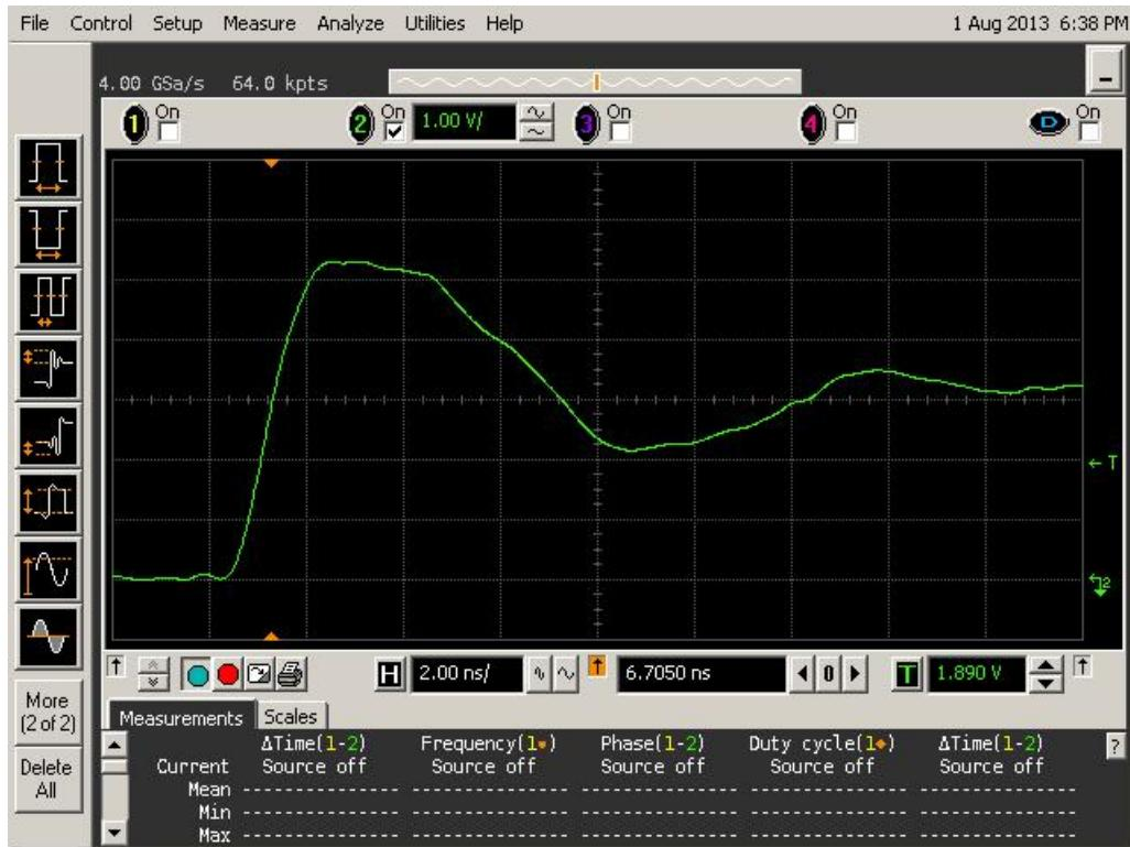
Figure 11a DUT 6621 Pre-Radiation Rising Edge
