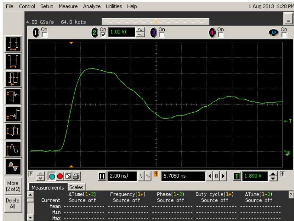
Figure 10a DUT 6606 Pre-Irradiation Rising Edge
