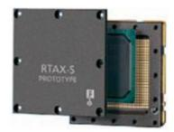
Prototyping board for RTAX2000S/CCGA624 or AX2000/FBGA896 is available from Cobham Gaisler
