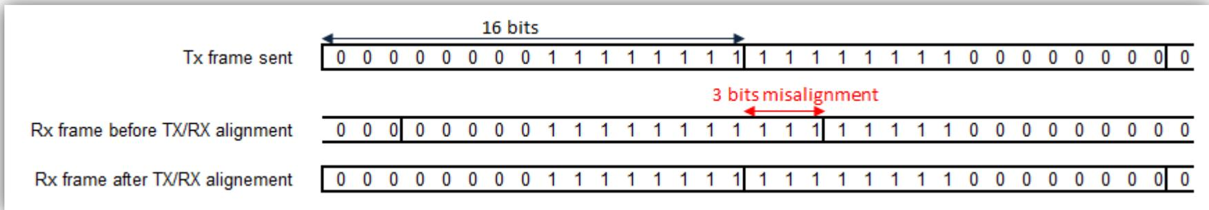
To correct frame misalignment, TX sends a known sequence for 32 frames used by RX to align its 16bits word to the TX frames.
