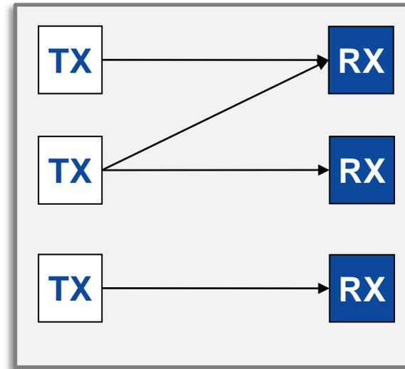
In case of multiple lanes configuration, in order to avoid cross-lane correlation issues the PRBS sequences between lanes should not be aligned.
