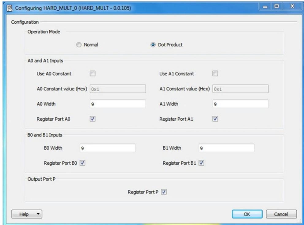
**Figure 1-2 • Hard Multiplier Configuration Options - Dot Product Mode**
