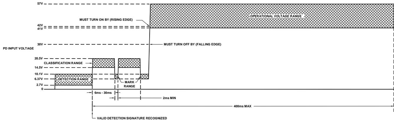
802.3at TYPE 2 and HDBaseT PD INPUT REQUIREMENTS
