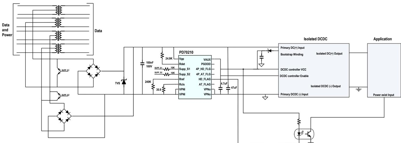
Figure 5: Typical 2 or 4 Pair Configuration with a Single PD70210 IC
