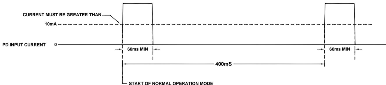
Figure 3: PoE Maintain Power Signature (MPS) Requirements
