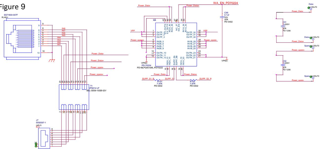
Figure 9: Type 3 HDBASET front end- connector and diode bridge(1 of 2)
