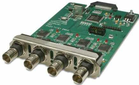
The E1 Output provides 2 MHz and 2 Mbit/sec outputs meeting the requirements of ITU-TG.703.10 and ITU-T G.703.6
