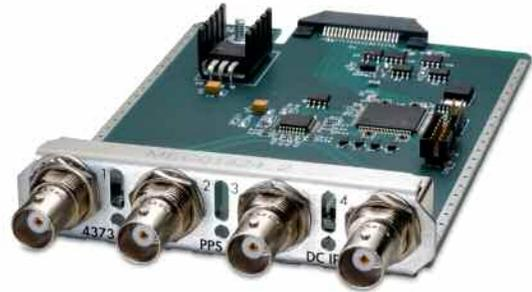
The 1PPS output card provides pulse outputs through four BNC connectors. These outputs are phase locked to the host receiver's disciplined reference oscillator. They are automatically enabled upon initialization and are independently selectable by the user with no configuration setup required.
