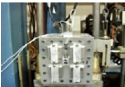
(+) Y-axis Shock (Specified Pulse) Test Setup.
