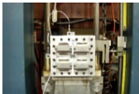
(-) X-axis Shock (Specified Pulse) Test Setup
