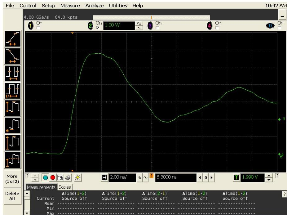
Figure 11a DUT 14678 Pre-Irradiation Rising Edge
