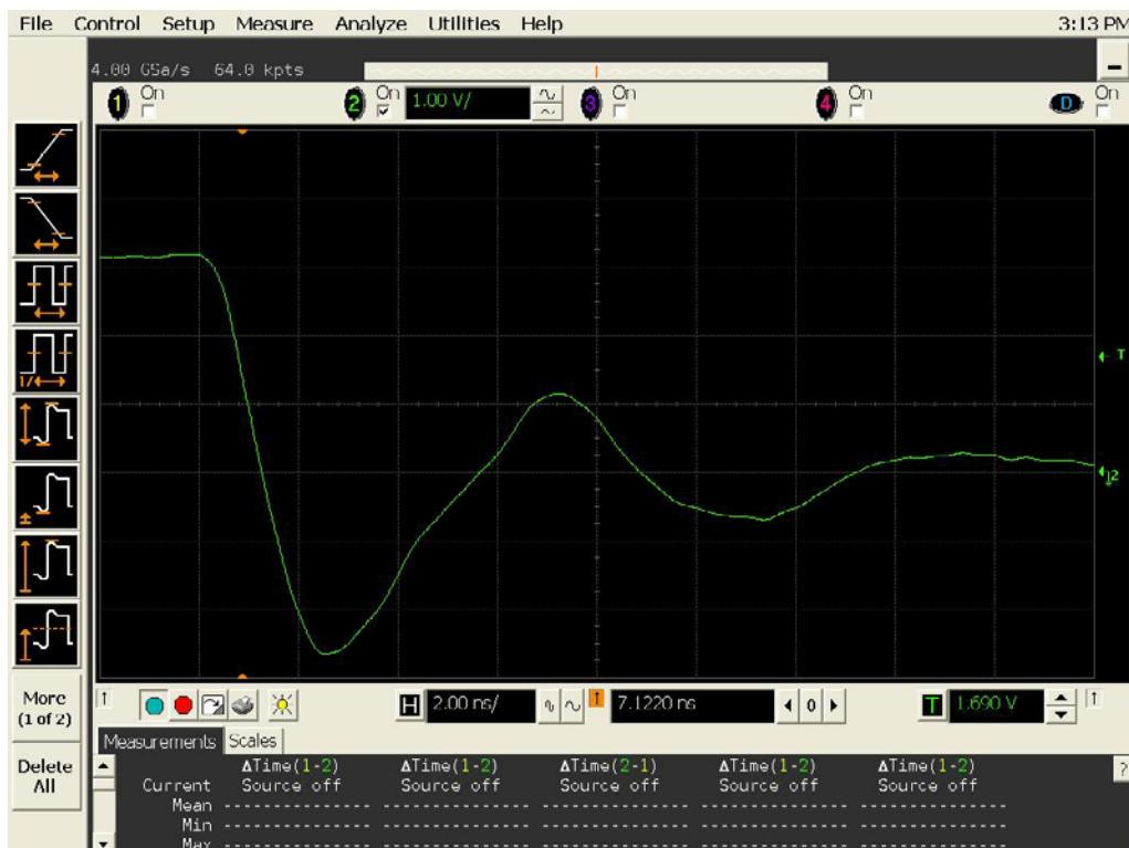
Figure 19b DUT 11460 Post-Annealing Falling Edge,
