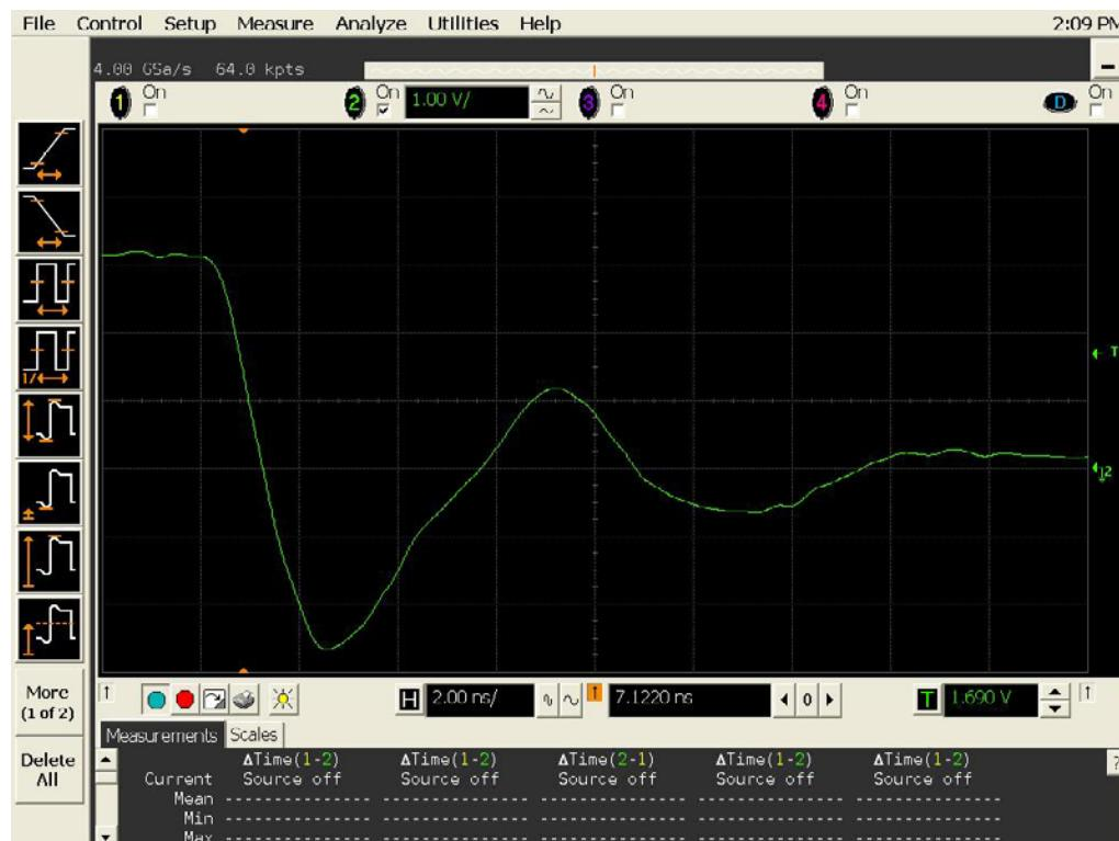
**Figure 18b DUT 11457 Post-Annealing Falling Edge,
