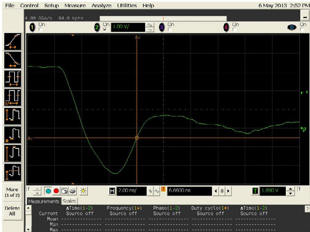
Figure 16a DUT 2245 Pre-Irradiation Falling Edge
