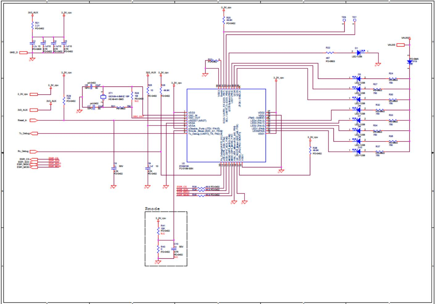
**Figure 4: PD39100 PoE Controller Circuitry**
