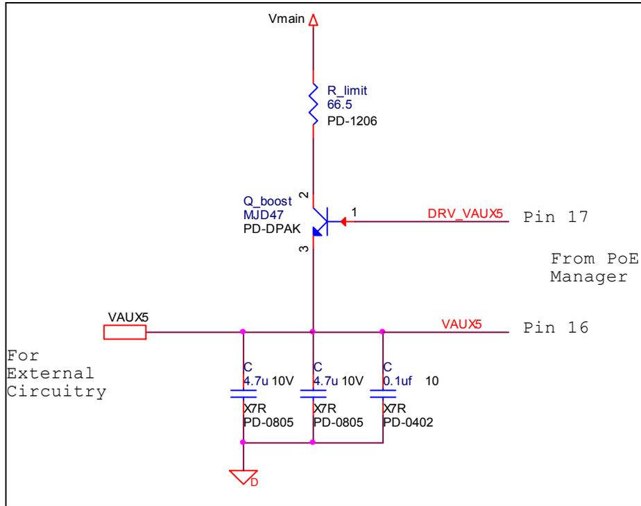
**Figure 9: Optional Boost Transistor Circuitry**
