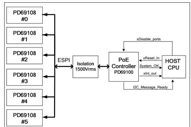
**Figure 3: Control and Indication Signals**
