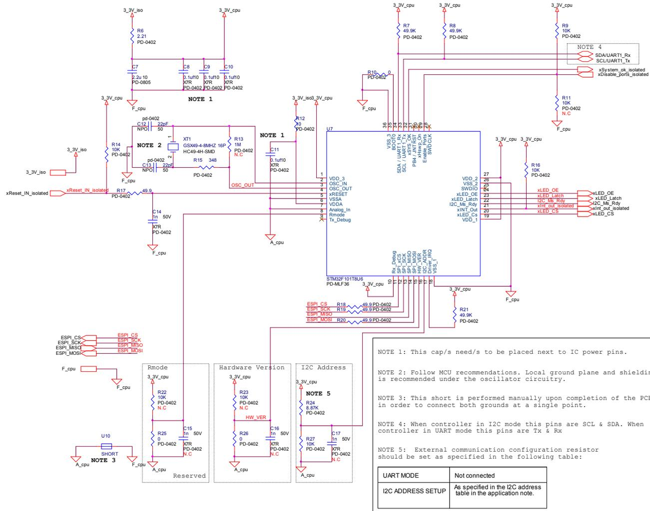
Figure 7: PD69100 PoE Controller Circuitry
