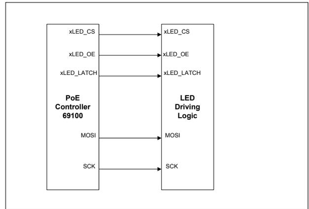
**Figure 4: SPI Bus and LED Support**
