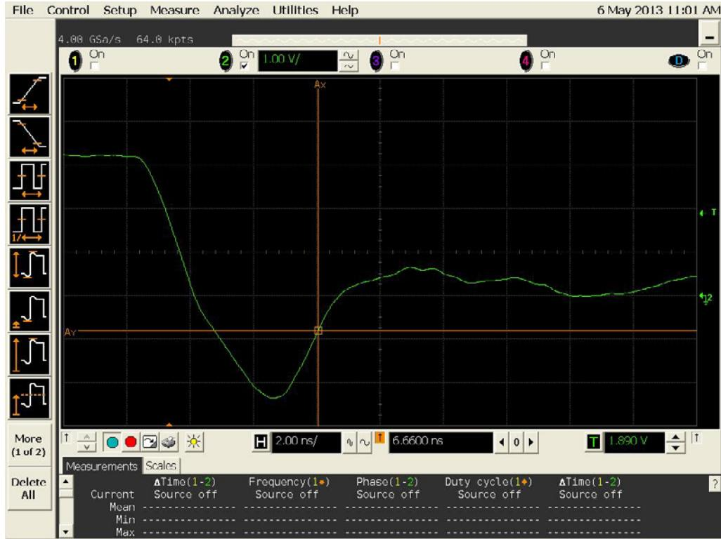
Figure 20a DUT 13233 Pre-Irradiation Falling Edge
