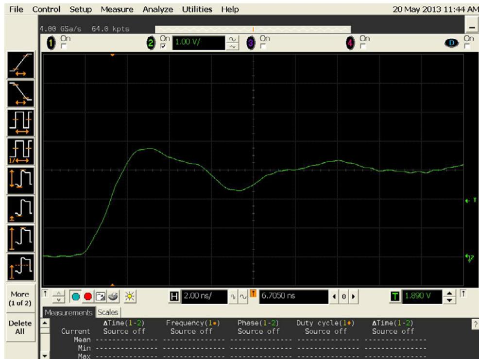
Figure 9b DUT 13199 Post-Annealing Rising Edge
