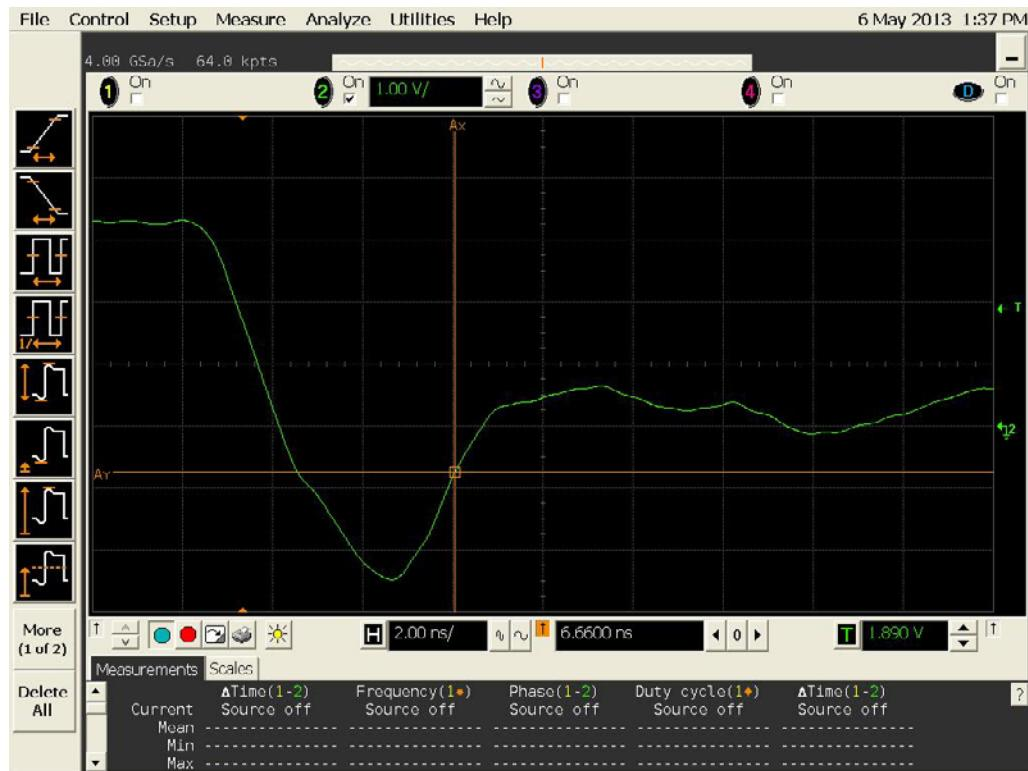
Figure 18a DUT 13207 Pre-Irradiation Falling Edge
