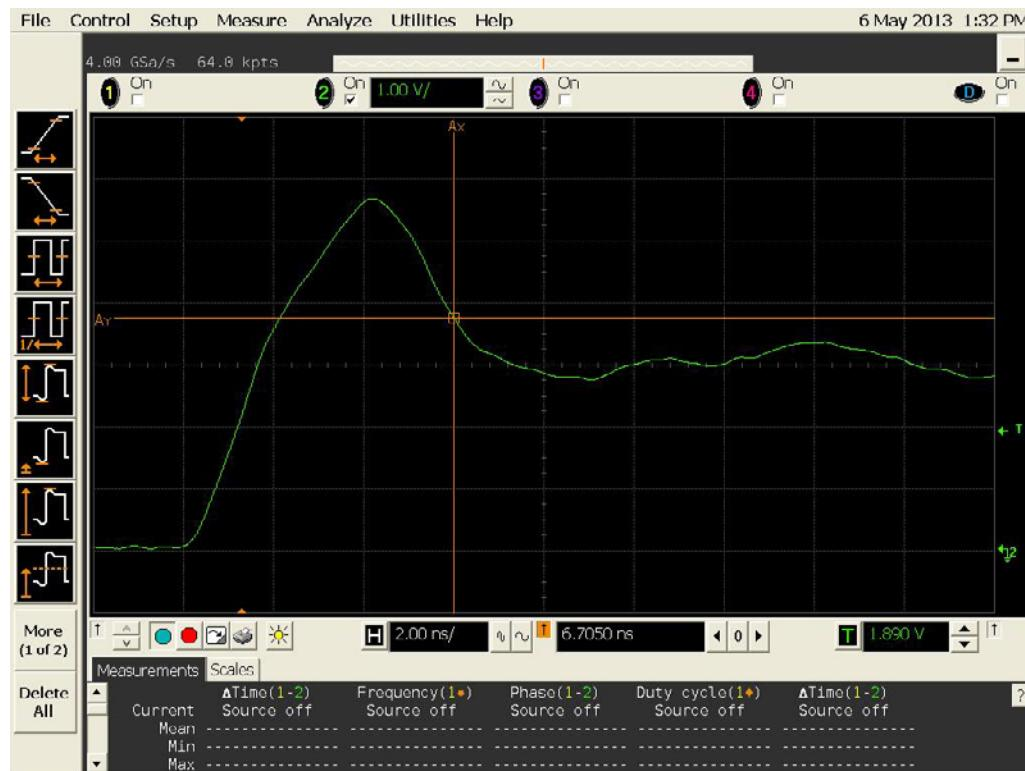
Figure 11a DUT 13205 Pre-Radiation Rising Edge
