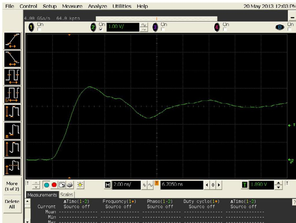
Figure 13b DUT 13224 Post-Annealing Rising Edge
