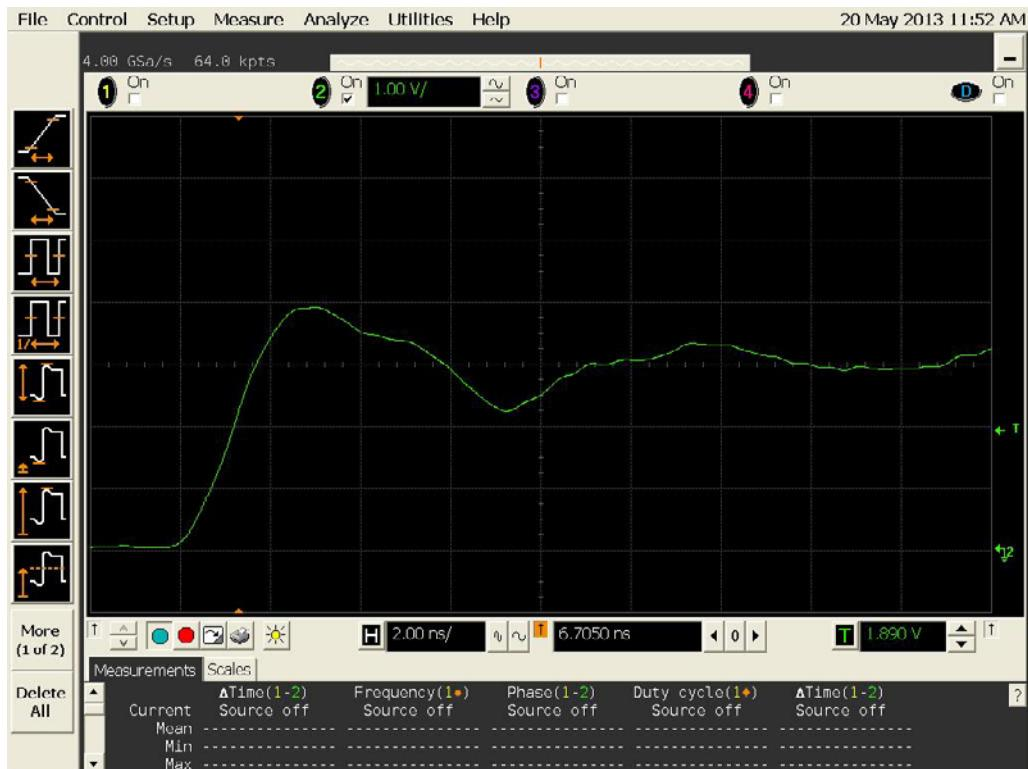
Figure 10b DUT 13202 Post-Annealing Rising Edge
