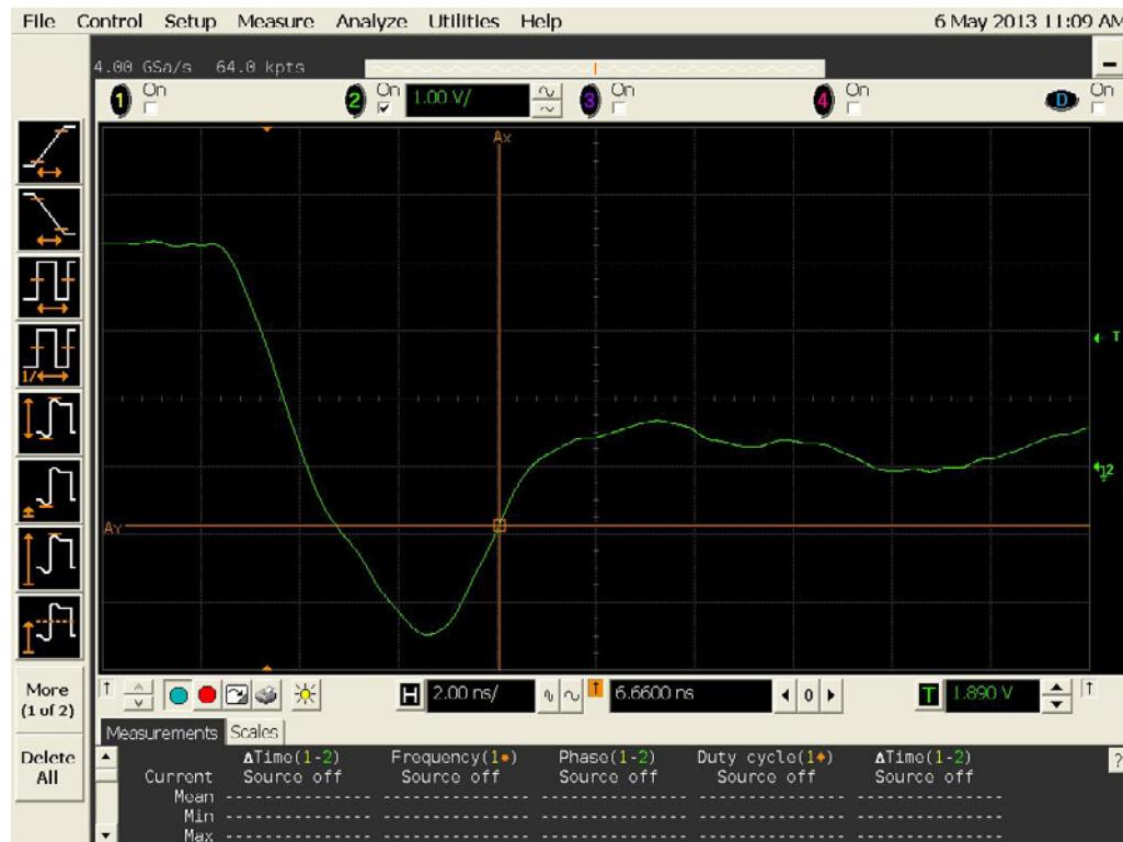
Figure 19a DUT 13224 Pre-Irradiation Falling Edge
