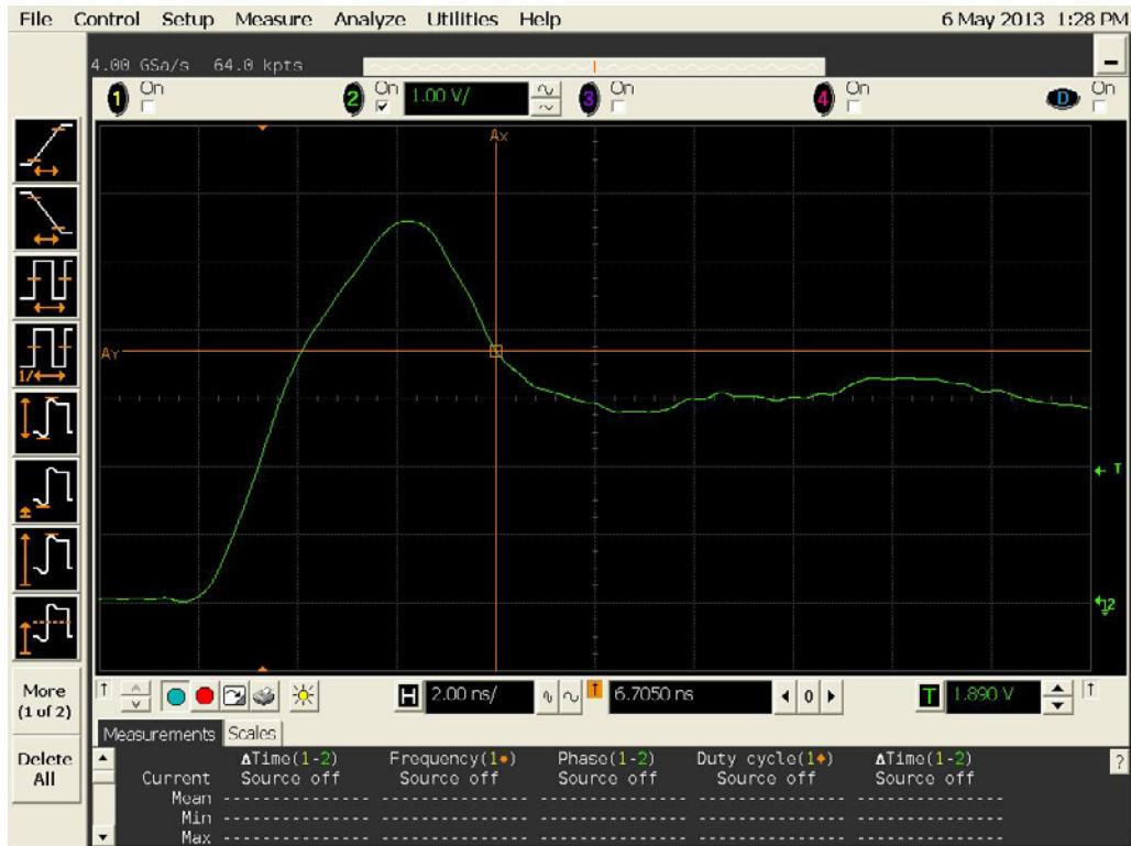
Figure 10a DUT 13202 Pre-Irradiation Rising Edge
