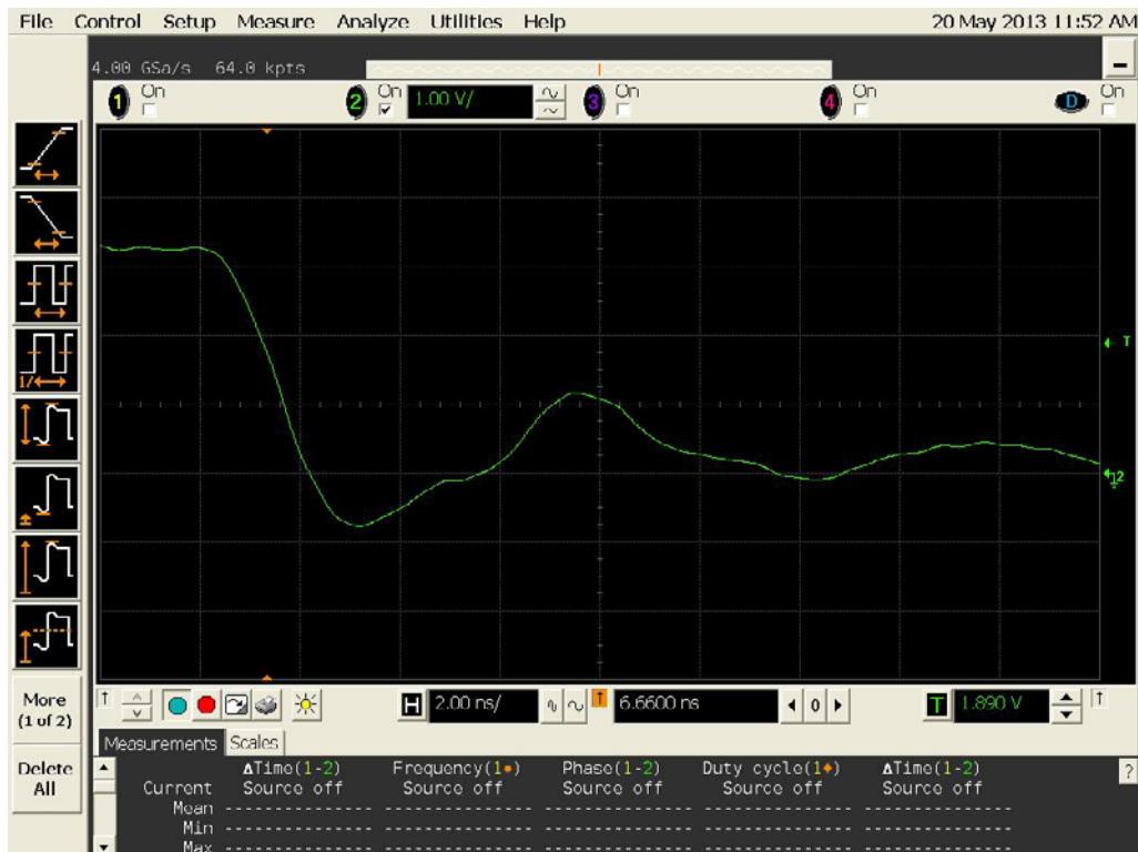
Figure 16b DUT 13202 Post-Annealing Falling Edge
