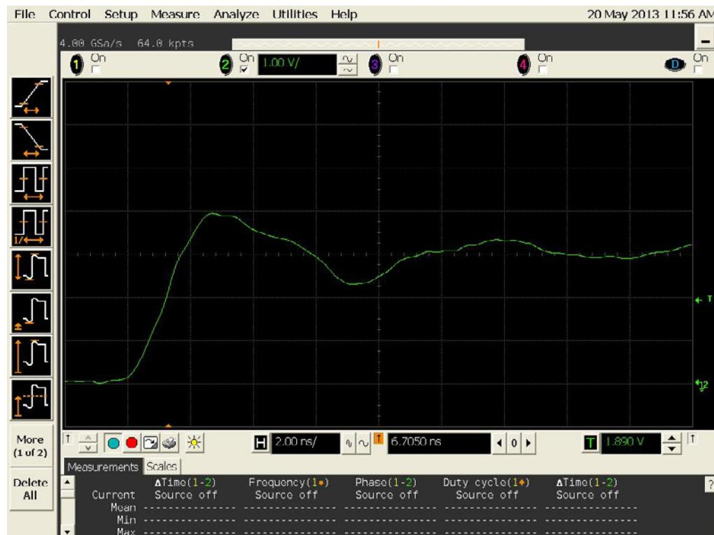
Figure 11b DUT 13205 Post-Annealing Rising edge
