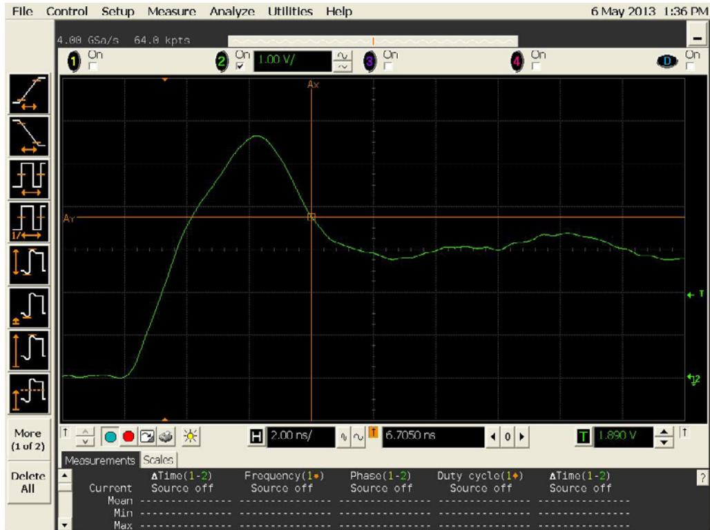
Figure 12a DUT 13207 Pre-Irradiation Rising Edge
