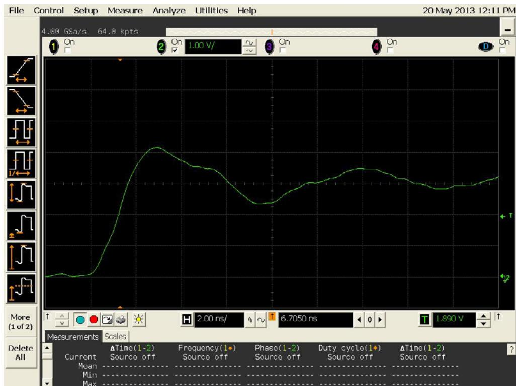
Figure 14b DUT 13233 Post-Annealing Rising Edge
