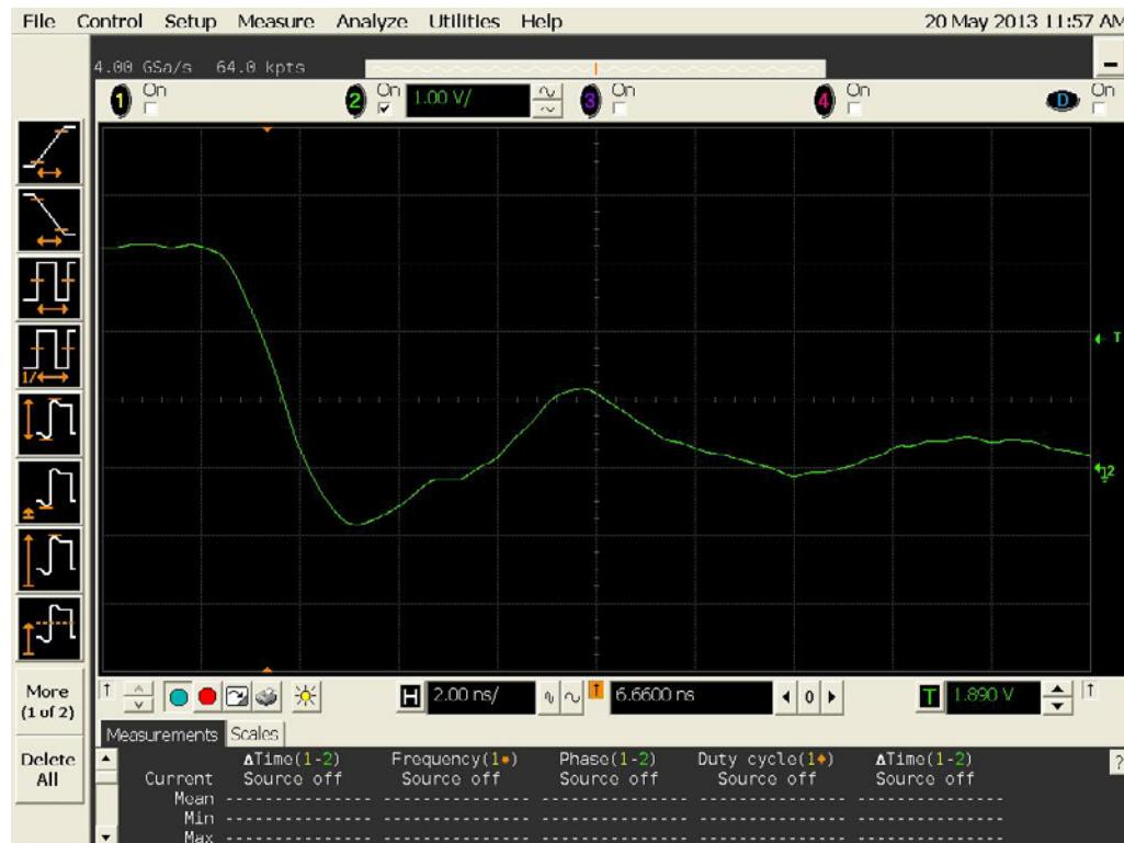
Figure 17b DUT 13205 Post-Annealing Falling Edge
