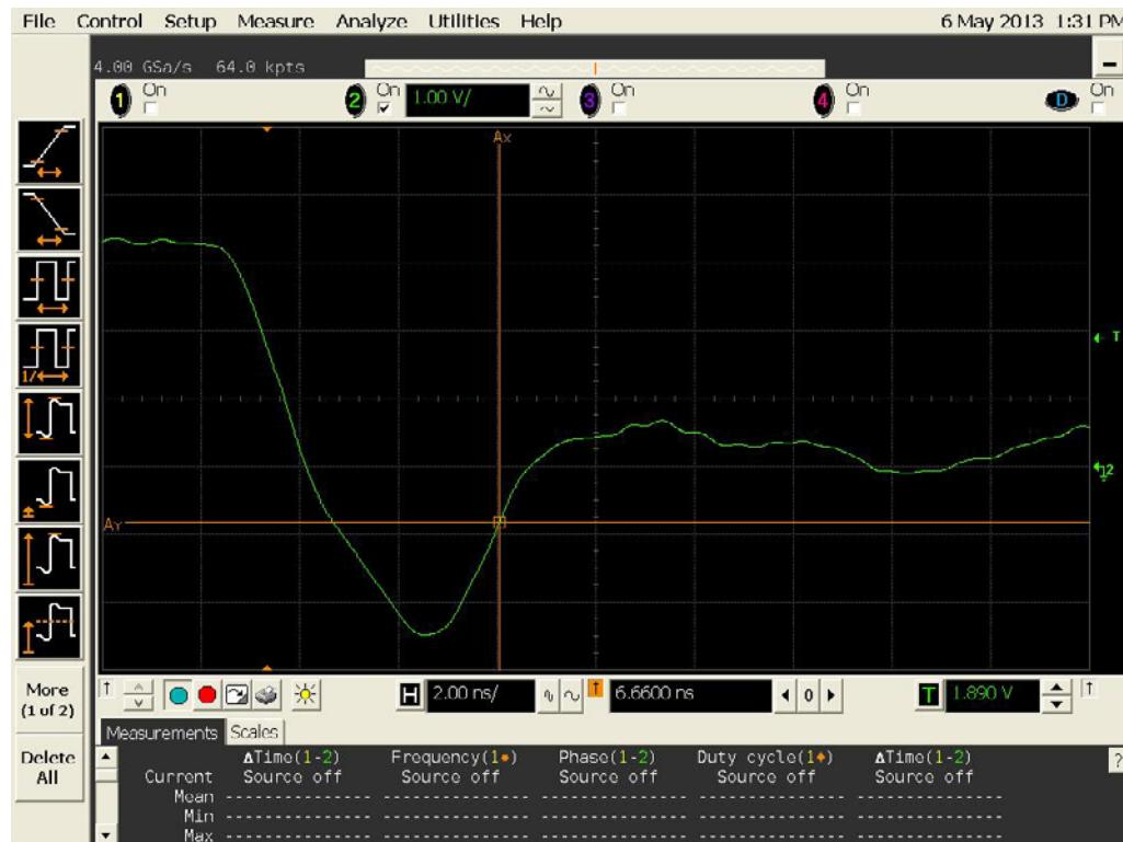
Figure 17a DUT 13205 Pre-Irradiation Falling Edge
