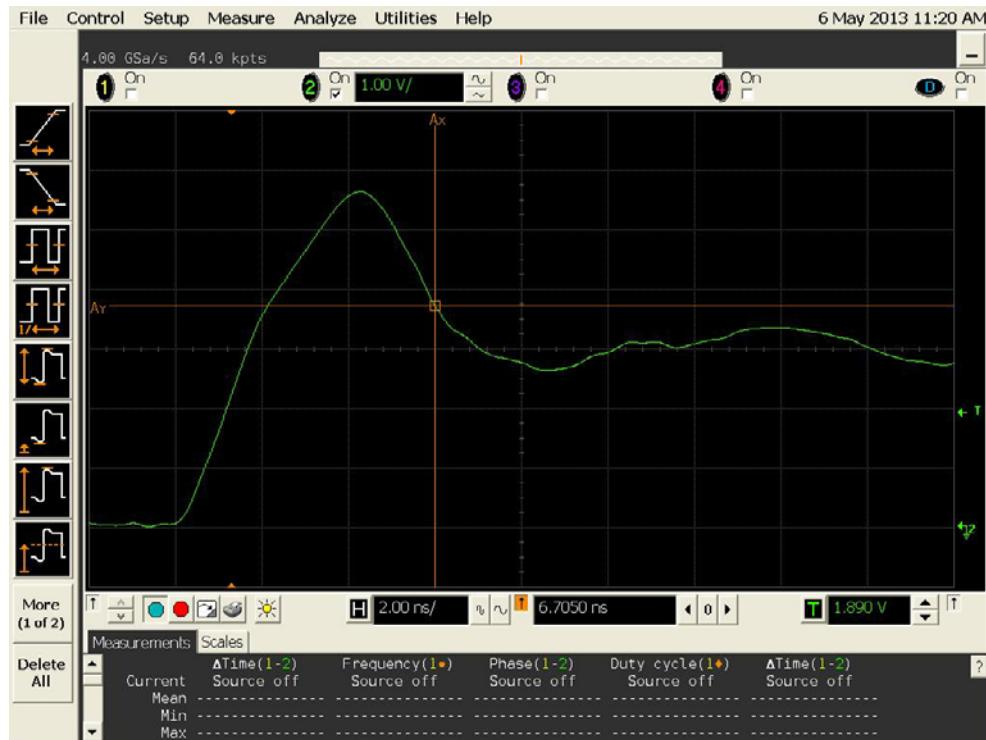
Figure 9a DUT 13199 Pre-Irradiation Rising Edge
