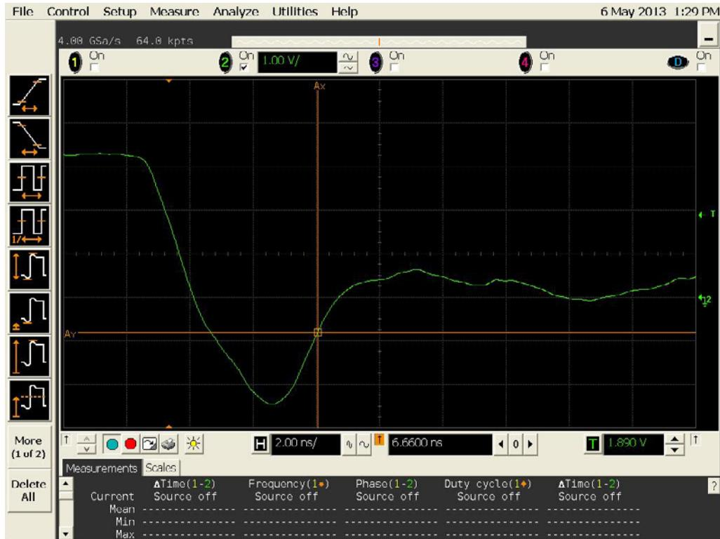
Figure 16a DUT 13202 Pre-Irradiation Falling Edge
