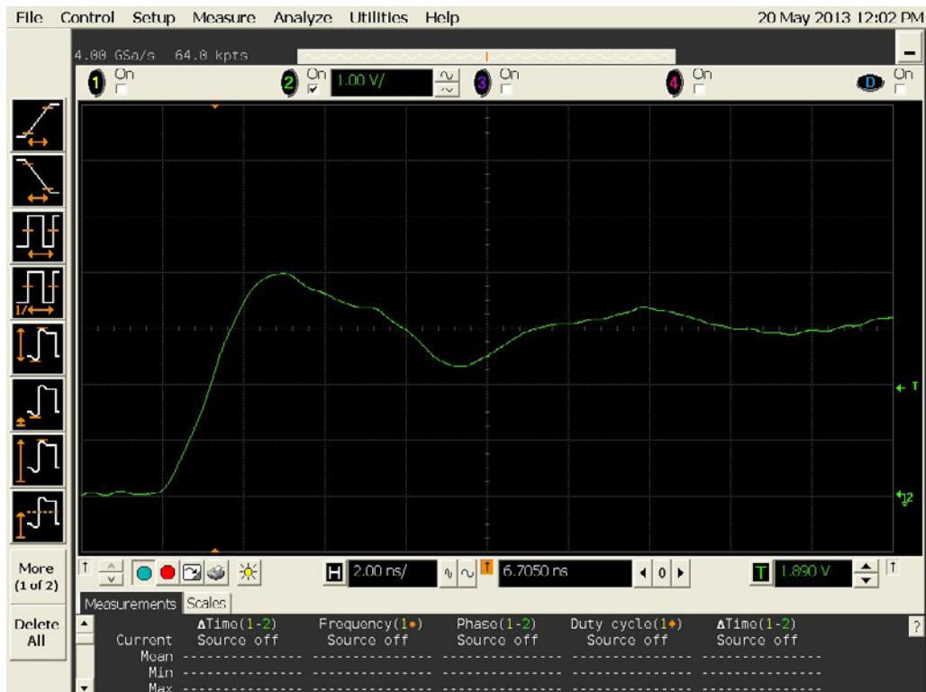
Figure 12b DUT 13207 Post-Annealing Rising Edge
