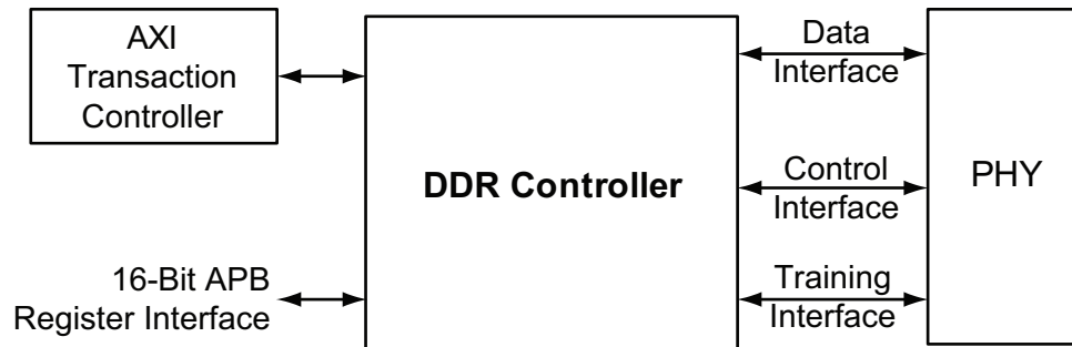
Figure 1-6. DDR Controller Block Diagram
