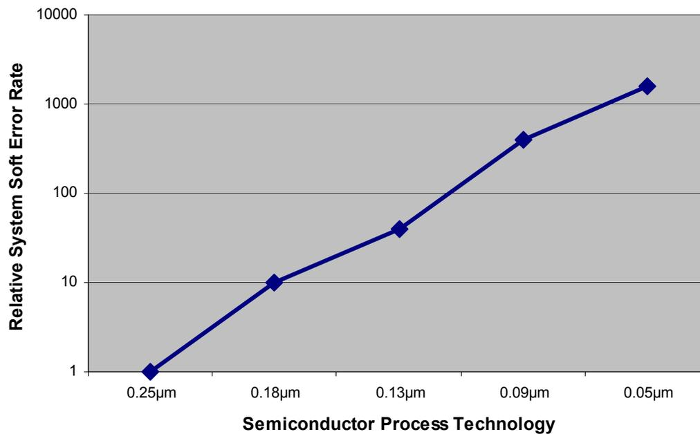
**Figure 4:** Soft Error Rates as a Function of IC Process Technology<sup>4</sup>
