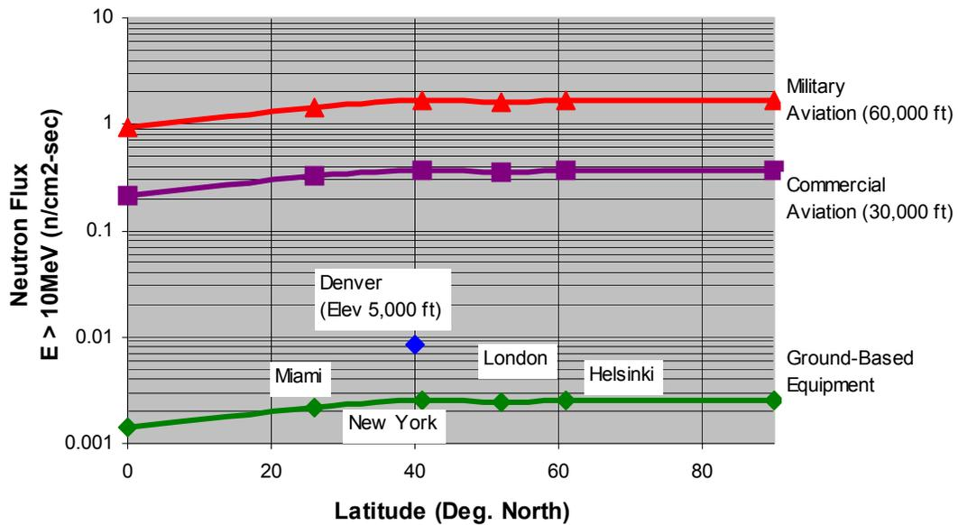
Figure 2: Neutron Flux as a Function of Altitude and Latitude<sup>2</sup>
