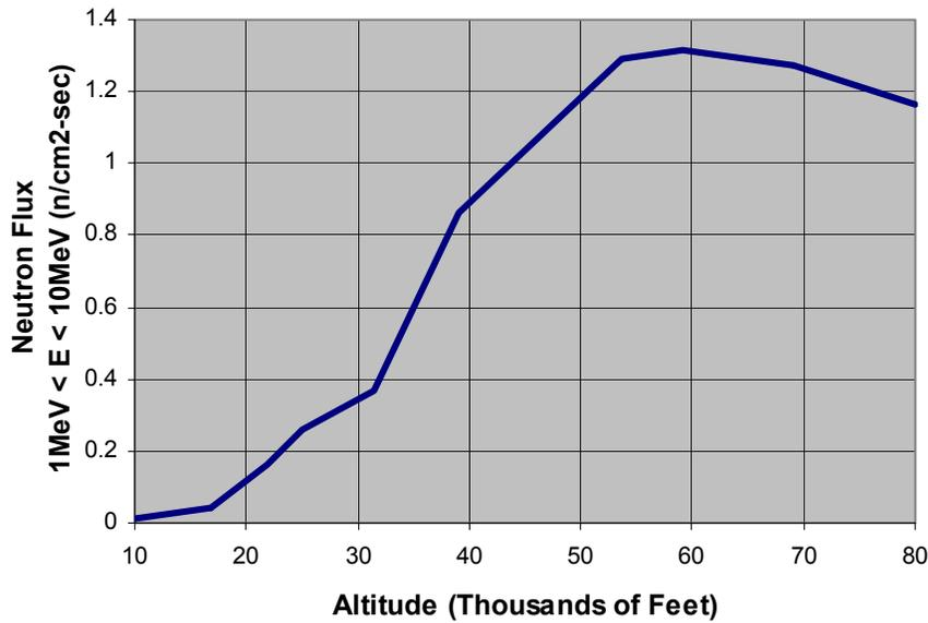
Figure 1: Neutron Flux as a Function of Altitude<sup>1</sup>
