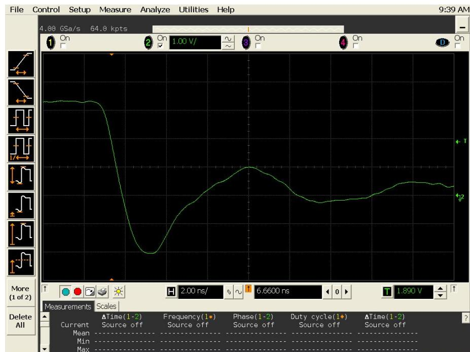
Figure 12a DUT 12008 Pre-Irradiation Falling Edge,
