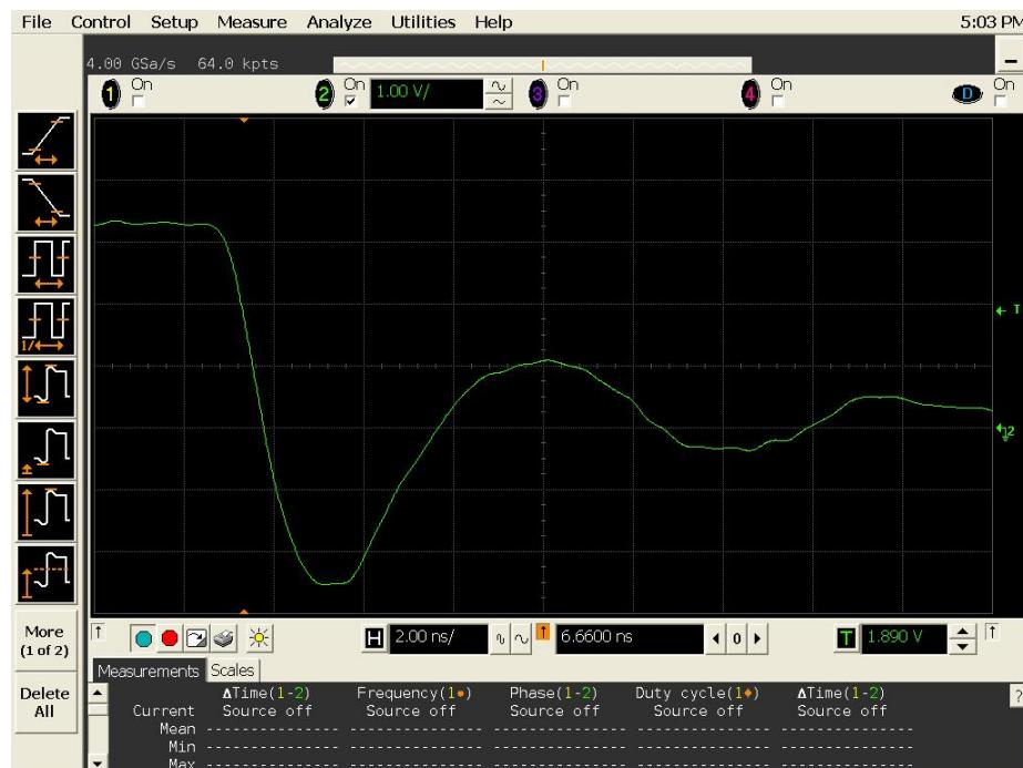
Figure 14b DUT 12025 Post-Annealing Falling Edge,
