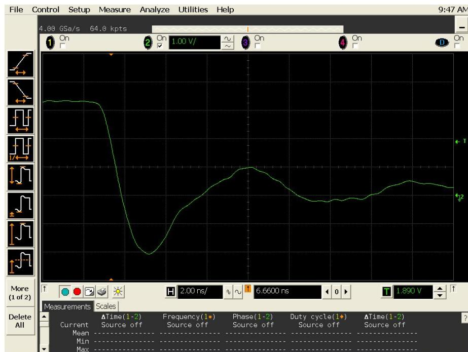
**Figure 15a DUT 12030 Pre-Irradiation Falling Edge,
