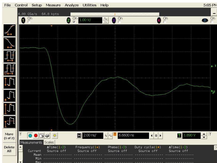
**Figure 15b DUT 12030 Post-Annealing Falling Edge,
