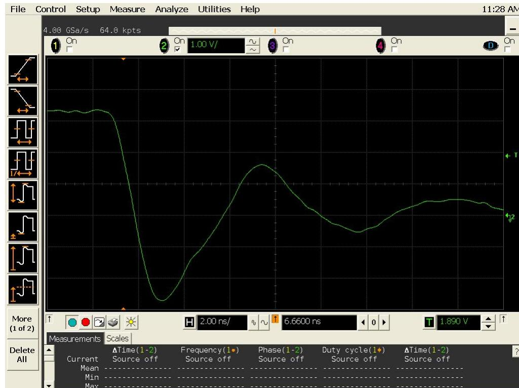
Figure 18b DUT 5800 Post-Annealing Falling Edge
