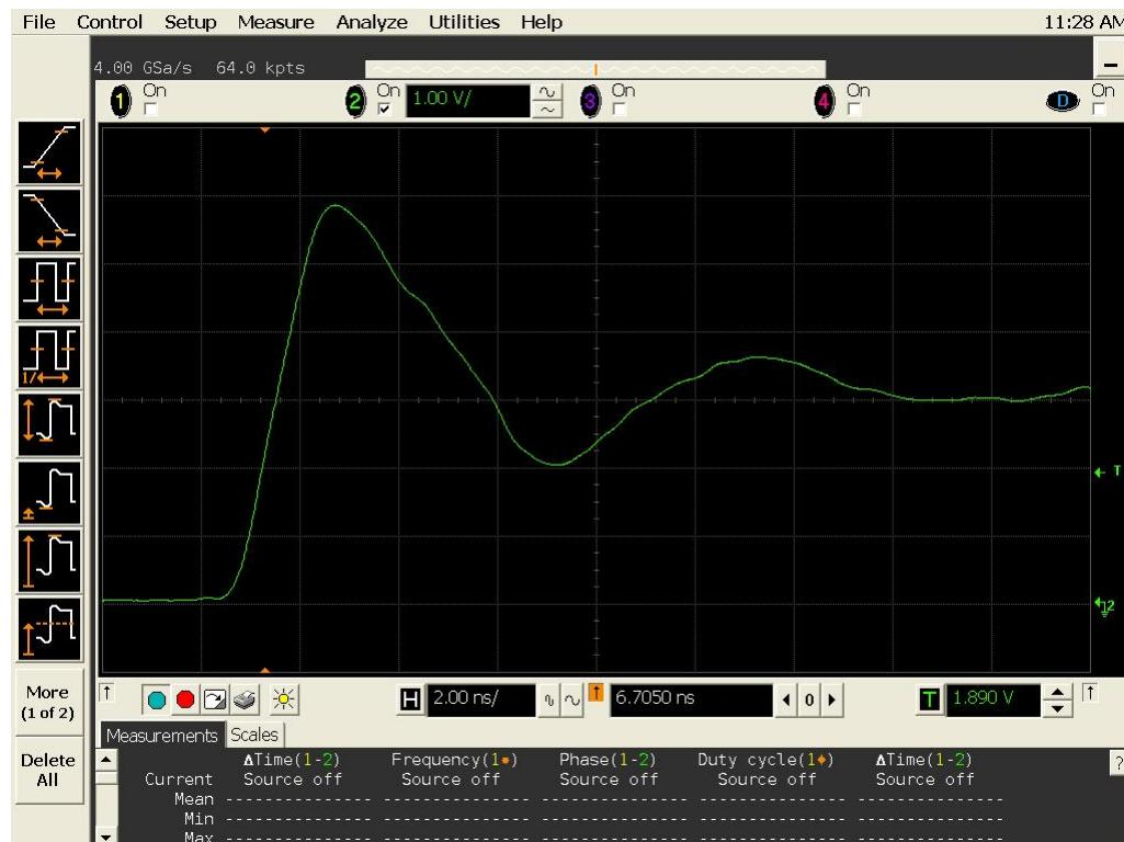
Figure 12b DUT 5800 Post-Annealing Rising Edge
