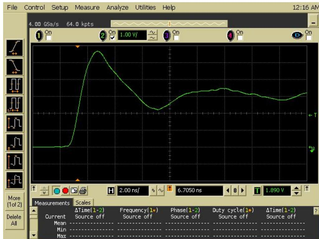
Figure 14a DUT 5835 Pre-Irradiation Rising Edge
