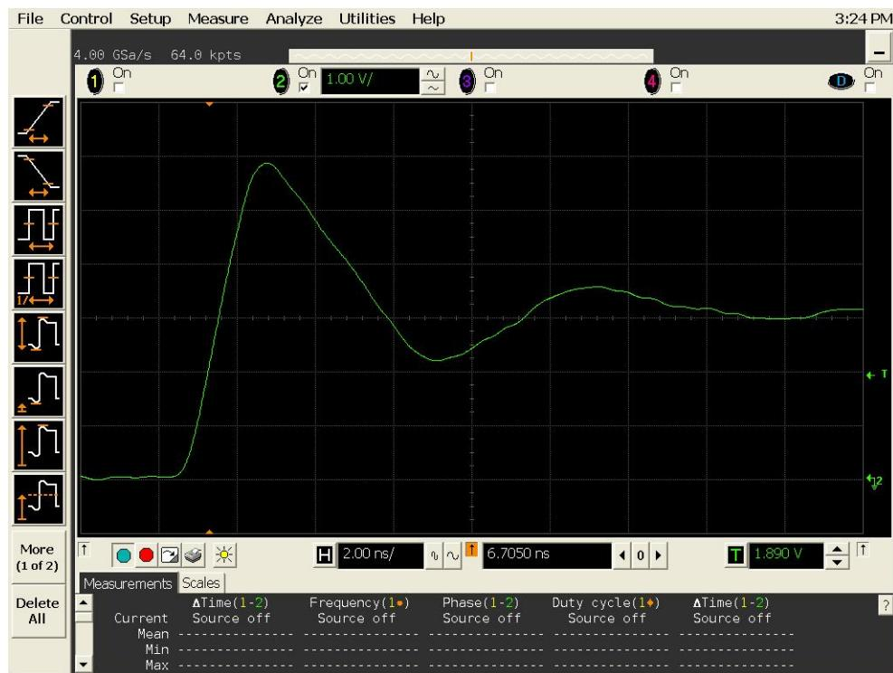
Figure 9b DUT 5782 Post-Annealing Rising Edge
