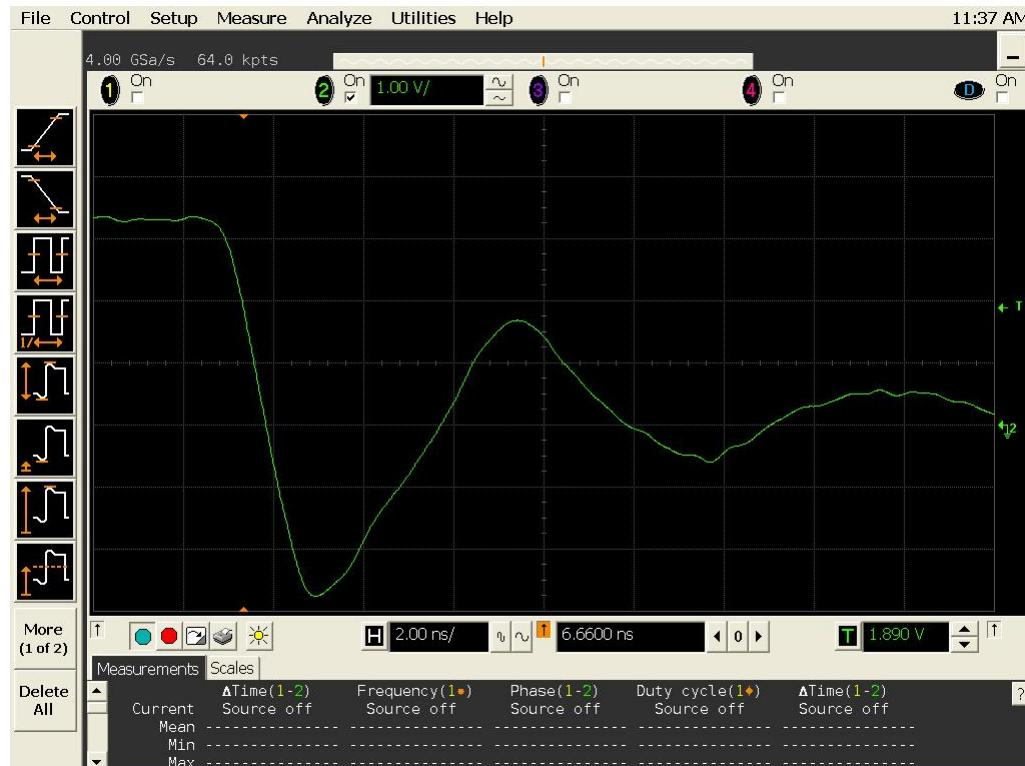
Figure 20b DUT 5835 Post-Annealing Falling Edge
