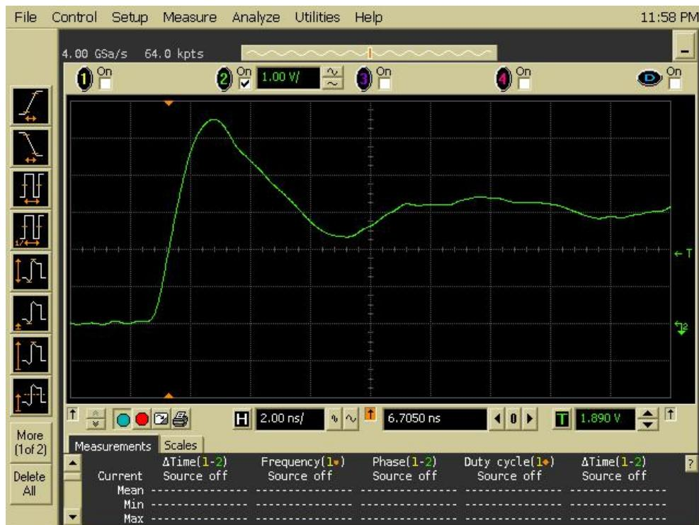
Figure 9a DUT 5782 Pre-Irradiation Rising Edge
