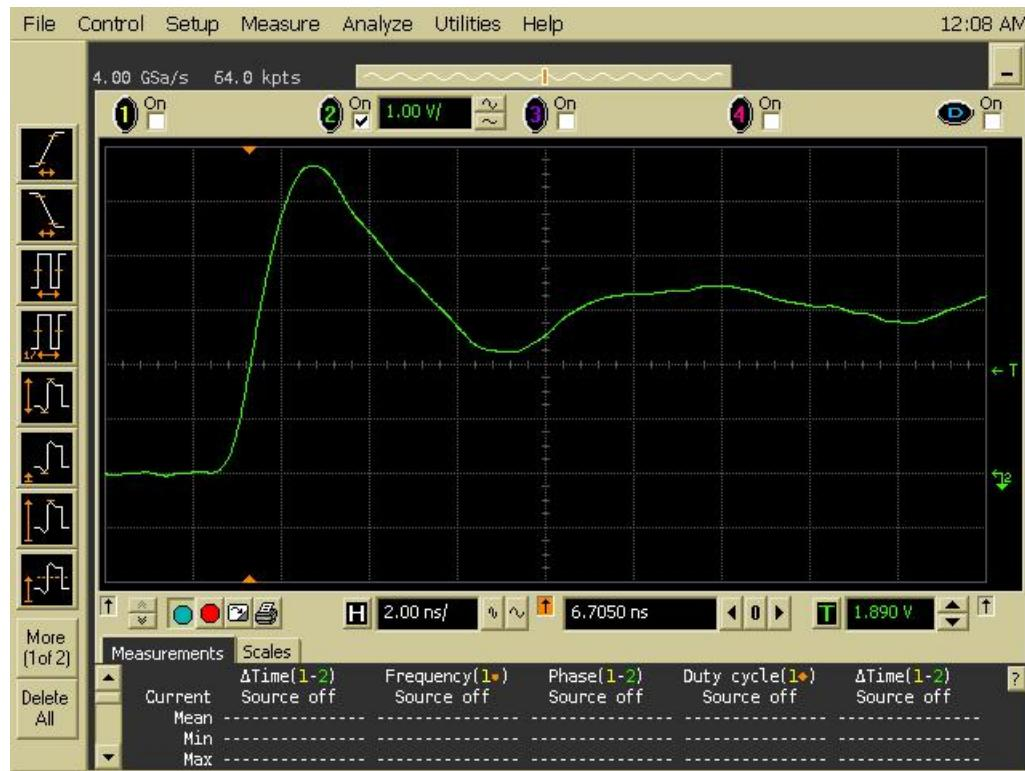
Figure 10a DUT 5785 Pre-Irradiation Rising Edge
