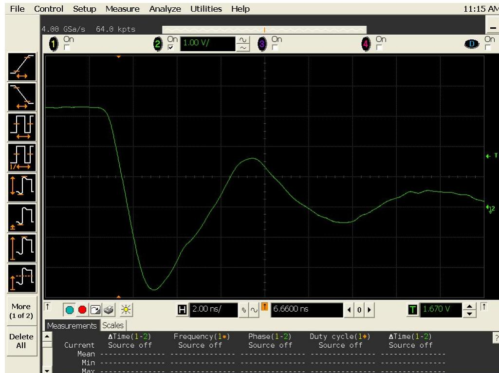
Figure 16b DUT 5785 Post-Annealing Falling Edge
