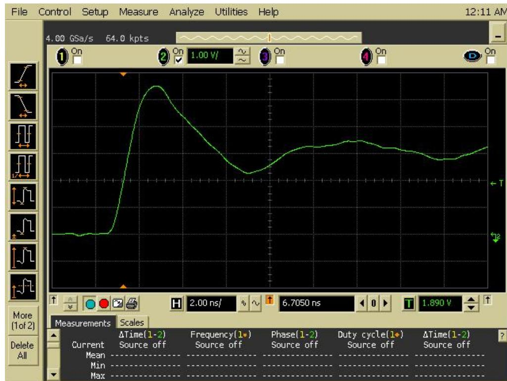
Figure 12a DUT 5800 Pre-Irradiation Rising Edge
