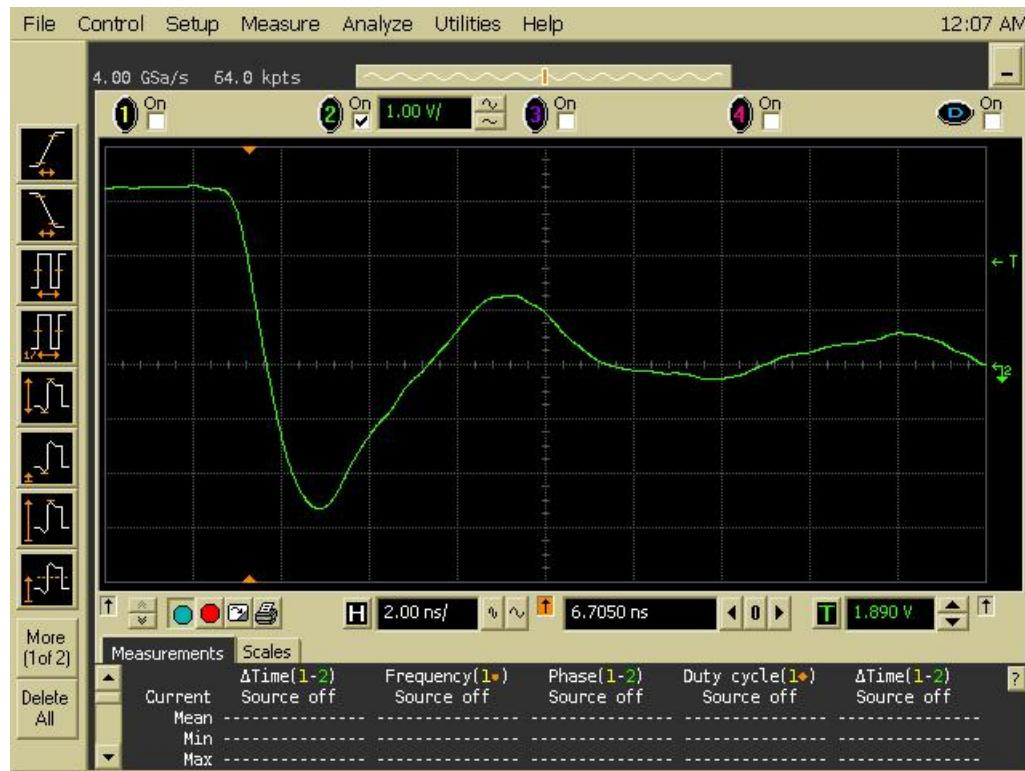
Figure 16a DUT 5785 Pre-Irradiation Falling Edge
