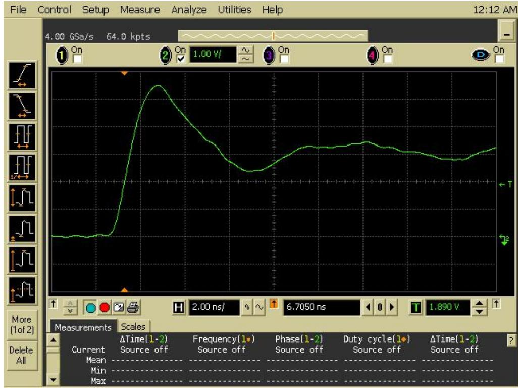
Figure 13a DUT 5814 Pre-Irradiation Rising Edge
