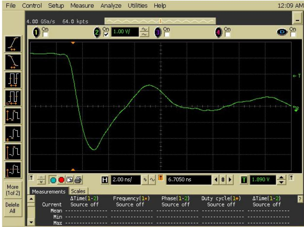
Figure 17a DUT 5797 Pre-Irradiation Falling Edge
