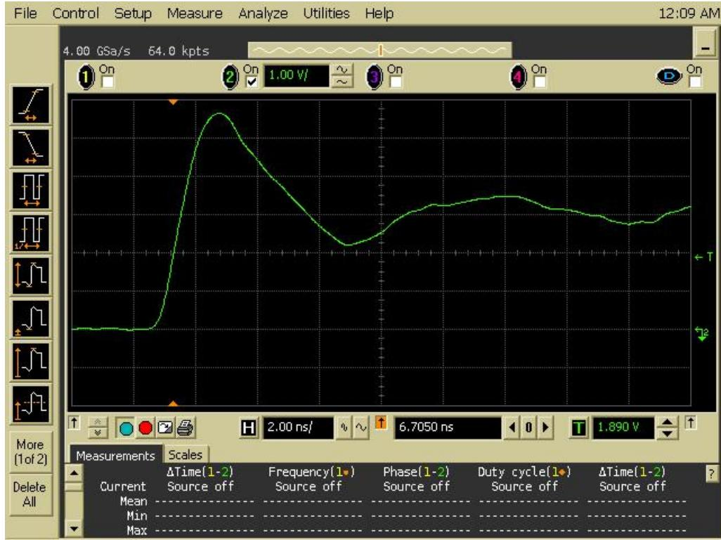
Figure 11a DUT 5797 Pre-Radiation Rising Edge
