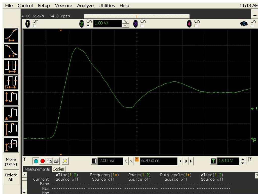
Figure 10b DUT 5785 Post-Annealing Rising Edge
