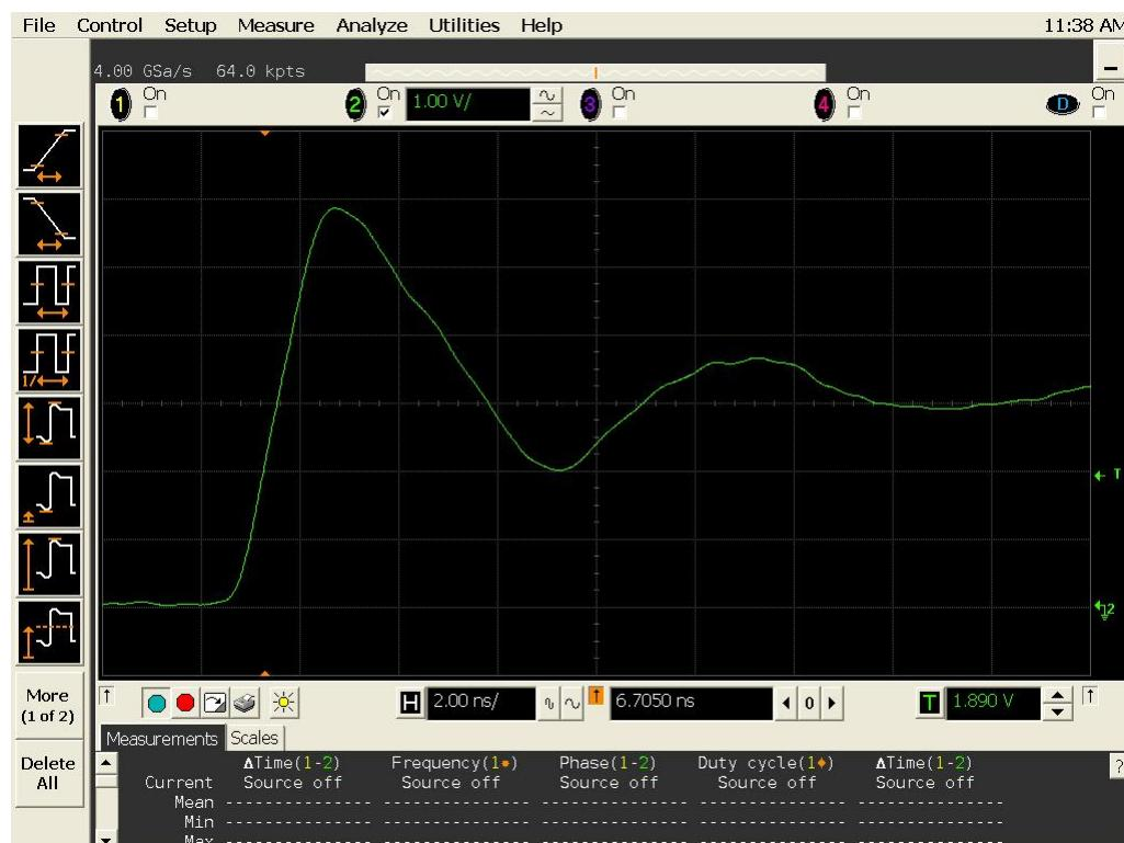
Figure 14b DUT 5835 Post-Annealing Rising Edge
