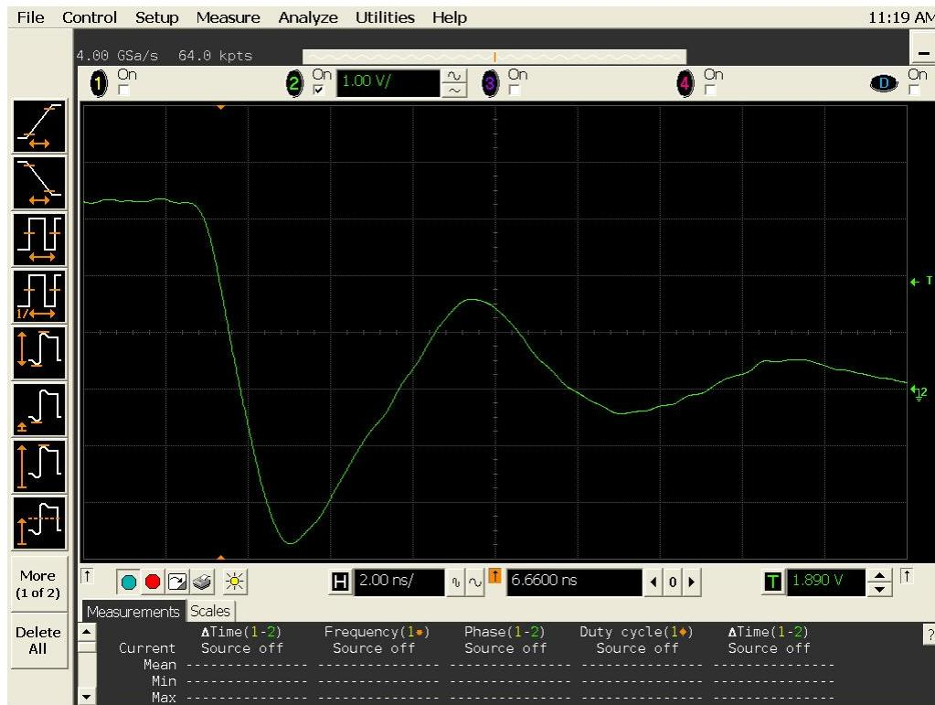
Figure 20a DUT 5356 Pre-Irradiation Falling Edge
