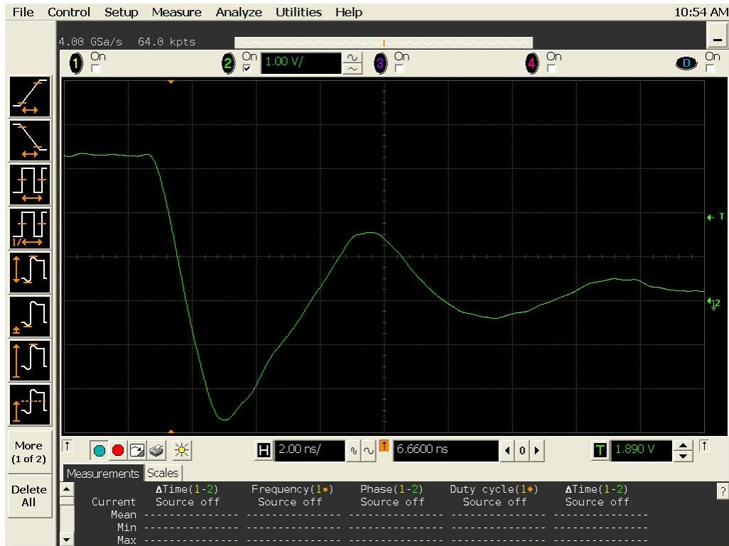
Figure 15a DUT 5318 Pre-Radiation Falling Edge
