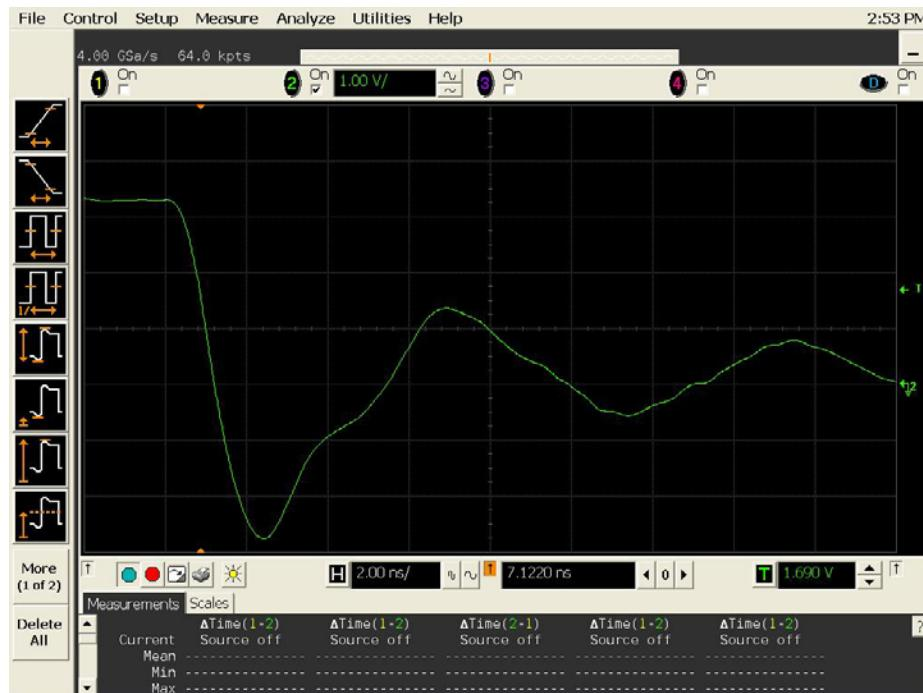
Figure 18b DUT 3542 Post-Annealing Falling Edge
