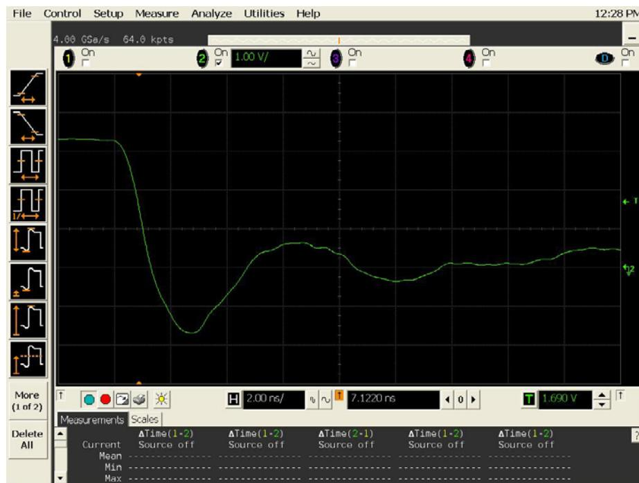
Figure 20a DUT 3557 Pre-Irradiation Falling Edge
