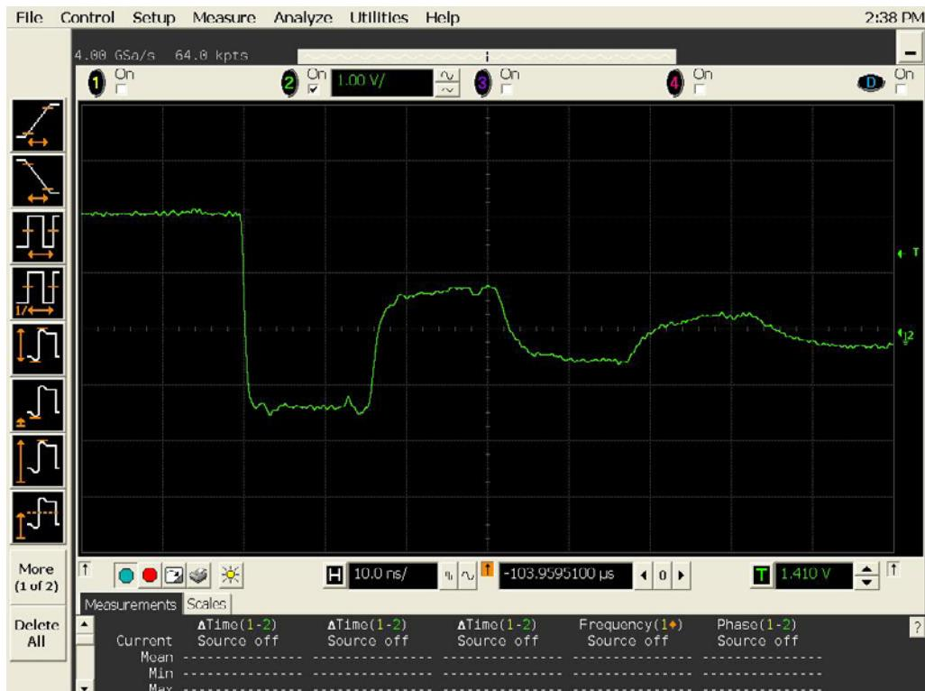
Figure 17b DUT 7972 Post-Annealing Falling Edge,
