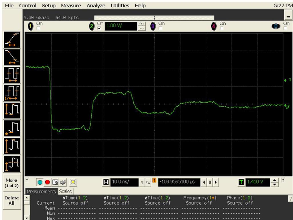
Figure 17a DUT 7972 Pre-Irradiation Falling Edge,
