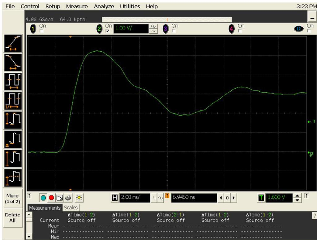
Figure 14(a) DUT 9765 pre-irradiation rising edge.
