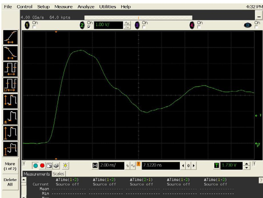
Figure 9(b) DUT 9693 post-annealing rising edge. Notice the time scale is different from pre-irradiation.
