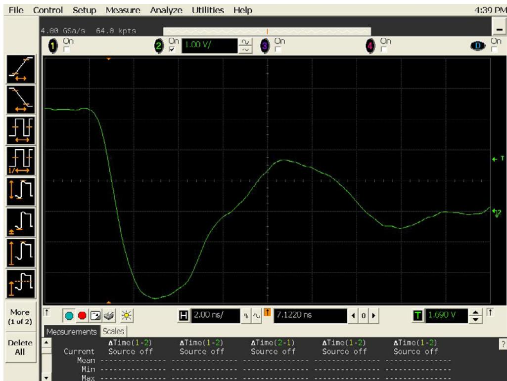
Figure 17(b) DUT 9745 post-annealing falling edge.
