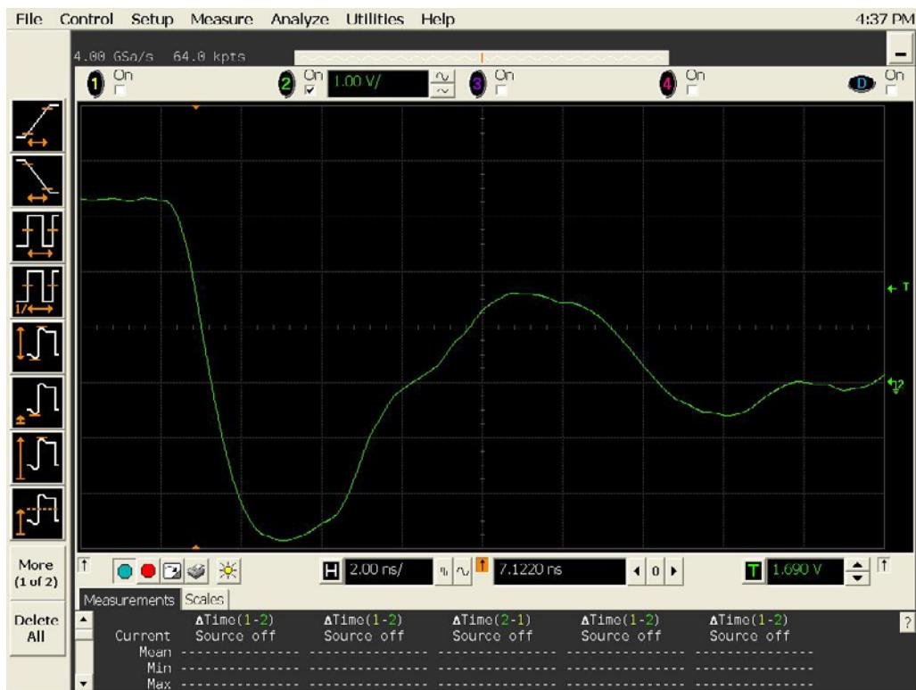
Figure 16(b) DUT 9709 post-annealing falling edge.
