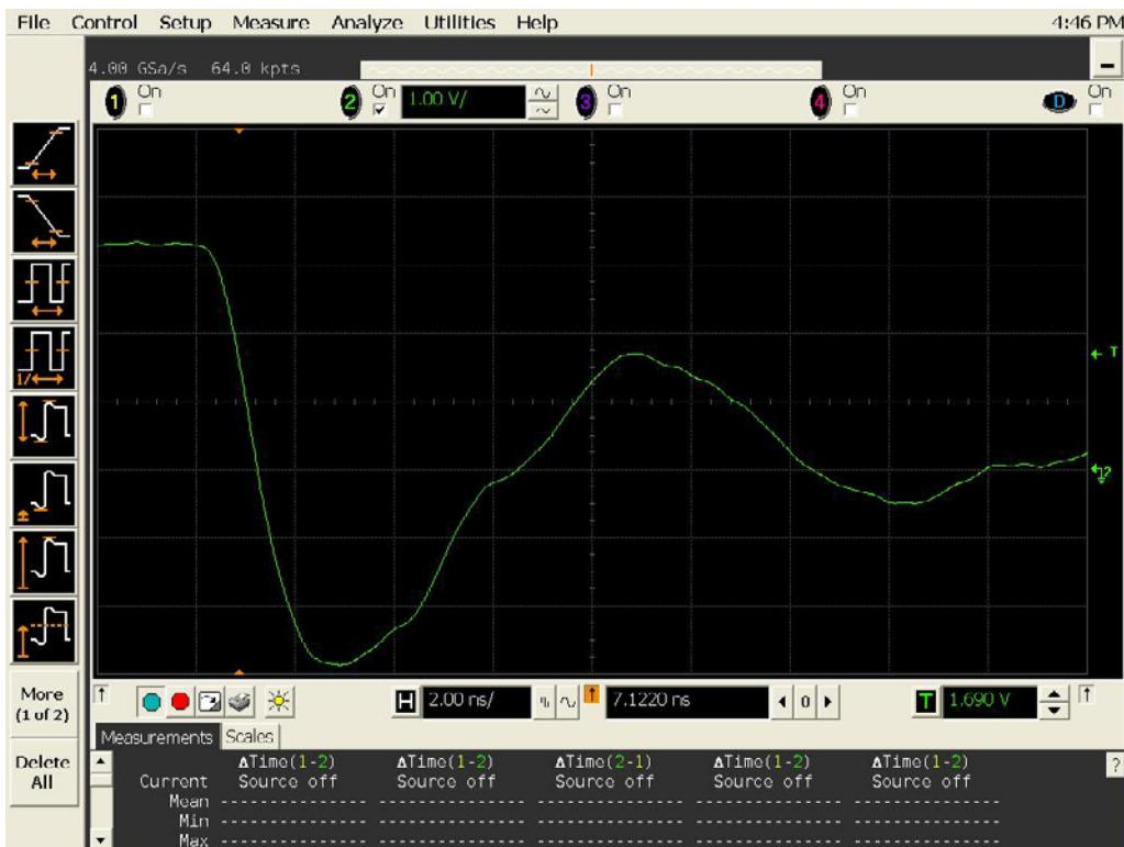
Figure 19(b) DUT 9757 post-annealing falling edge.
