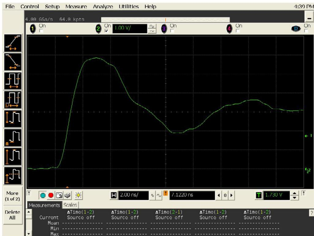
Figure 11(b) DUT 9745 post-annealing rising edge.
