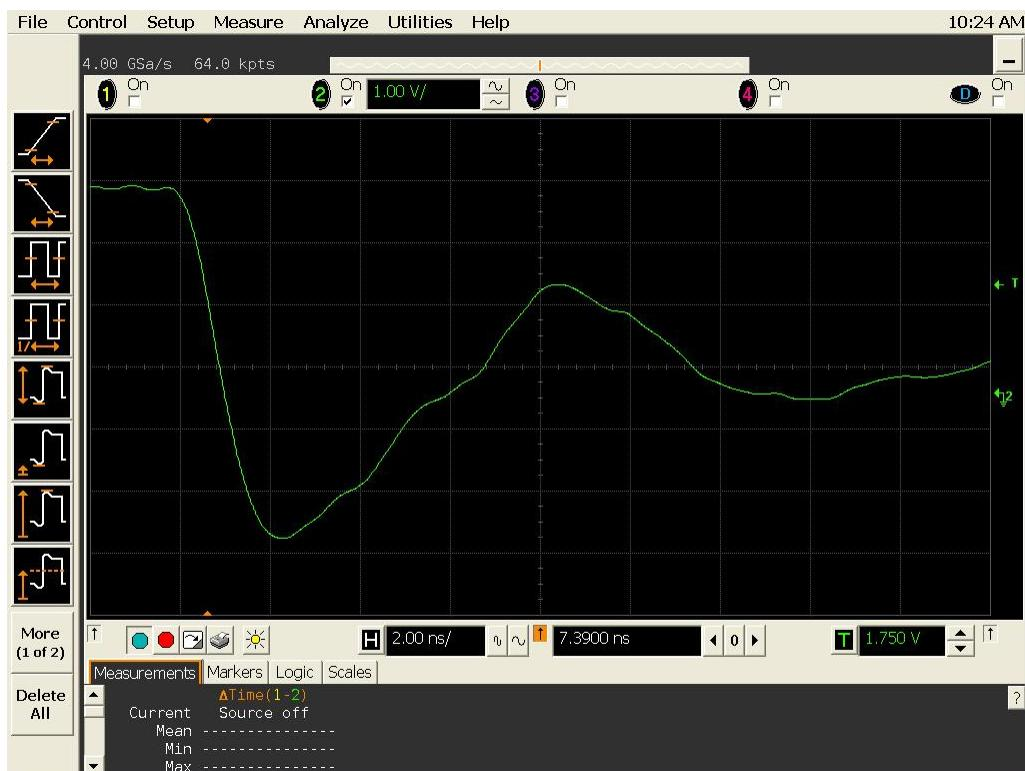
Figure 16(b) DUT 5866 post-annealing falling edge.
