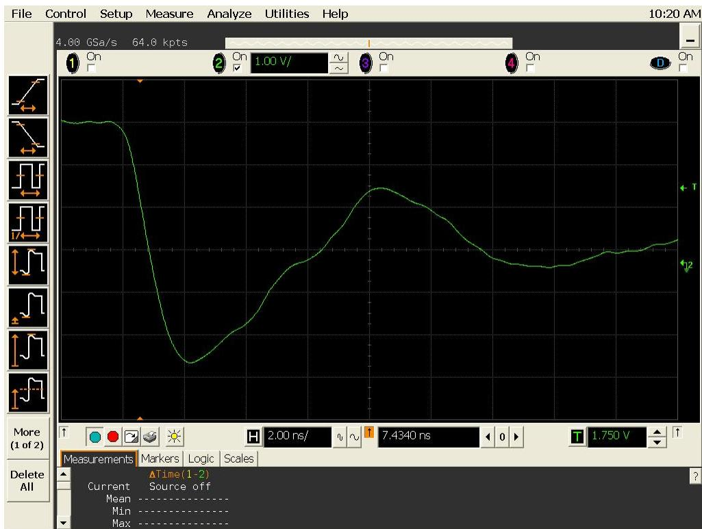
Figure 15(a) DUT 5746 pre-irradiation falling edge.
