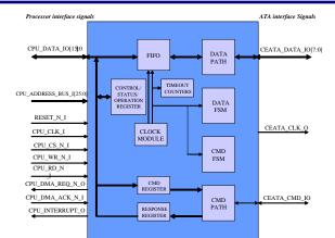
The block diagram, left, shows the modules built into the ProASIC3 chip where the CE-ATA controller logic is implemented. It also shows the interface signals between the processor and the FPGA.
