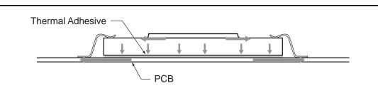
Figure 2-2 • Heat Flow in a Vacuum
