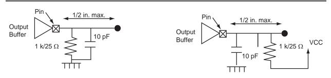
Figure 2-10 • 3.3 V PCI Output Loading
