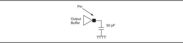
Figure 2-8 • 5 V PCI Output Loading
