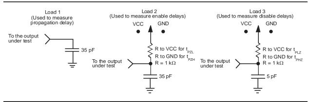
Figure 2-6 • AC Test Loads
