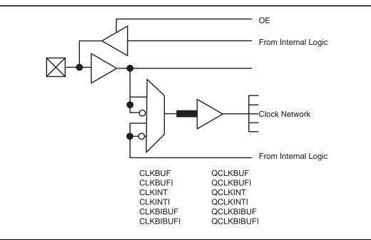
Figure 2-21 • Routed and Quadrant Clock Buffers in RTSX72SU
