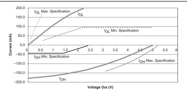
Figure 2-7 • 5 V PCI V/I Curve for RTSX-SU
