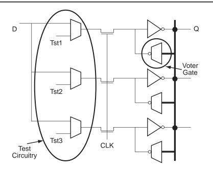
Figure 2-16 • R-Cell Implementation – Test Circuitry
