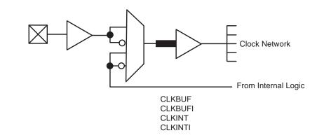
*Figure 2-20* • Routed Clock Buffers in RTSX32SU
