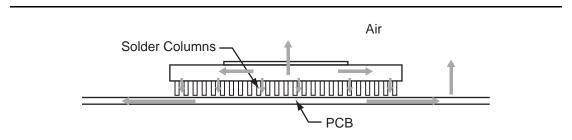
Figure 2-1 • Hear Flow when Air is Present
