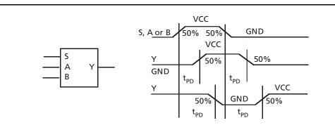
Figure 2-12 • C-Cell Timing Model and Waveforms
