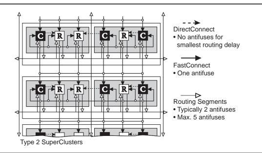
Figure 1-4 • DirectConnect and FastConnect for SuperCluster 2's
