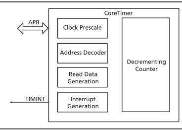
Figure 1 • CoreTimer Block Diagram
