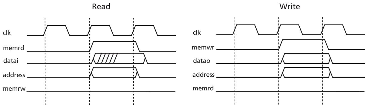
Figure 6 • Actel Core8051 XDATA Read and Write Operation
