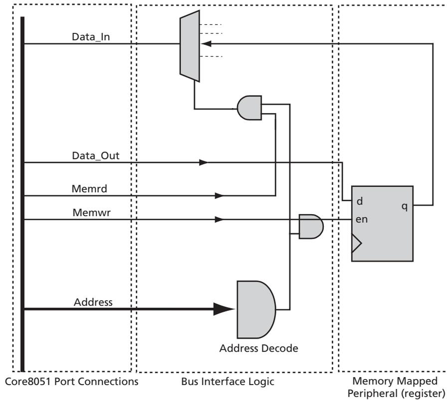
Figure 5 • Typical Actel Core8051 Custom Logic Implementation
