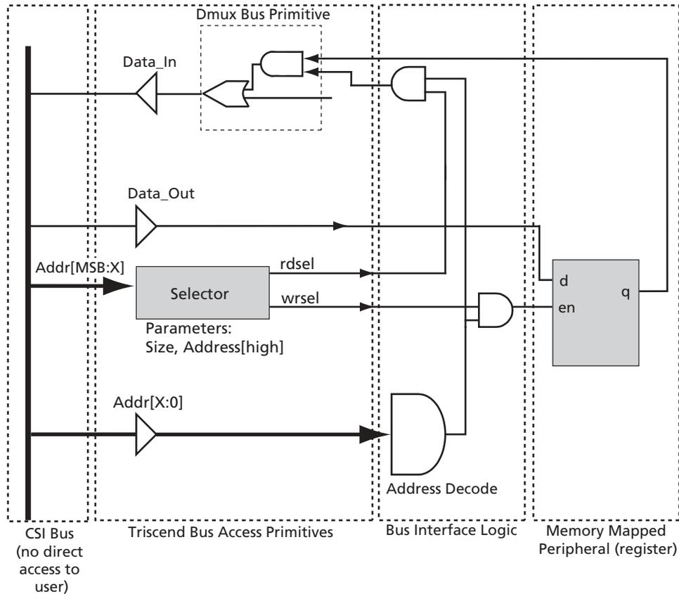
Figure 3 • Typical Triscend TE5 Custom Logic Implementation
