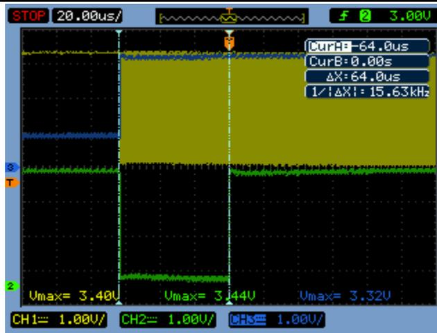
**Figure 2 • Pulse Generated Due to Reset from the POR or PPR Circuit**
