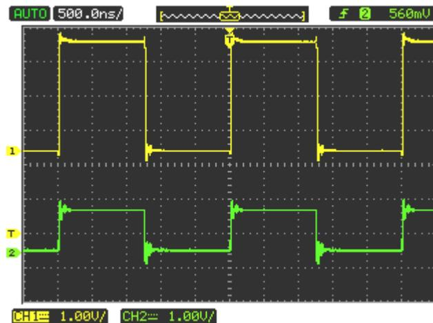
Figure 3 • Voltage Translation from 1.2 V to 3.3 V
