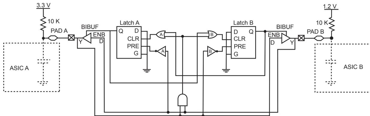
Figure 2 • Bidirectional Level Shifter Circuit Diagram
