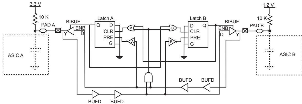
Figure 4 • Bidirectional Level Shifter with Input Path Delay
