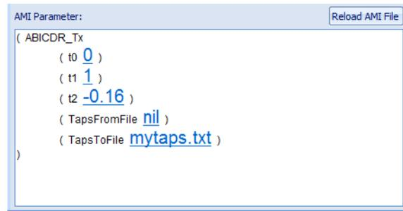
Transceiver contains 3-tap FFE filter settings, which are used to modify the transmitter waveform. A tap is a point at which the weighting is applied to each cursor. 3-tap equalization applies energy at the bit before and the bit after the main bit. The taps are named as t0, t1 and t2.
