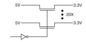
Figure 2 • IDTQS32X2384 Bus Switch
