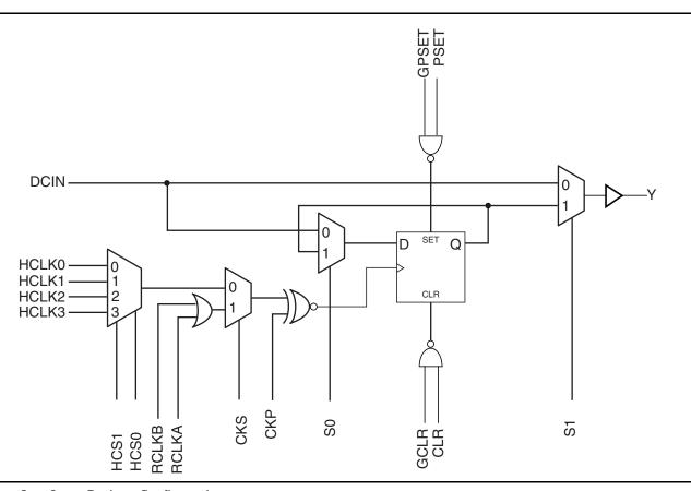
Figure 8 • Input Register Configuration
