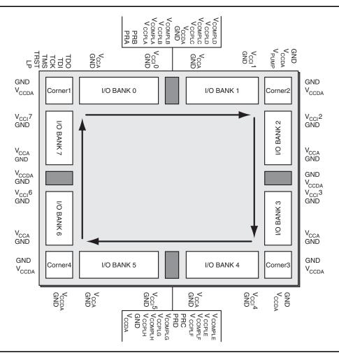
Figure 10 • I/O Layout Plan
