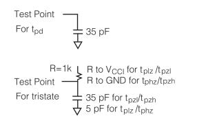
Figure 3 • Test Circuit for LVTTL and LVCMOS
