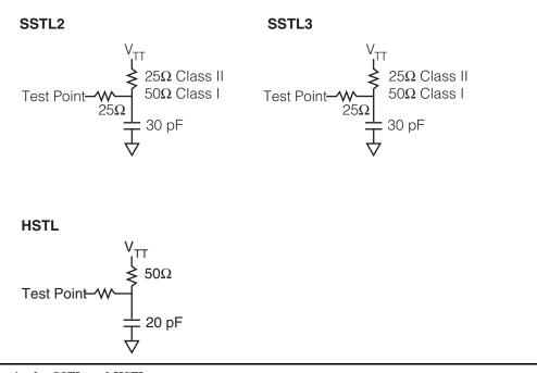
Figure 4 • Test Circuits for SSTL and HSTL
