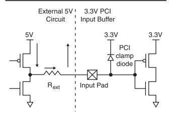
Figure 1 • 5V Tolerance with 3.3V PCI
