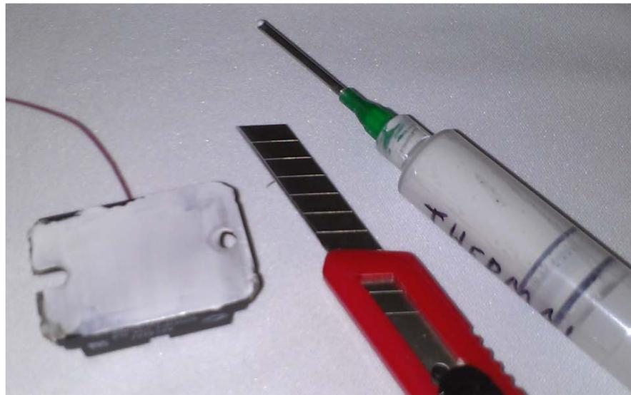
**Figure 2 · Example of applying thermal grease onto the base plate of SOT-227.**
