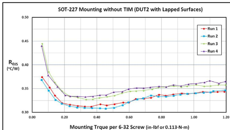
**Figure 9 - Thermal resistance vs. mounting torque without TIM and treated surfaces.**
