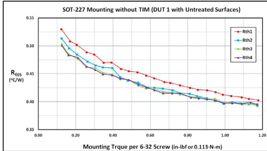
**Figure 8 - Thermal resistance vs. mounting torque without TIM and untreated surfaces.**
