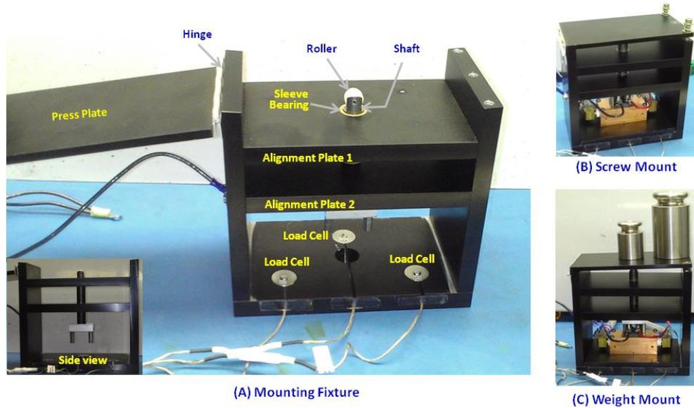
Figure 6 · Test fixture for thermal resistance vs. mounting pressure measurement: (A) Mounting fixture assembly, (B) Mounting force controlled by screws, and (C) Mounting force controlled by weights.
