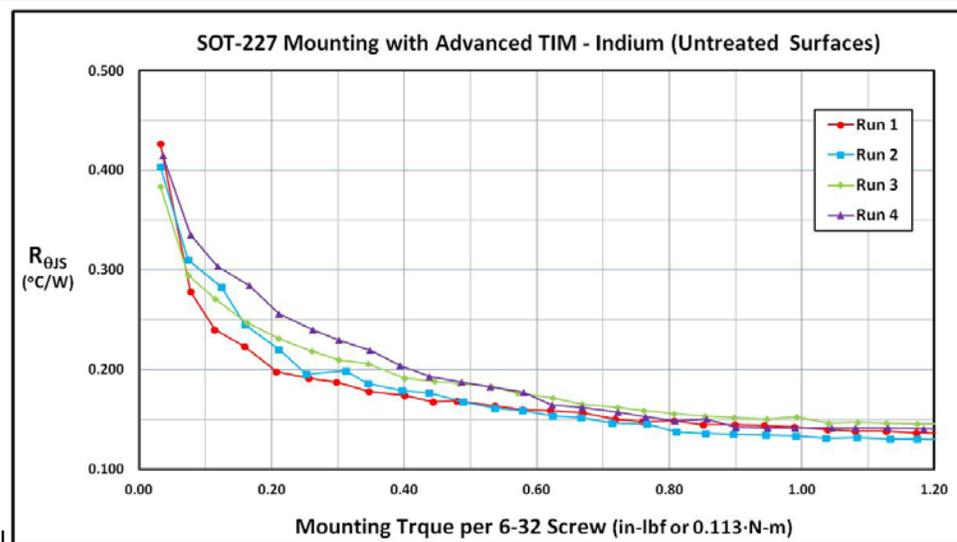
Figure 5 - Thermal resistance vs. mounting torque with advanced TIM - Indium and untreated surfaces.
