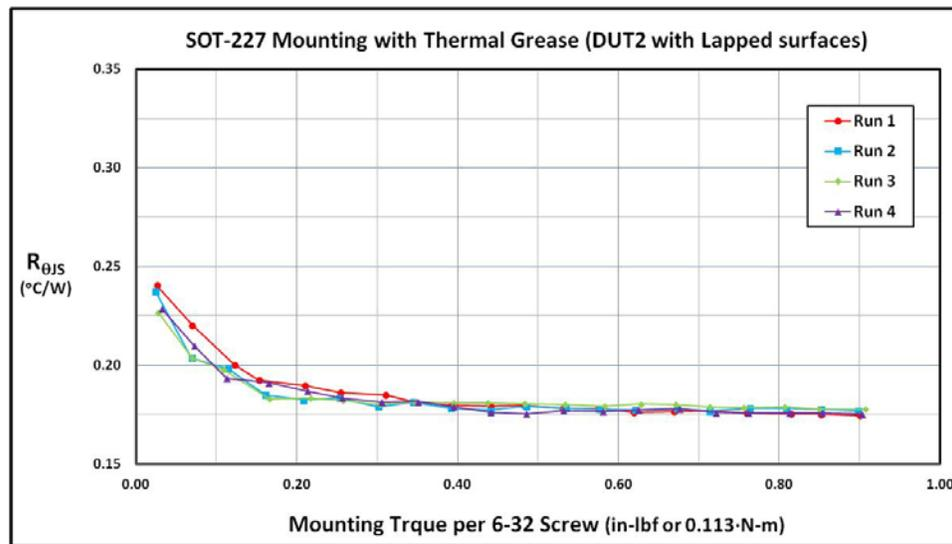
Figure 4 · Thermal resistance vs. mounting torque with Thermal Grease TIM and treated surfaces (DUT 2).
