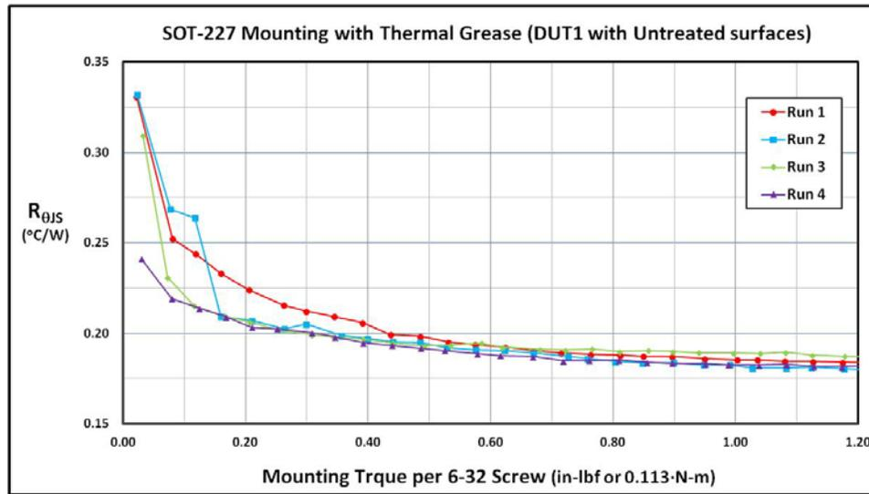
Figure 3 · Thermal resistance vs. mounting torque with Thermal Grease TIM and untreated surfaces (DUT 1).
