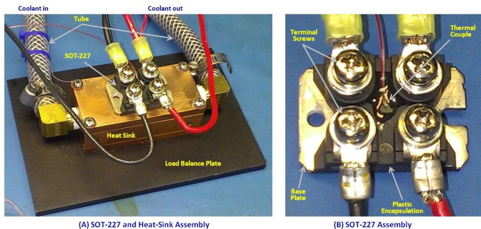
Figure 7 · Heat sink and SOT-227 assemblies of the thermal resistance vs. mounting pressure measurement.
