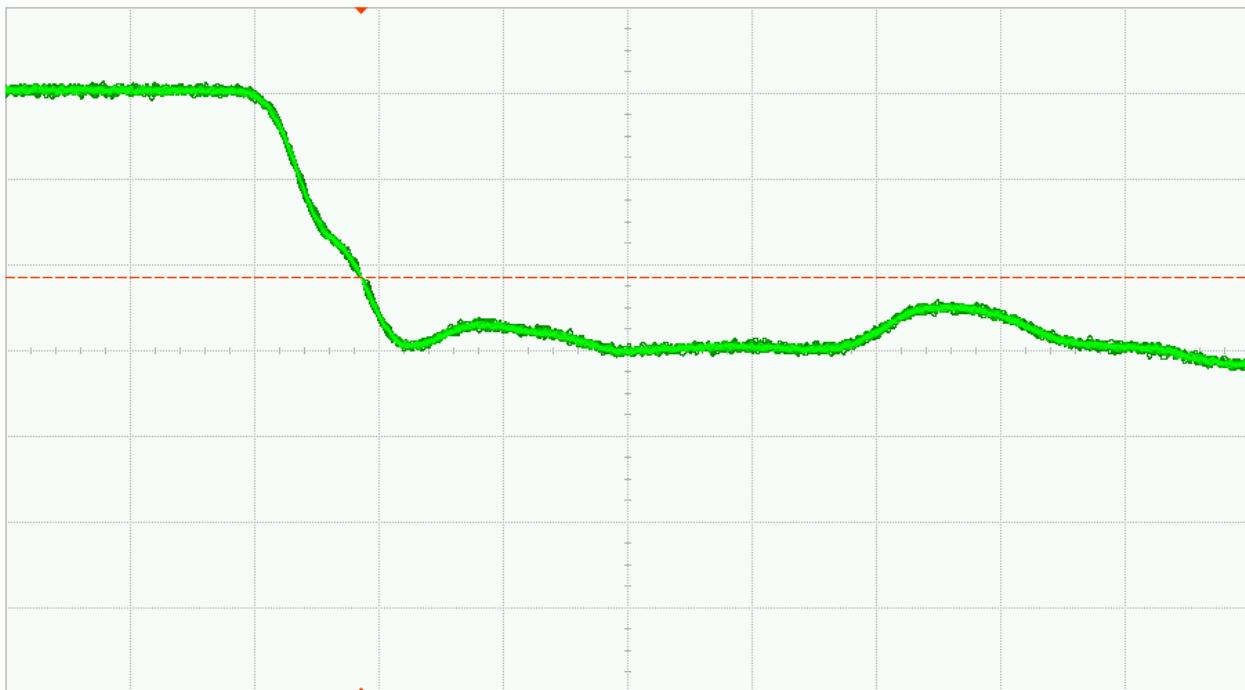
Fig. 34 (b). DUT 07596 post-annealing falling edge, abscissa scale is 1V/div and ordinate scale is 2ns/div
