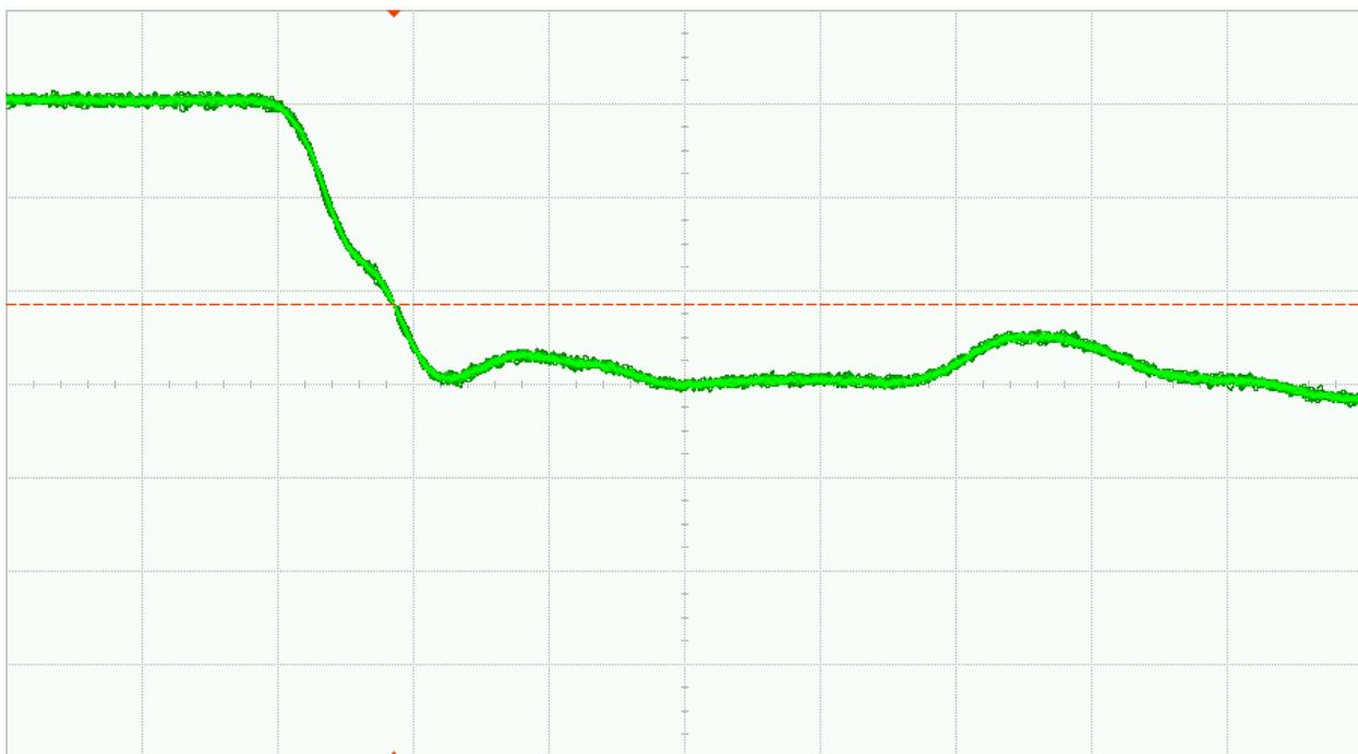
Fig. 33 (b). DUT 07585 post-annealing falling edge, abscissa scale is 1V/div and ordinate scale is 2ns/div
