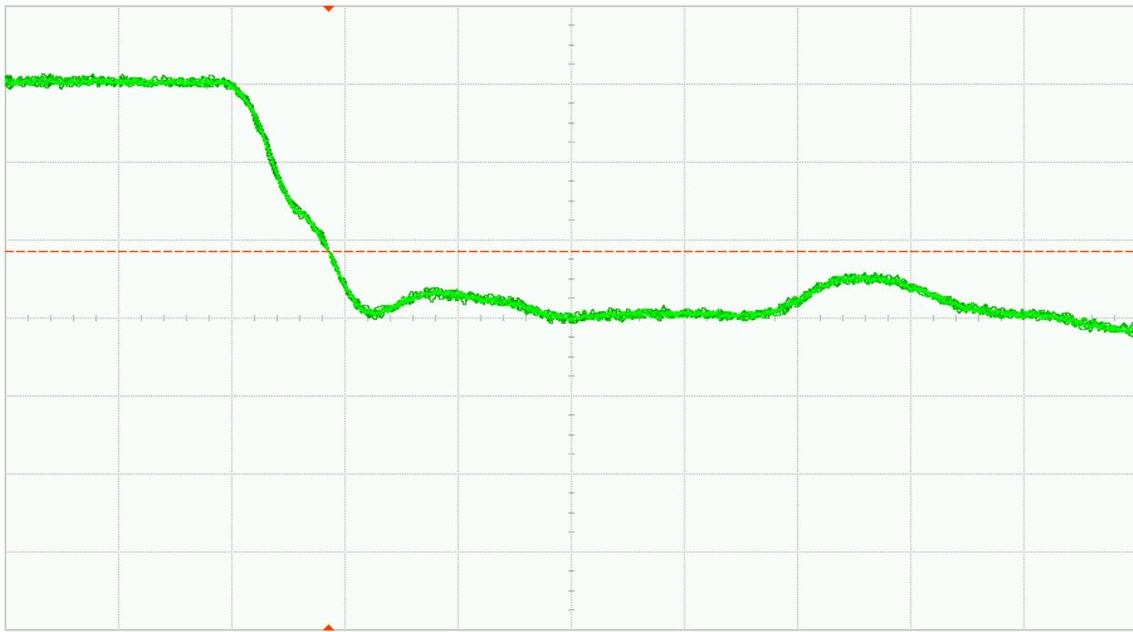
Fig. 37 (a). DUT 07640 pre-irradiation falling edge, abscissa scale is 1V/div and ordinate scale is 2ns/div
