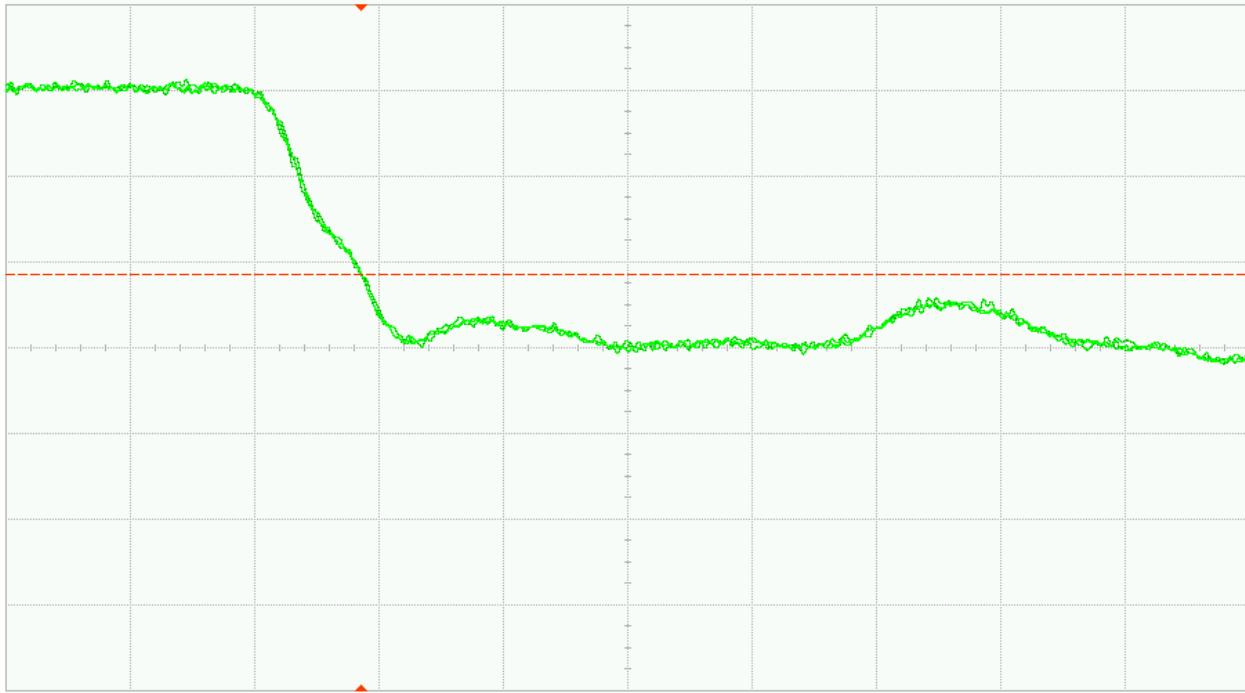
Fig. 35 (a). DUT 07617 pre-irradiation falling edge, abscissa scale is 1V/div and ordinate scale is 2ns/div
