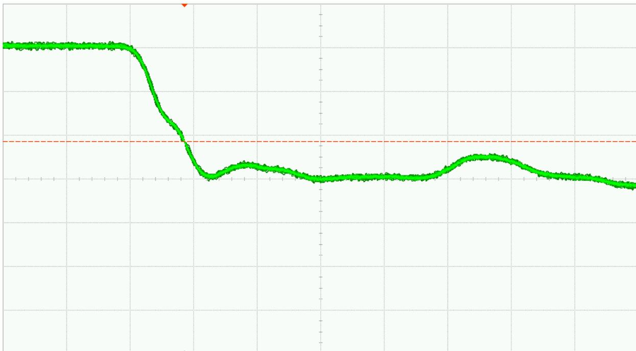
Fig. 35 (b). DUT 07617 post-annealing falling edge, abscissa scale is 1V/div and ordinate scale is 2ns/div
