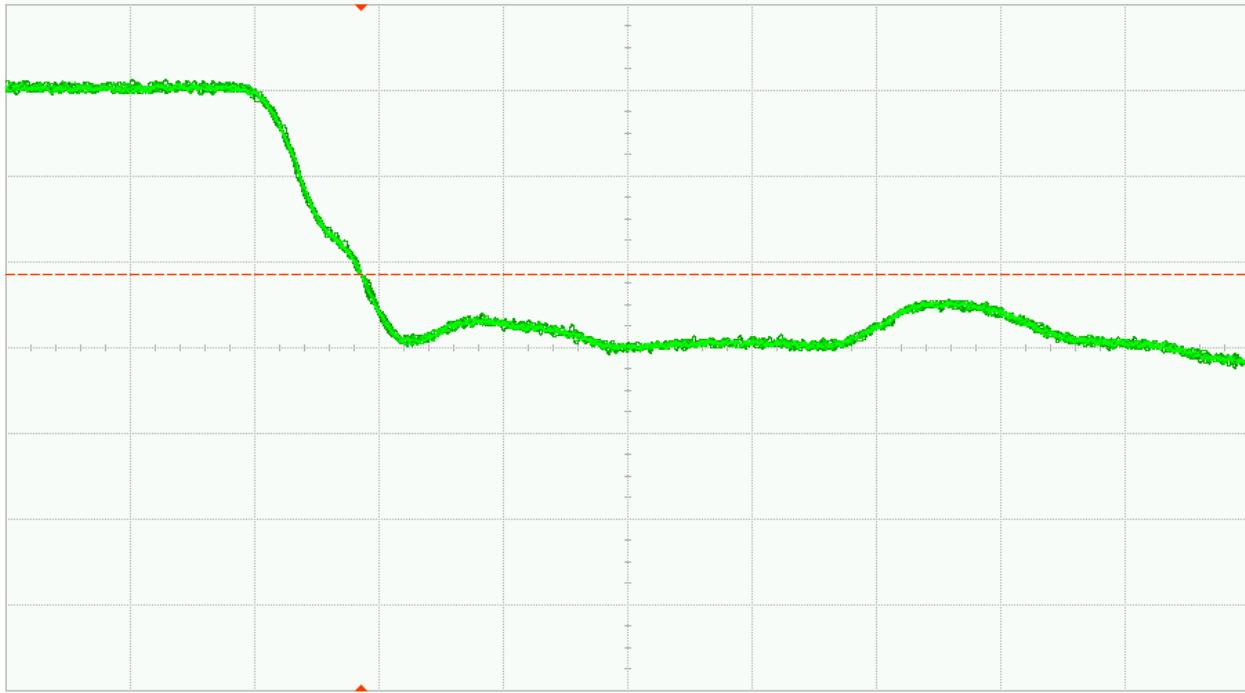
Fig. 32 (a). DUT 07573 pre-irradiation falling edge, abscissa scale is 1V/div and ordinate scale is 2ns/div
