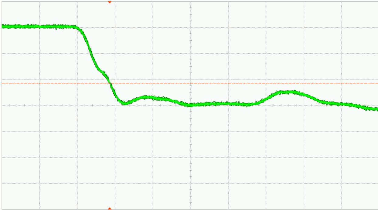
Fig. 36 (a). DUT 07622 pre-irradiation falling edge, abscissa scale is 1V/div and ordinate scale is 2ns/div
