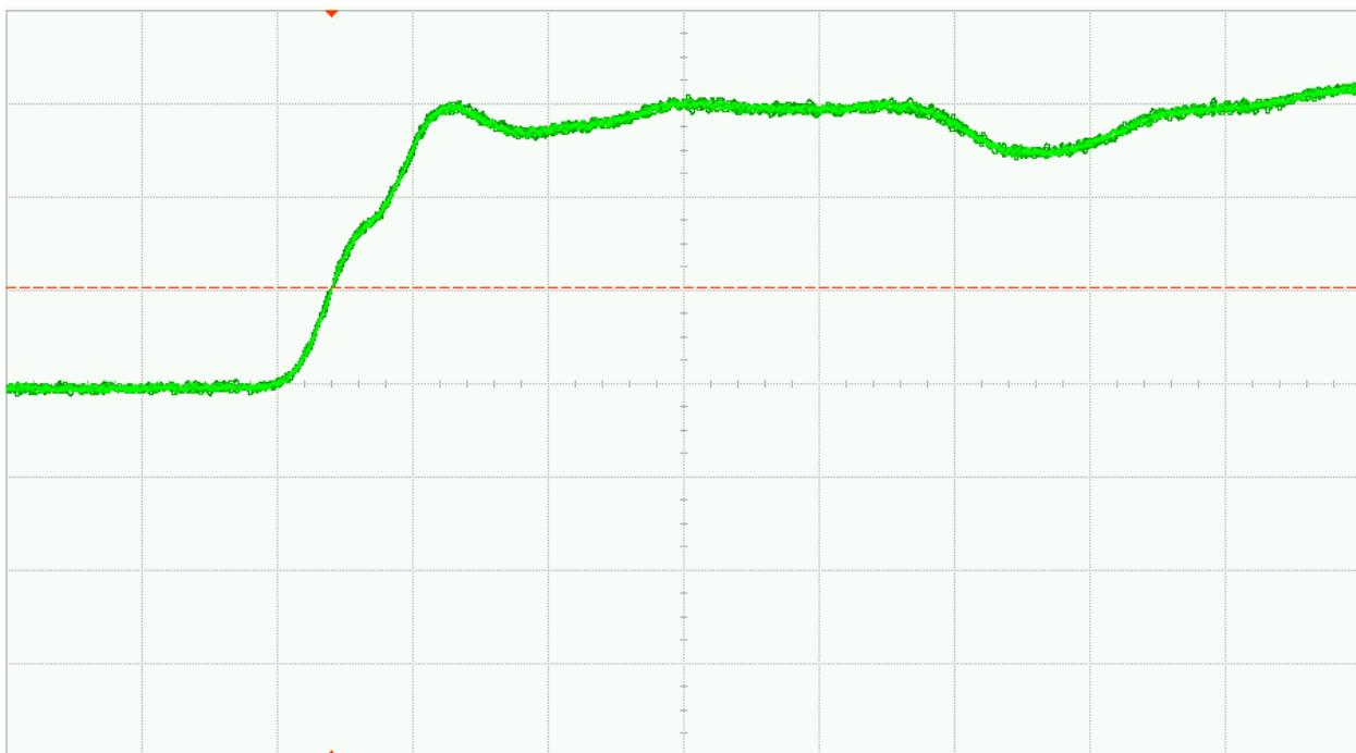
Fig. 29 (b). DUT 07617 post-annealing rising edge, abscissa scale is 1V/div and ordinate scale is 2ns/div
