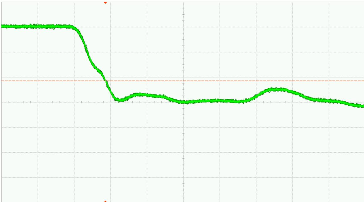
Fig. 35 (a). DUT 06829 pre-irradiation falling edge, abscissa scale is 1V/div and ordinate scale is 2ns/div
