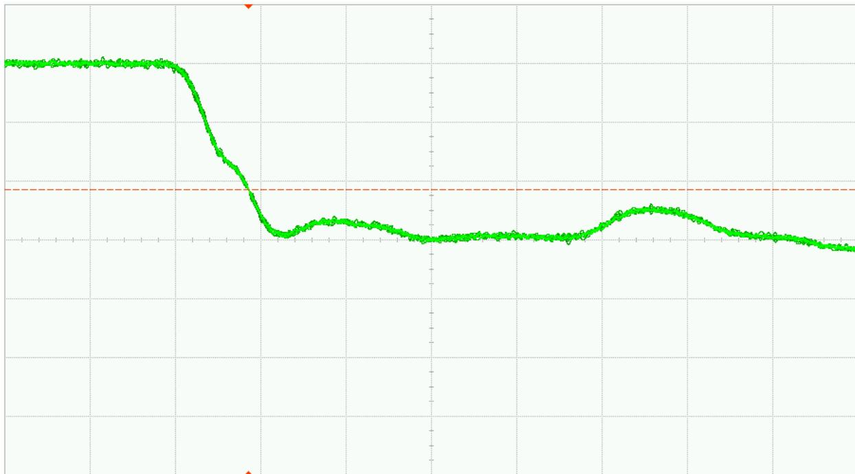
Fig. 37 (a). DUT 06917 pre-irradiation falling edge, abscissa scale is 1V/div and ordinate scale is 2ns/div
