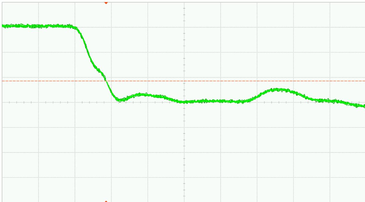
Fig. 37 (b). DUT 06917 post-annealing falling edge, abscissa scale is 1V/div and ordinate scale is 2ns/div
