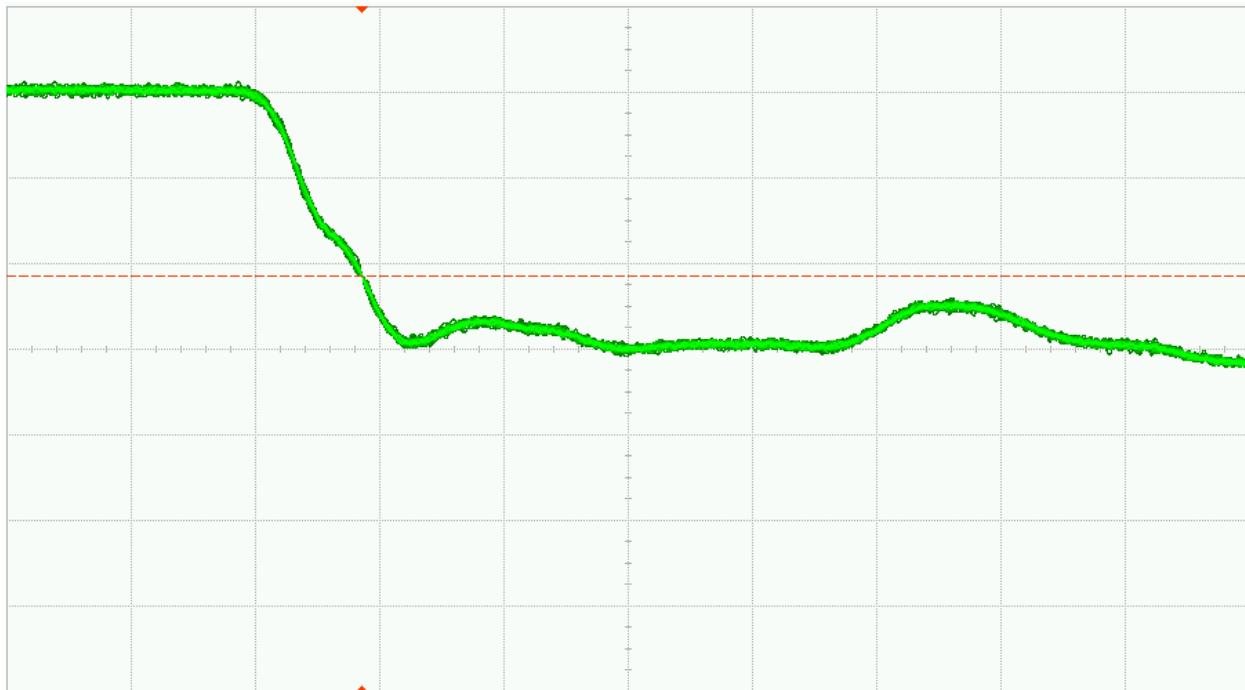
Fig. 34 (a). DUT 06828 pre-irradiation falling edge, abscissa scale is 1V/div and ordinate scale is 2ns/div
