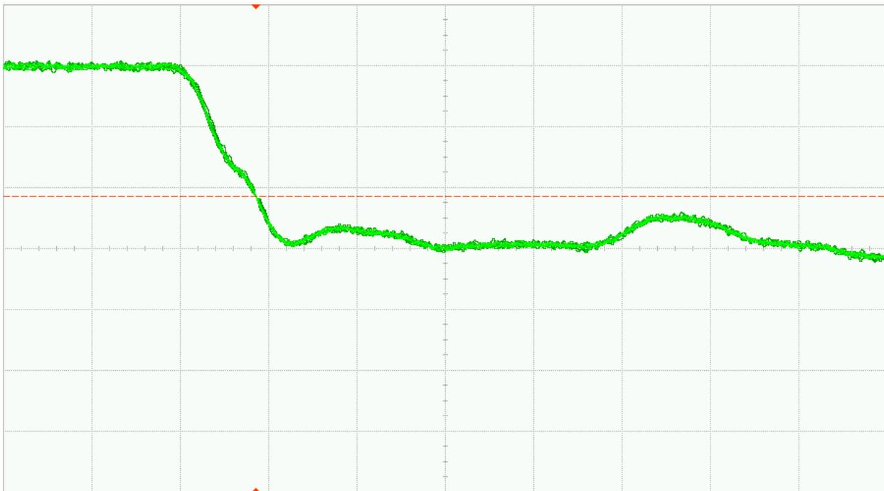
Fig. 36 (a). DUT 06877 pre-irradiation falling edge, abscissa scale is 1V/div and ordinate scale is 2ns/div
