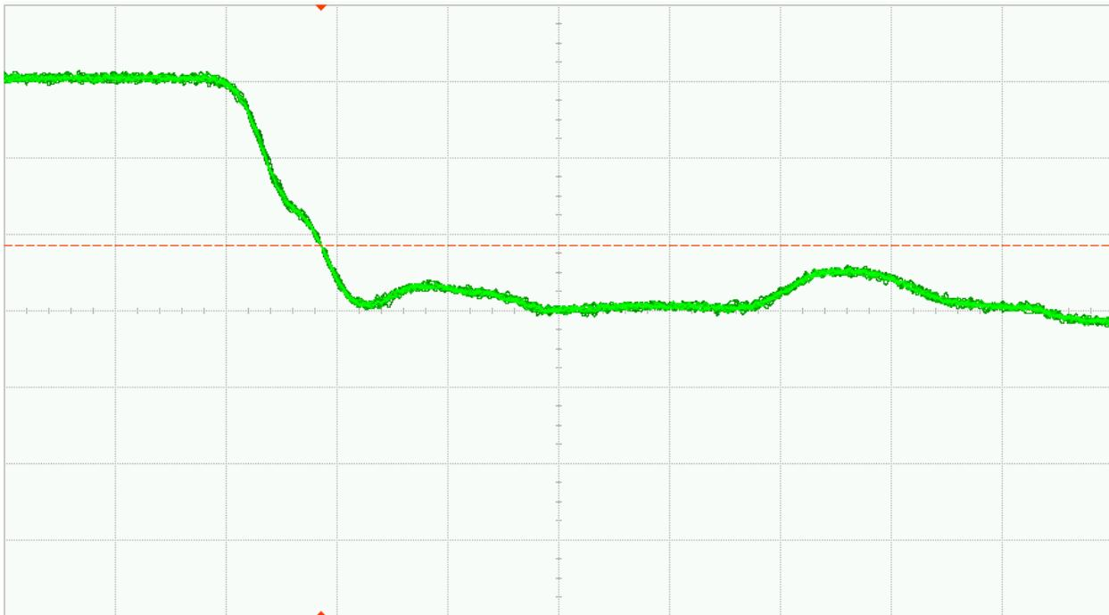
Fig. 35 (b). DUT 06829 post-annealing falling edge, abscissa scale is 1V/div and ordinate scale is 2ns/div
