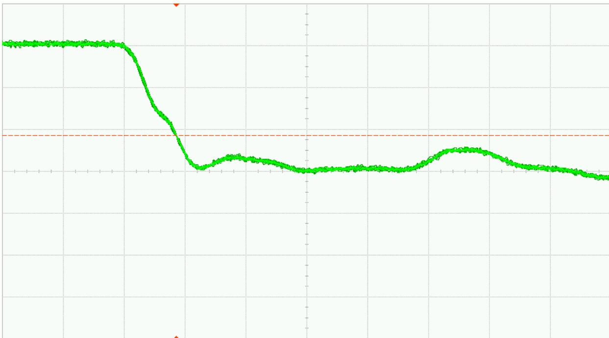
Fig. 36 (b). DUT 06877 post-annealing falling edge, abscissa scale is 1V/div and ordinate scale is 2ns/div
