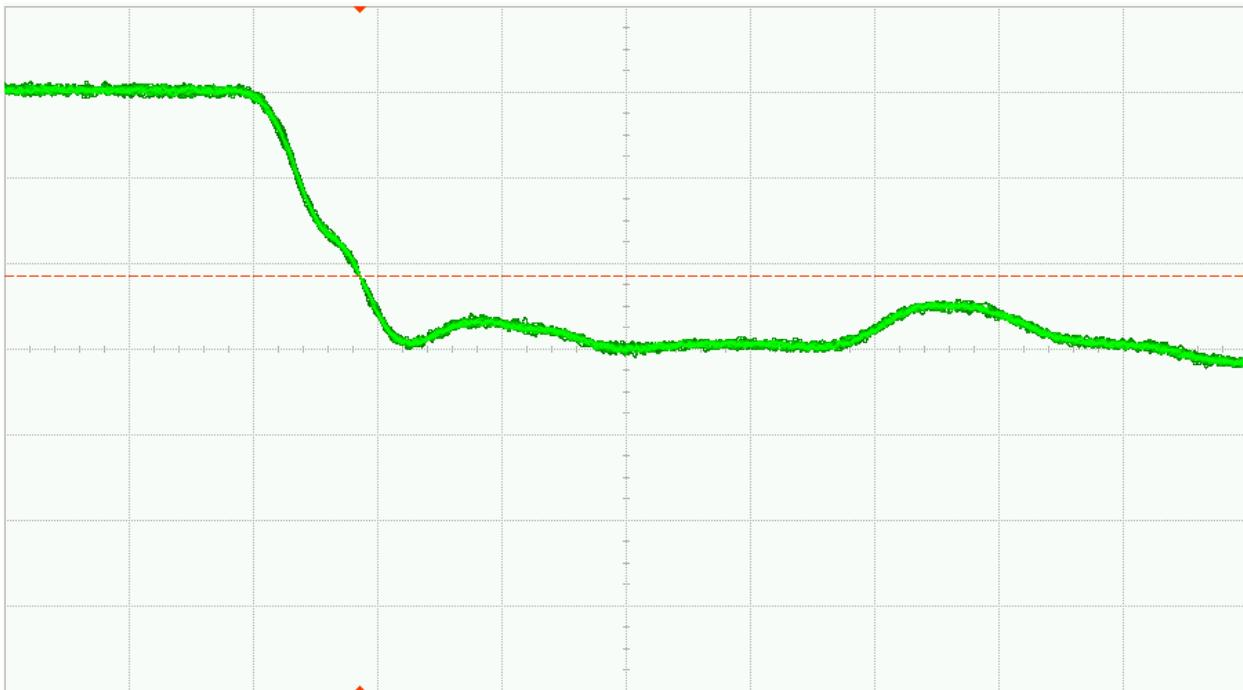
Fig. 32 (a). DUT 06787 pre-irradiation falling edge, abscissa scale is 1V/div and ordinate scale is 2ns/div
