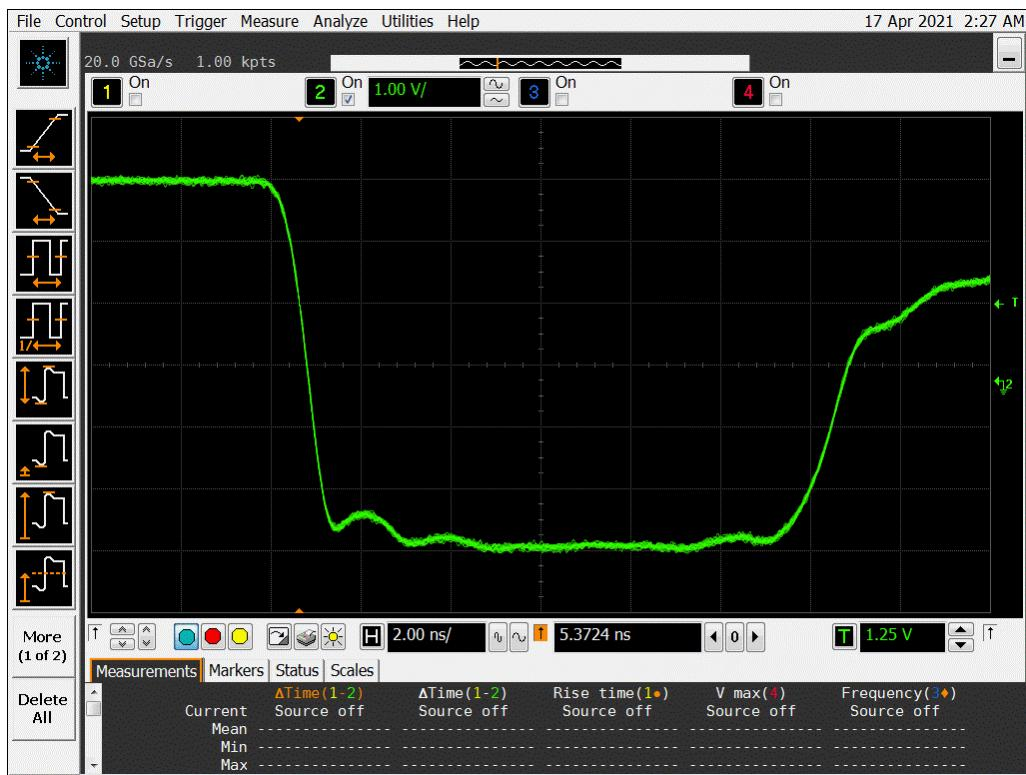
**Figure 20b DUT 439 Post-Annealing Falling Edge**
