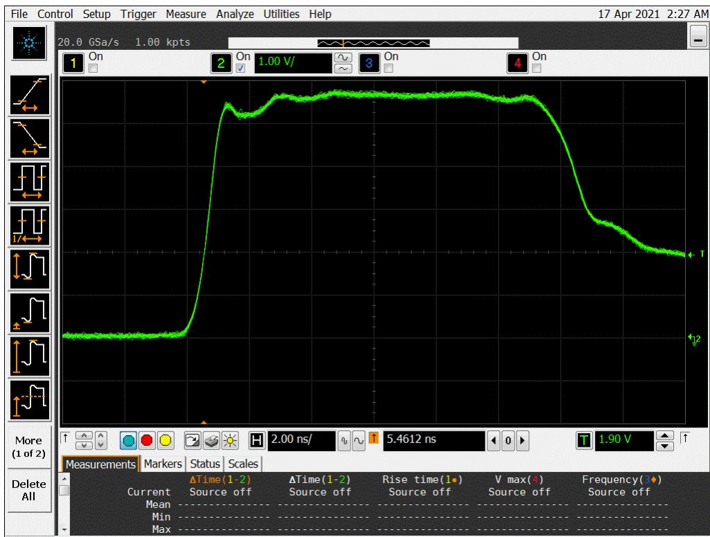
**Figure 14b DUT 439 Post-Annealing Rising Edge**
