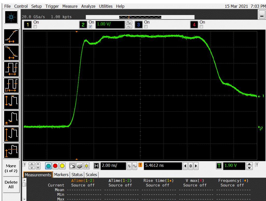
**Figure 10a DUT 507 Pre-Irradiation Rising Edge**
