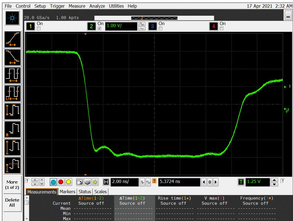
**Figure 18b DUT 490 Post-Annealing Falling Edge**
