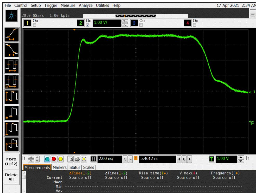
**Figure 9b DUT 505 Post-Annealing Rising Edge**
