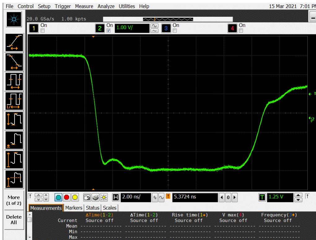
**Figure 15a DUT 505 Pre-Radiation Falling Edge**
