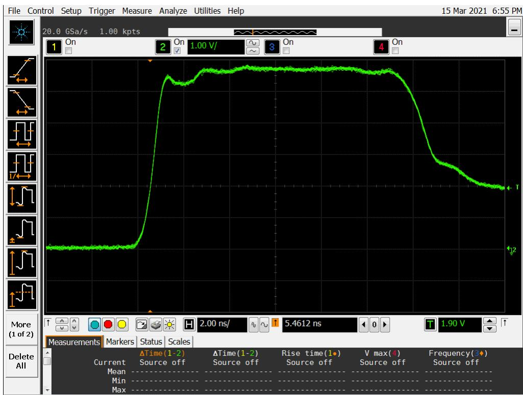
**Figure 14a DUT 439 Pre-Irradiation Rising Edge**
