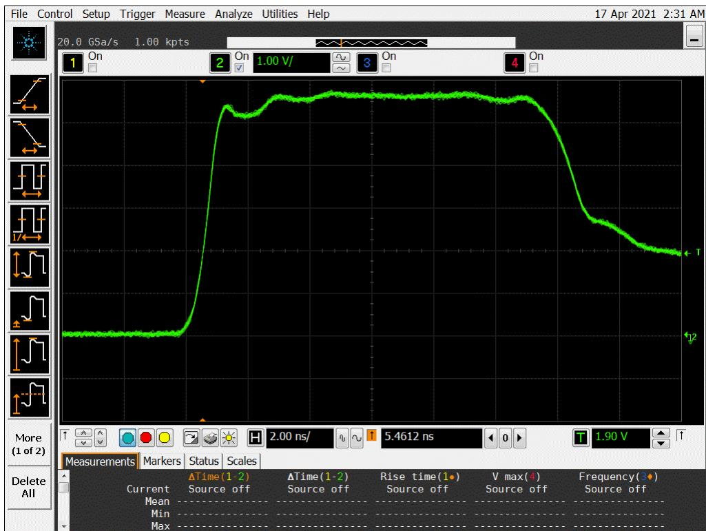
Figure 12b DUT 490 Post-Annealing Rising Edge
