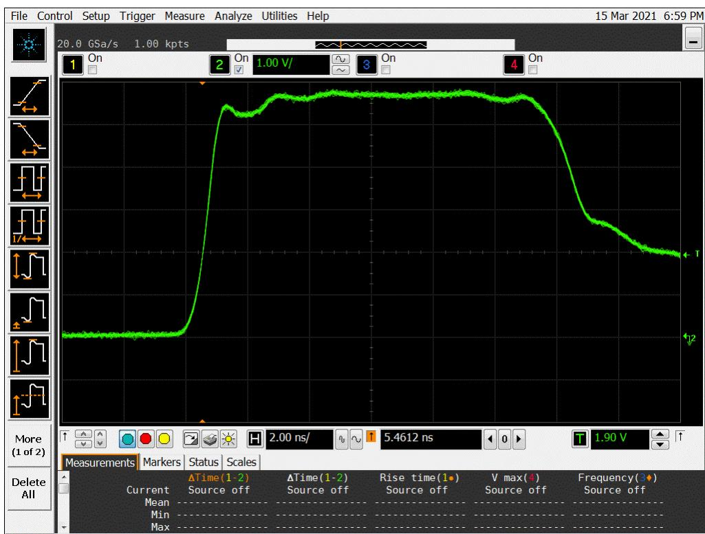
Figure 12a DUT 490 Pre-Irradiation Rising Edge
