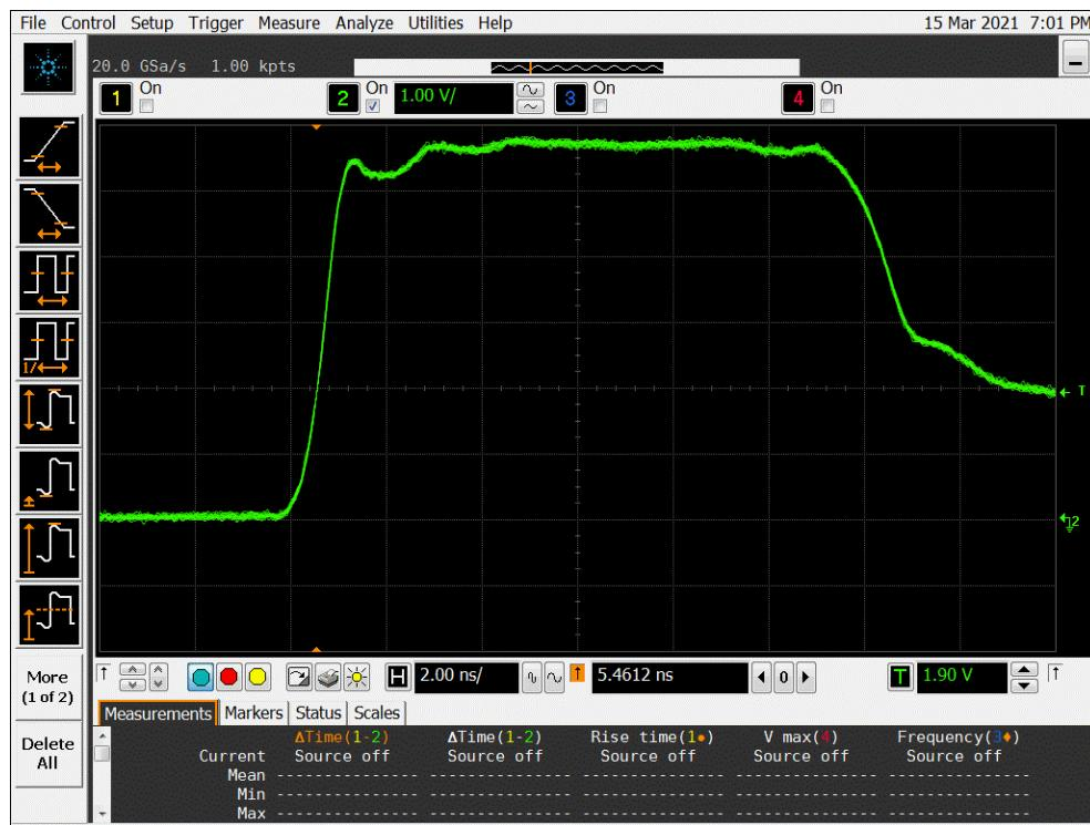
**Figure 9a DUT 505 Pre-Irradiation Rising Edge**
