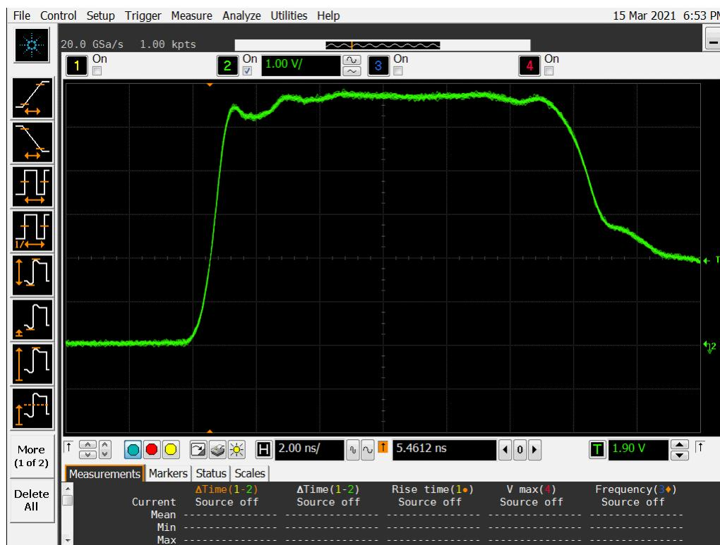
**Figure 13a DUT 394 Pre-Irradiation Rising Edge**
