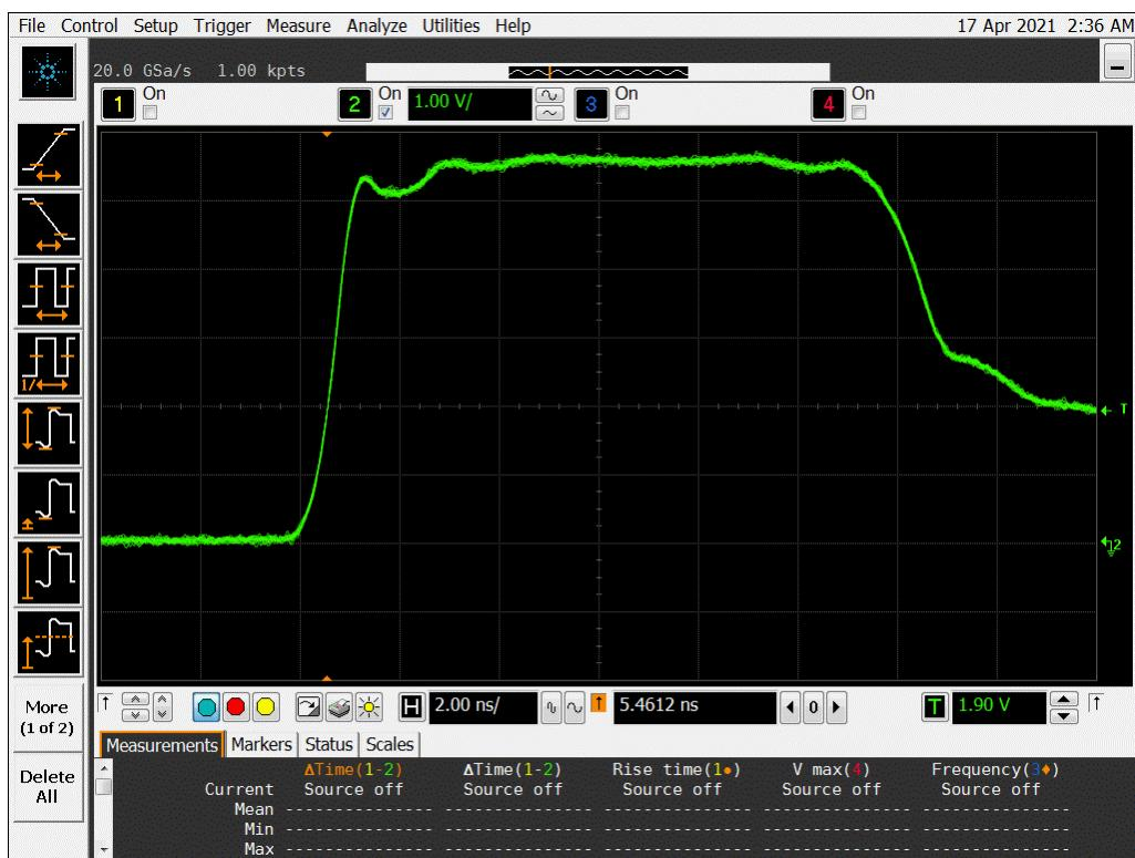
**Figure 10b DUT 507 Post-Annealing Rising Edge**
