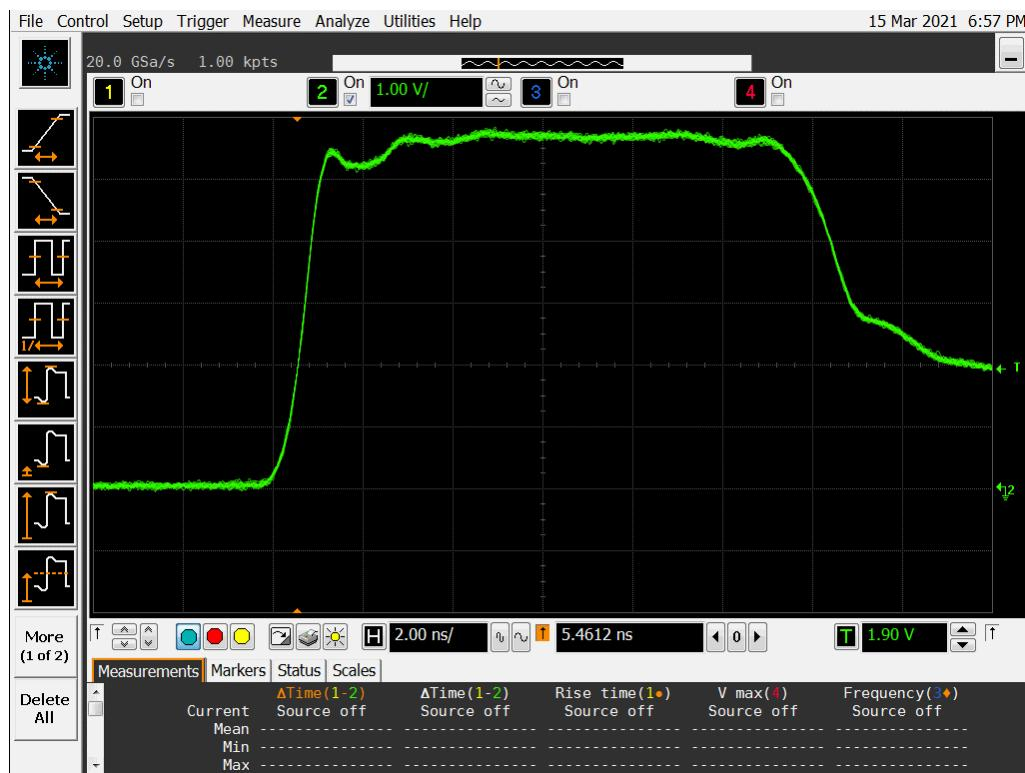
**Figure 11a DUT 453 Pre-Radiation Rising Edge**
