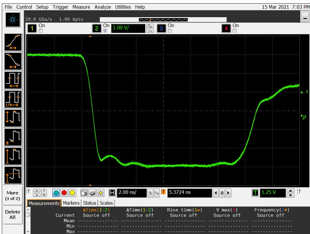
Figure 16a DUT 507 Pre-Irradiation Falling Edge
