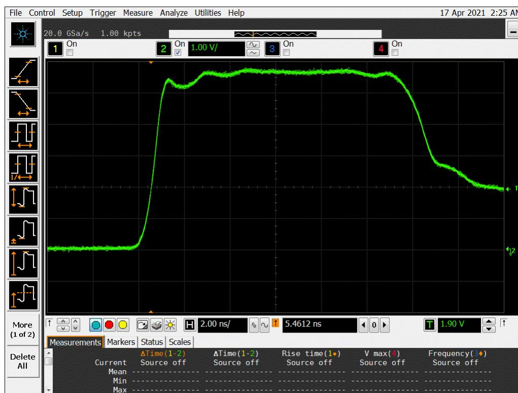
**Figure 13b DUT 394 Post-Annealing Rising Edge**
