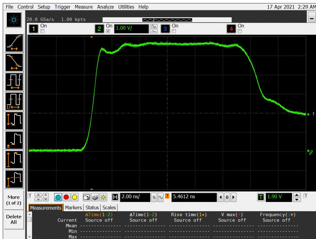
**Figure 11b DUT 453 Post-Annealing Rising edge**
