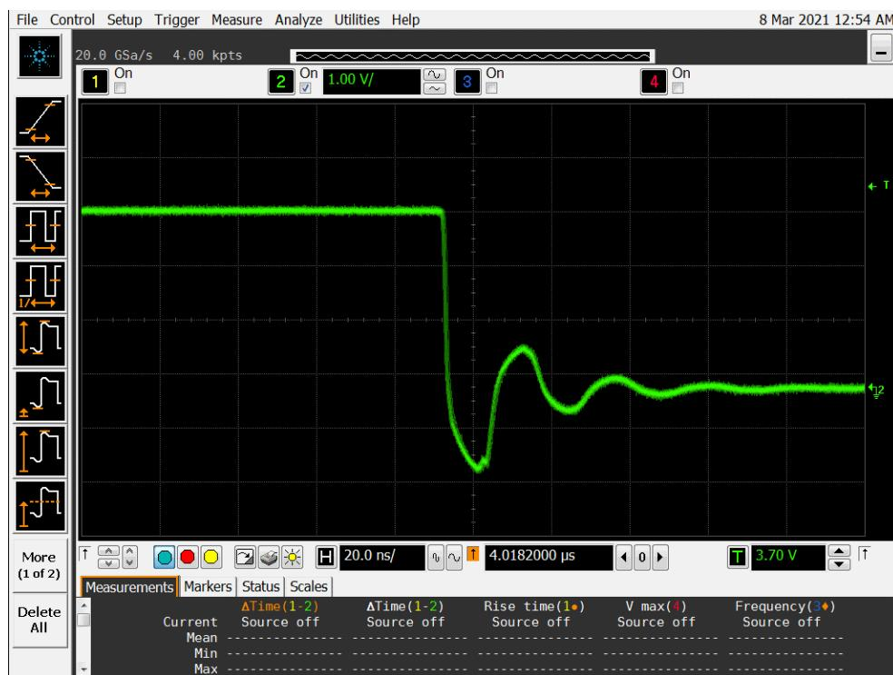
**Figure 11a DUT 16206 Pre-Irradiation Falling Edge**
