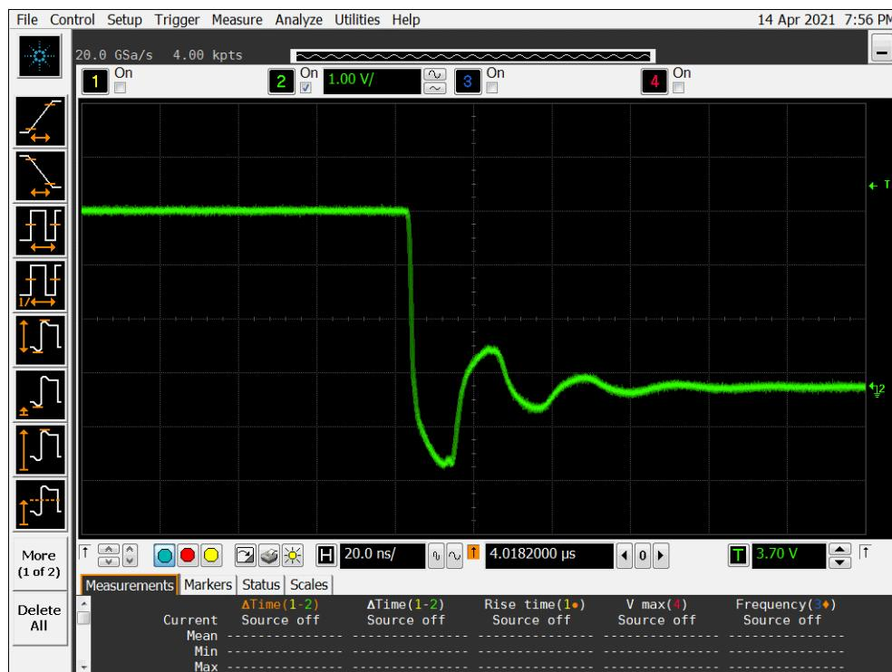
**Figure 9b DUT 16177 Post-Annealing Falling Edge**
