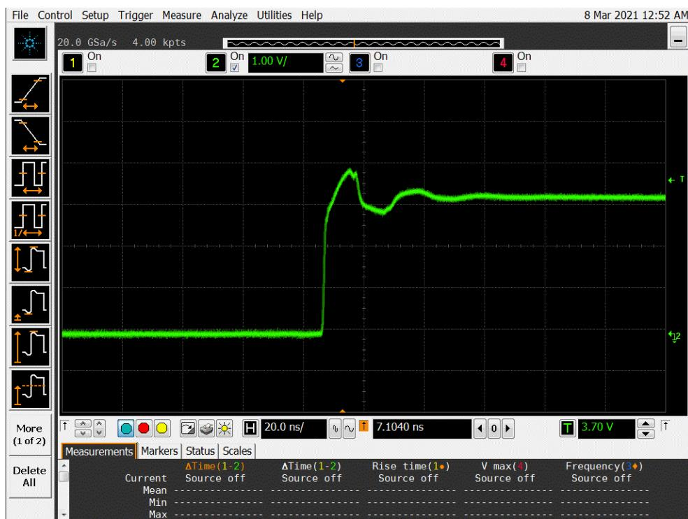
**Figure 4a DUT 16178 Pre-Irradiation Rising Edge**
