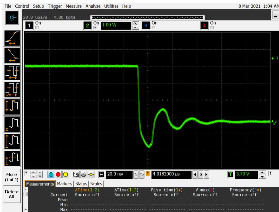
Figure 14a DUT 16224 Pre-Irradiation Falling Edge
