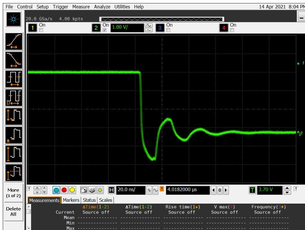
**Figure 11b DUT 16206 Post-Annealing Falling Edge**
