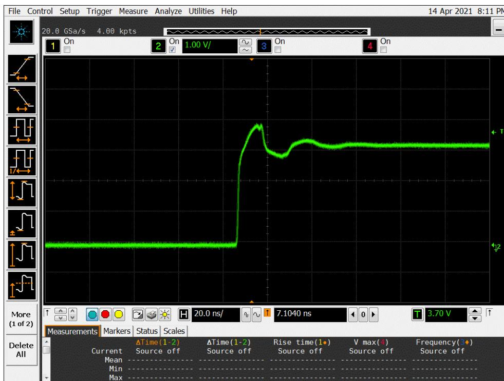
Figure 8b DUT 16224 Post-Annealing Rising Edge
