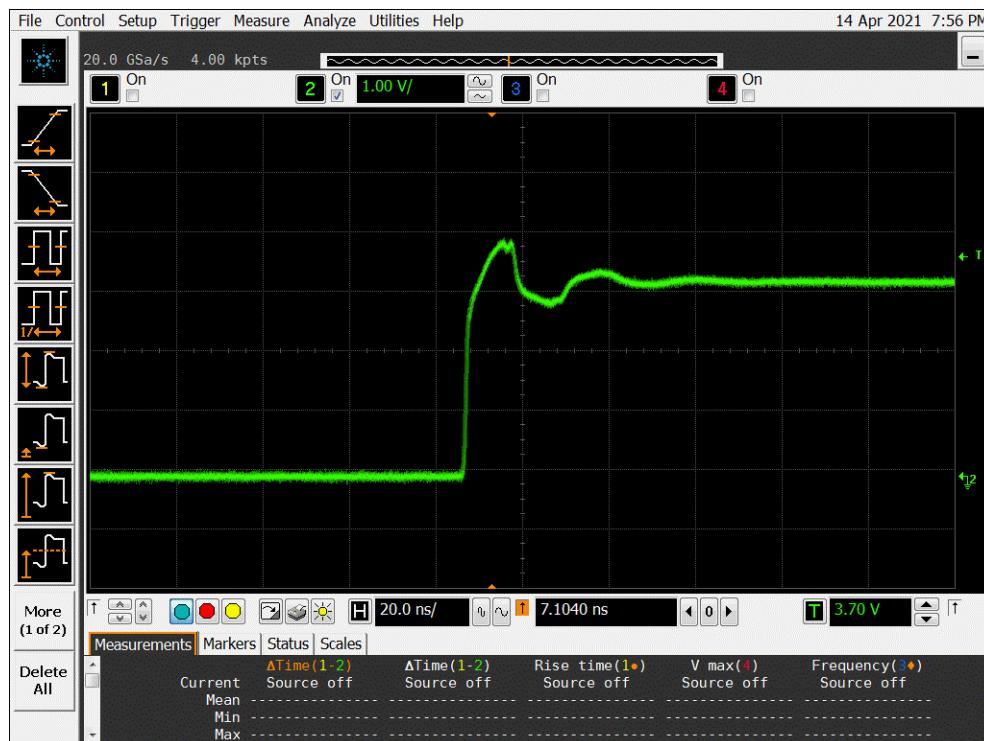
Figure 3b DUT 16177 Post-Annealing Rising Edge
