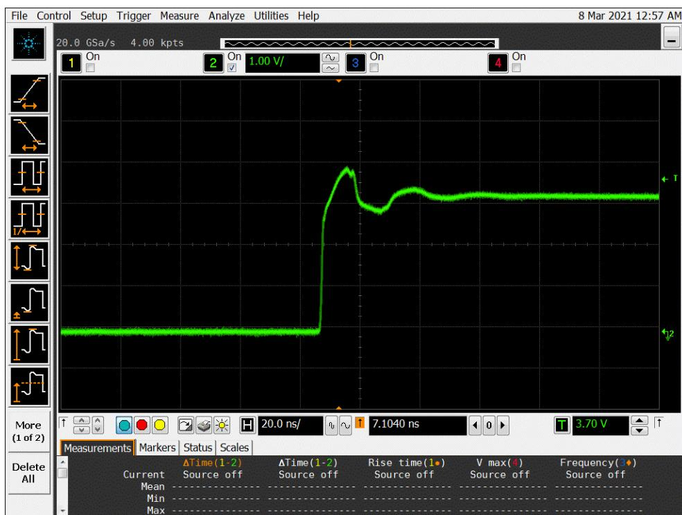
Figure 6a DUT 16207 Pre-Irradiation Rising Edge
