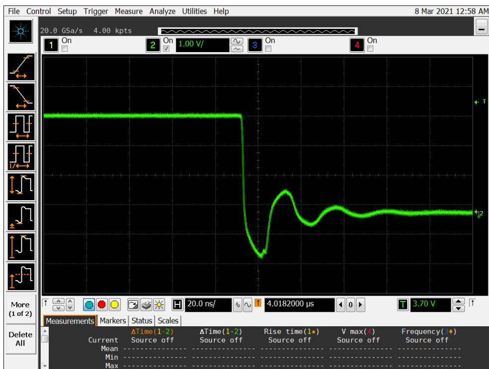
**Figure 12a DUT 16207 Pre-Irradiation Falling Edge**
