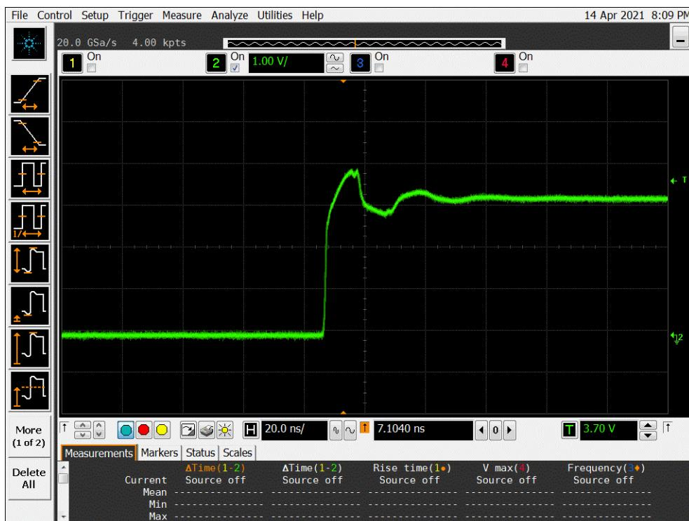
Figure 7b DUT 16208 Post-Annealing Rising Edge
