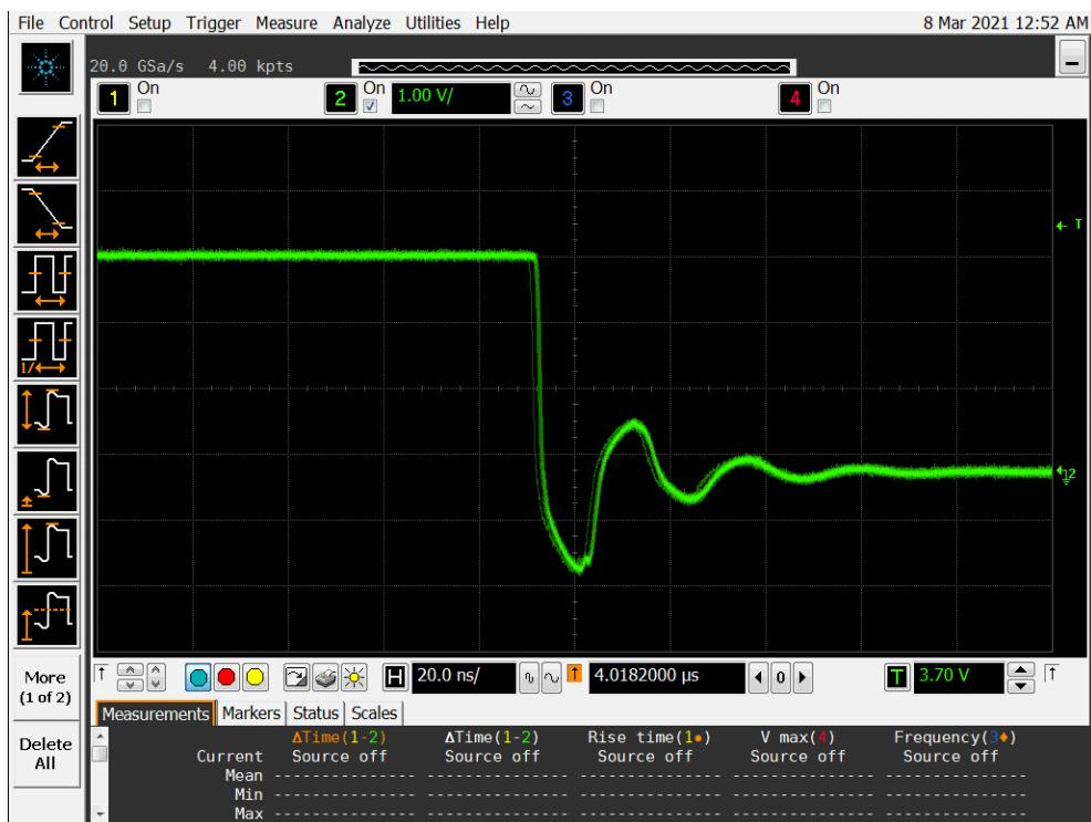
**Figure 10a DUT 16178 Pre-Irradiation Falling Edge**
