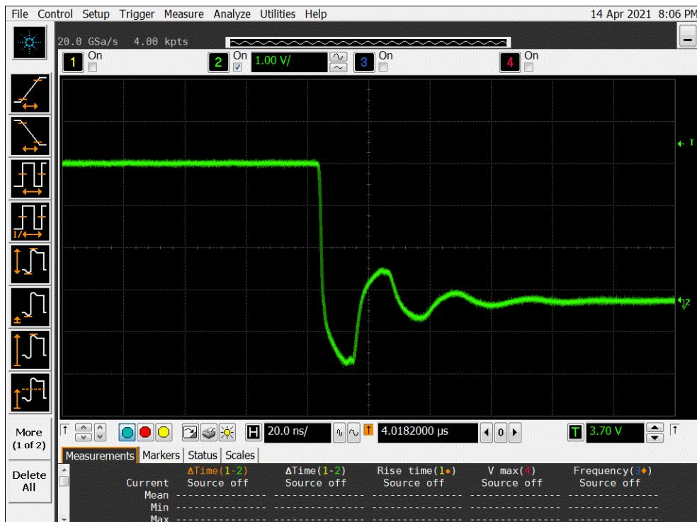
**Figure 12b DUT 16207 Post-Annealing Falling Edge**
