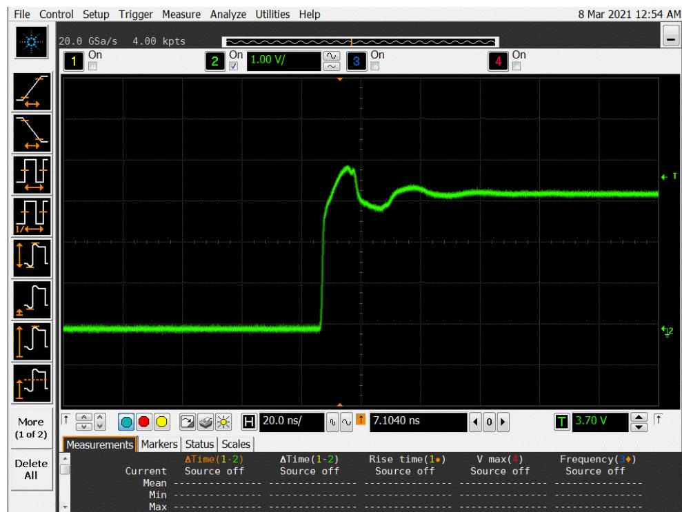
**Figure 5a DUT 16206 Pre-Irradiation Rising Edge**
