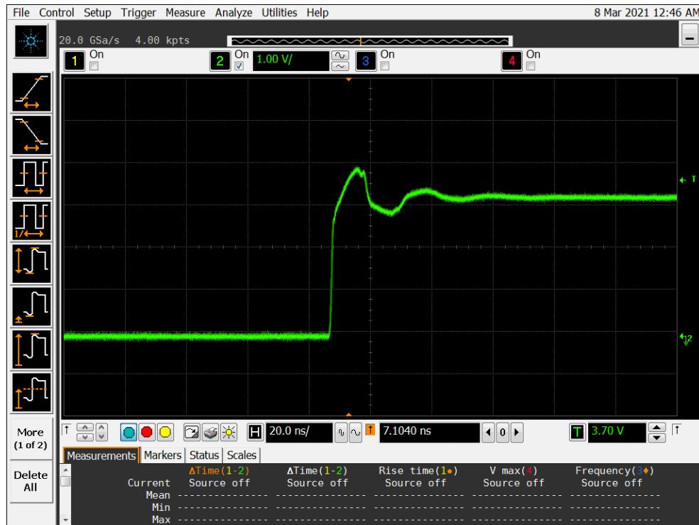
Figure 3a DUT 16177 Pre-Irradiation Rising Edge
