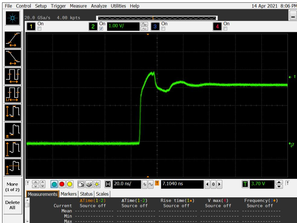
Figure 6b DUT 16207 Post-Annealing Rising Edge
